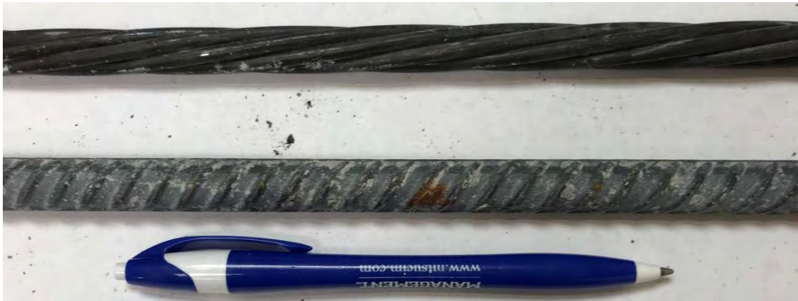
#6-10 (2.0% cast-in NaCl, high-chloride aggregate)
