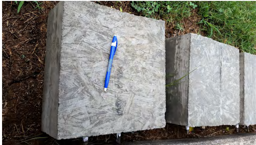
Figure 3.4 Examples of field-exposed concrete specimens
