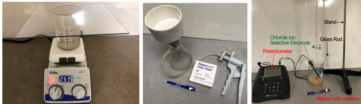
(a) Hot plate to boil sample (b) Filtration system (c) Titration system
