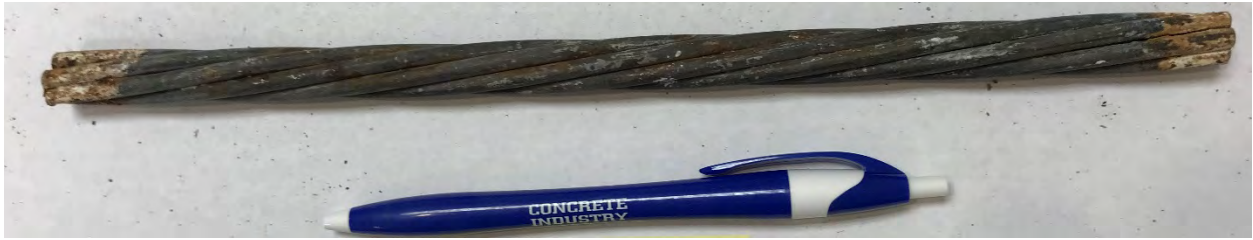
#12-8 (3.0% cast-in NaCl) Unstressed strand
