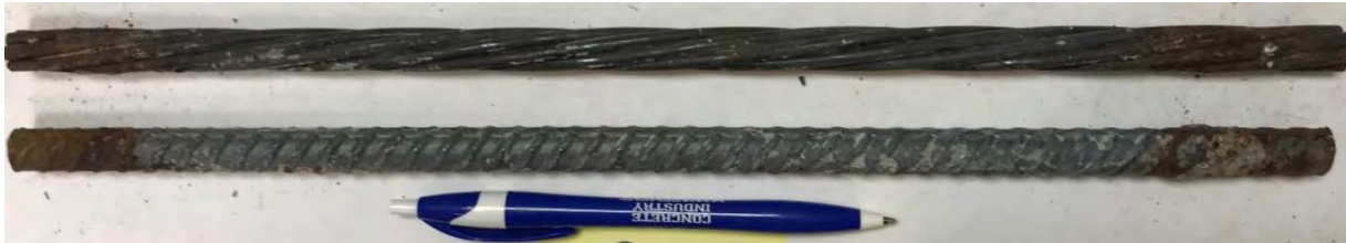
#5-10 (2.0% cast-in NaCl, high-chloride aggregate)
