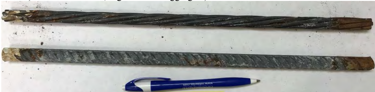
#6-10 (2.0% cast-in NaCl, high-chloride aggregate)
