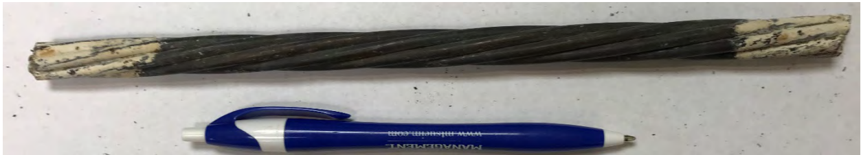
#12-6 (2.0% cast-in NaCl) Unstressed strand
