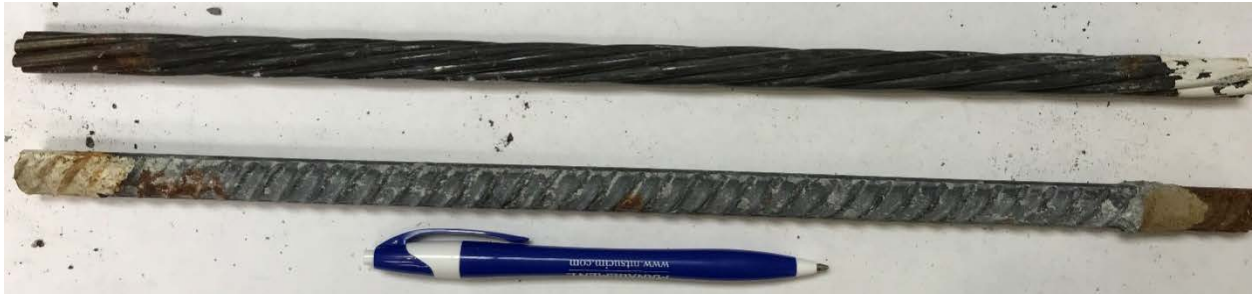
#6-9 (0.3% cast-in NaCl, high-chloride aggregate)
