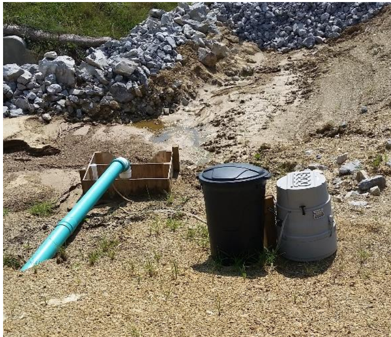
Figure 2.10. Alternate view of outlet monitoring device at Knox County, includes ISCO® 3700 Portable Sampler, tubing, and bubbler housing.
