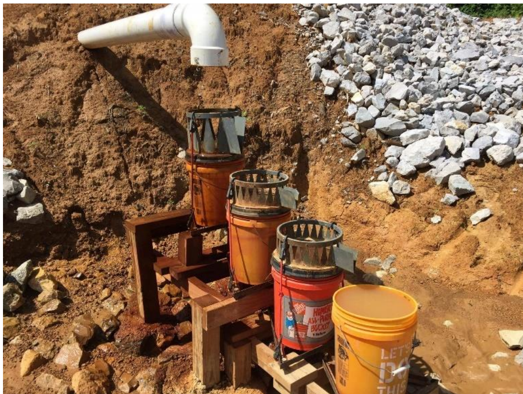
Figure 2.7. Morgan County sediment basin outlet monitoring buckets, stand, and leveling device.
