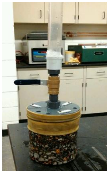
Figure 4-6 Permeability test setup
