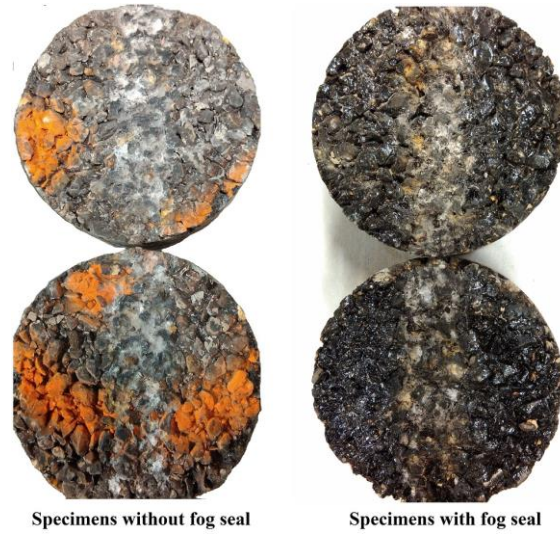
Figure 4-12 Cores after loaded wheel abrasion test
