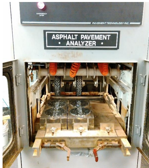
Figure 4-9 LWT abrasion test
