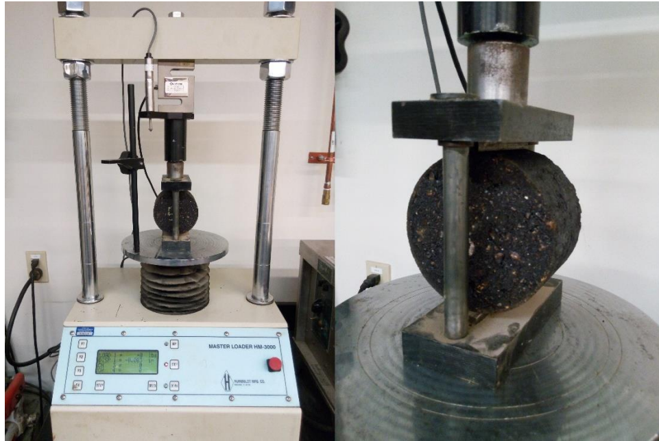
Figure 6-1 Testing tensile strength under diametral load
