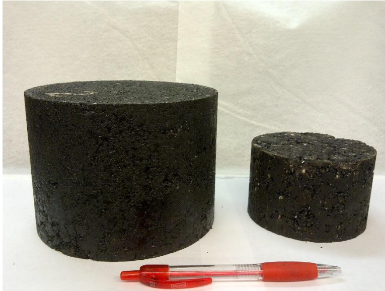
Figure 2-2. Superpave specimen on the left and Marshall specimen on the right.
