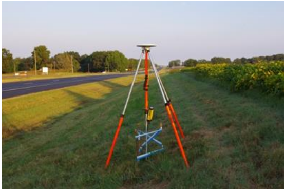
(a) GPS base station
