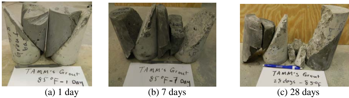
Figure B36 - Failure patterns of slant shear bond test for TAMM's Grout Supreme at different ages at medium temperature (85°F) (Mix #19)
