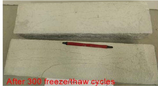
Figure D7- Visual appearance of specimens before and after freeze and thaw test for CTS Rapid Set CEMENT ALL Grout (Mix #7)
