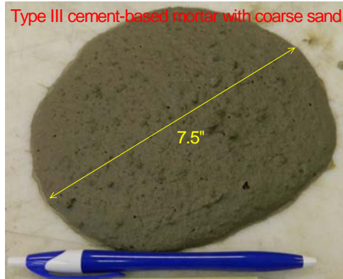
Figure E6-Spread of mini slump test for type III cement-based normal mortar with natural river sand (#45)
