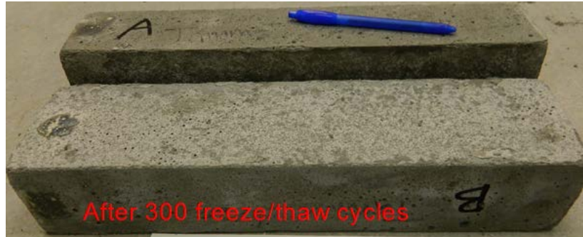
Figure D9- Visual appearance of specimens after freeze and thaw test for Euclid TAMMs GROUT SUPREME (Mix #19)
