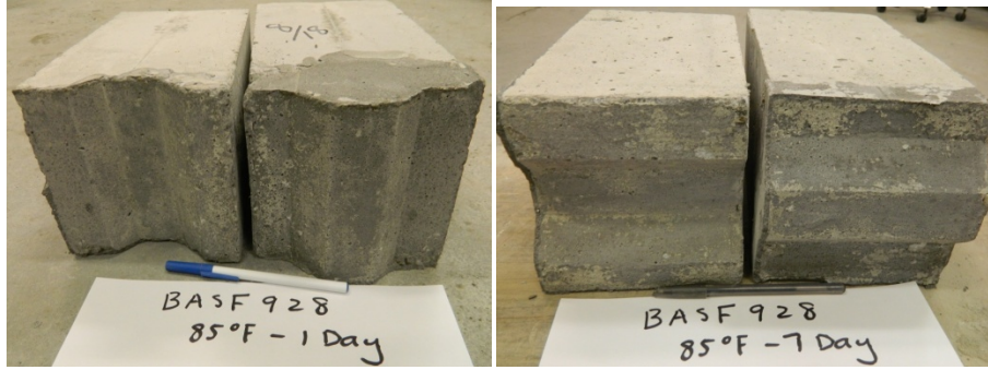
Figure A26 - Failure patterns of flexural bond test for BASF 928 Grout at different ages at medium temperature (85°F) (Mix #1)
