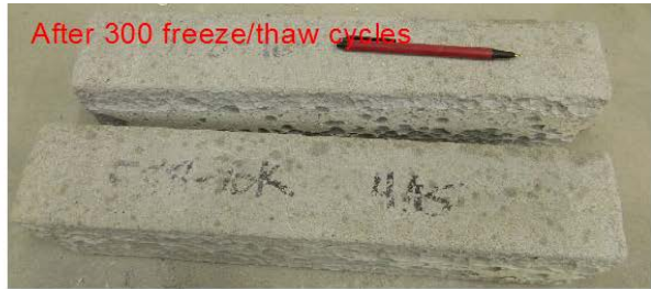
Figure D6- Visual appearance of specimens before and after freeze and thaw test for W.R Meadow SEALTIGHT 588-10K (Mix #6)
