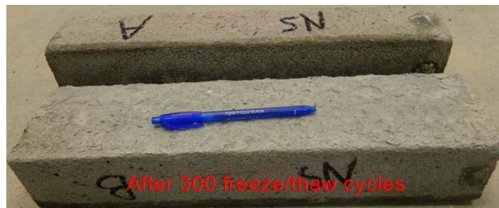
Figure D12- Visual appearance of specimens after freeze and thaw test for Euclid NS Grout (Mix #22)
