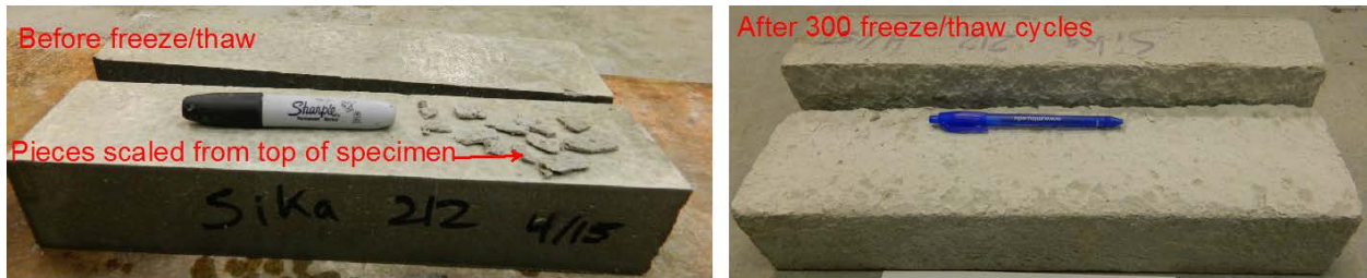
Figure D3- Visual appearance of specimens before and after freeze and thaw test for SikaGrout 212 (Mix #3)
