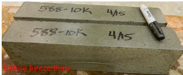
Figure D6- Visual appearance of specimens before and after freeze and thaw test for W.R Meadow SEALTIGHT 588-10K (Mix #6)
