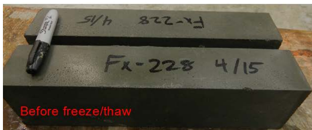
Figure D8- Visual appearance of specimens before and after freeze and thaw test for Simpson StrongTie FX-228 (Mix #9)
