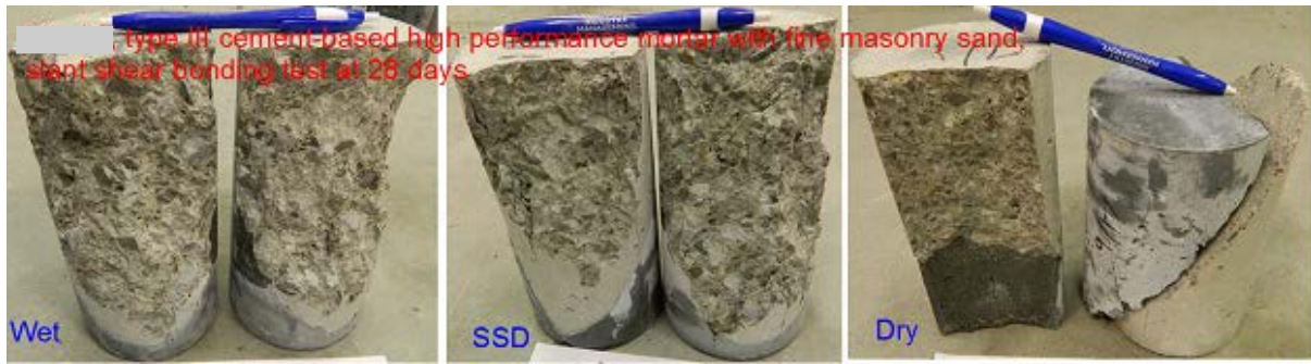
Figure G6-Failure mode of slant shear bond test at 28 days for type III cement-based high performance mortar using fine masonry sand and different substrate surface moisture conditions (#50)
