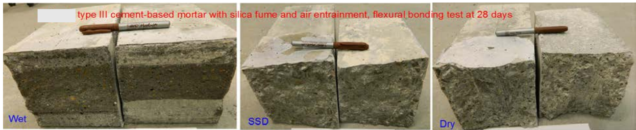
Figure F3-Failure mode of flexural bond test at 28 days for type III cement-based mortar using natural river sand, AEA, and different substrate surface moisture conditions (#47)
