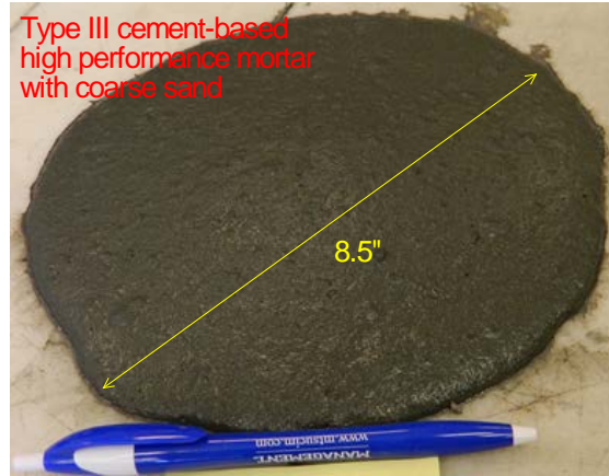
Figure E9-Spread of mini slump test for type III cement-based high performance mortar with natural river sand (#48)
