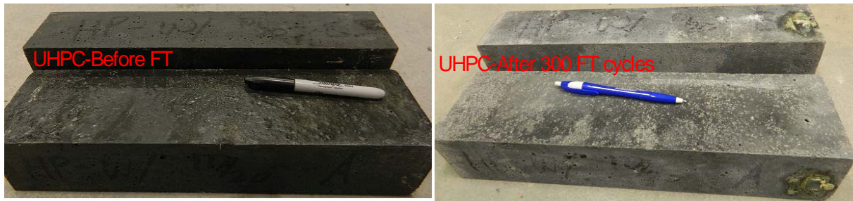
Figure H5-Visual appearance of freeze and thaw test specimens for type III cement-based UHPC (#51)
