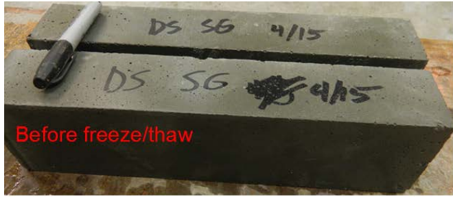
Figure D5 - Visual appearance of specimens before and after freeze and thaw test for Dayton Superior Sure-Grip High Performance Grout (Mix #5)
