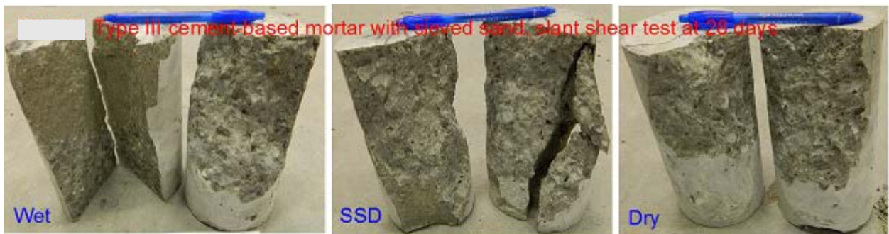
Figure G2-Failure mode of slant shear bond test at 28 days for type III cement-based mortar using sieved river sand and different substrate surface moisture conditions (#46)
