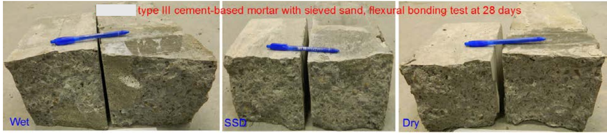
Figure F2-Failure mode of flexural bond test at 28 days for type III cement-based mortar using sieved river sand and different substrate surface moisture conditions (#46)
