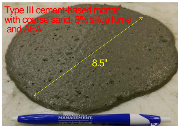
Figure E8-Spread of mini slump test for type III cement-based normal mortar with natural river sand, silica fume, and AEA (#47)
