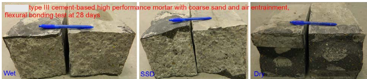
Figure F5-Failure mode of flexural bond test at 28 days for type III cement-based high performance mortar using natural river sand, AEA, and different substrate surface moisture conditions (#49)
