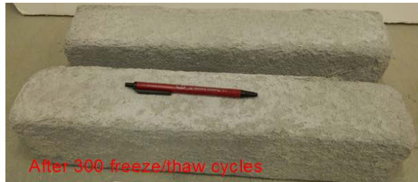
Figure D8- Visual appearance of specimens before and after freeze and thaw test for Simpson StrongTie FX-228 (Mix #9)
