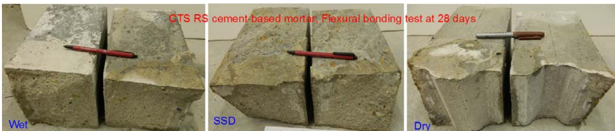
Figure F9-Failure mode of flexural bond test at 28 days for CTS rapid set cement-based mortar with different substrate surface moisture conditions (#54)
