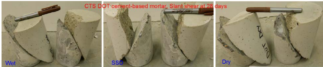
Figure G10-Failure mode of slant shear bond test at 28 days for CTS DOT cement-based mortar with different substrate surface moisture conditions (#55)
