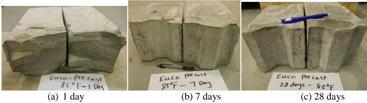
Figure A37 - Failure patterns of flexural bond test for Euclid Euco-PreCast Grout at different ages at medium temperature (85°F) (Mix #20)
