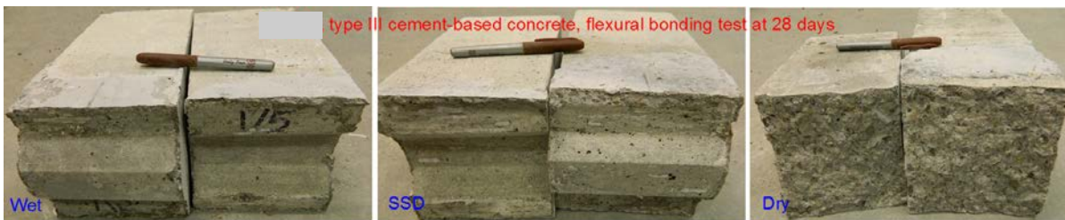
Figure F8-Failure mode of flexural bond test at 28 days for type III cement-based concrete with different substrate surface moisture conditions (#52)
