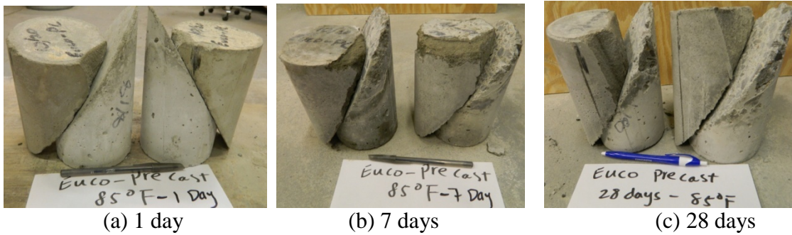
Figure B37 - Failure patterns of slant shear bond test for Euclid Euco Pre-cast Grout at different ages at medium temperature (85°F) (Mix #20)
