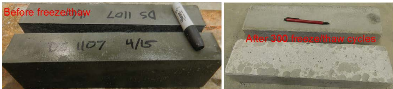
Figure D4- Visual appearance of specimens before and after freeze and thaw test for Dayton Superior 1107 Advantage Grout (Mix #4)
