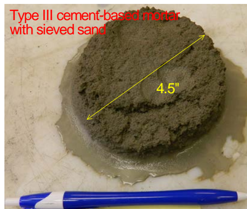
Figure E7-Spread of mini slump test for type III cement-based mortar with sieved river sand (#46) (note: water separation possibly due to insufficient paste)
