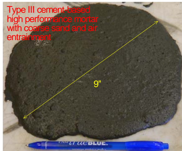
Figure E10 -Spread of mini slump test for type III cement-based high performance mortar with natural river sand, AEA, and SRA (#49)
