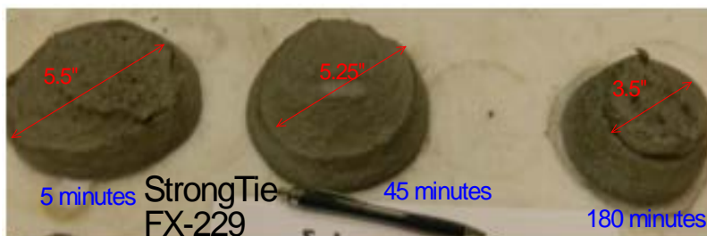
Figure C43 - Spread of mini slump test for Simpson StrongTie FX-229 Grout at different time at high temperature (95°F) (Mix #10)
