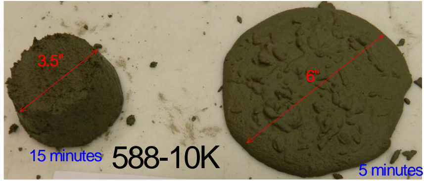
Figure C40 - Spread of mini slump test for W.R Meadows 588-10K Grout at different time at high temperature (95°F) (Mix #6)
