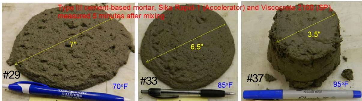
Figure E4-Spread of mini slump test for type III cement-based mortars (#29, #33, and #37) using Sika Rapid-1 (accelerator) and Viscocrete 2100 (superplsticizer) at different temperatures
