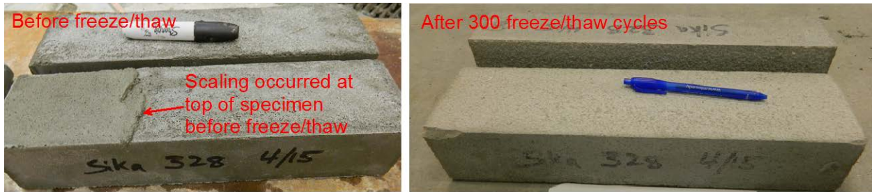
Figure D2- Visual appearance of specimens before and after freeze and thaw test for SikaGrout 328 (Mix #2)
