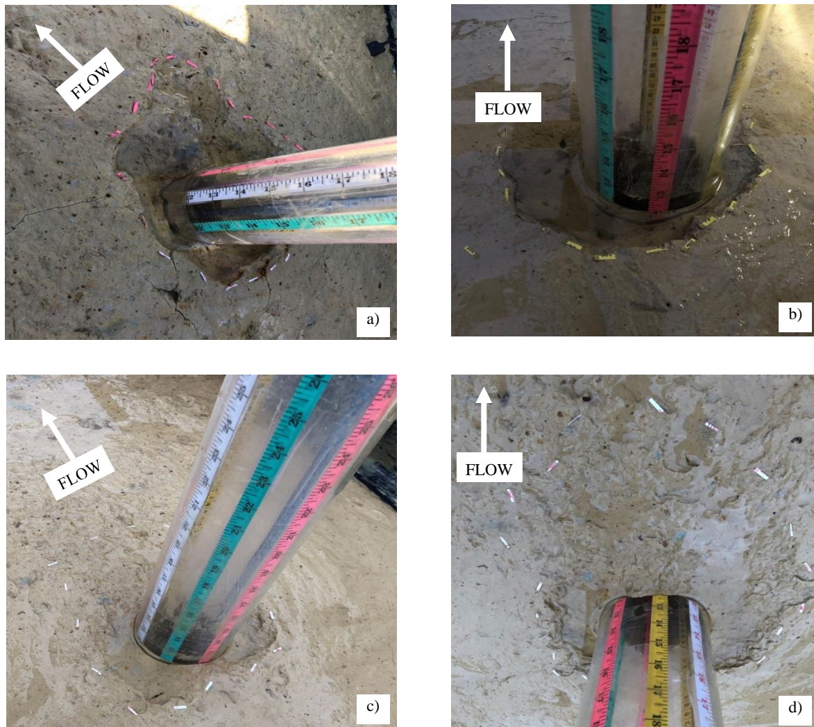
Figure 4.4. Scour hole development for: a) run 16, V = 80.68 cm/s, WC = 37.45\% , b) run 14, V = 80.10 cm/s, WC = 38.12\% , c) run 10, V = 90.26 cm/s, WC = 31.25\% , and d) run 9, V = 102.40 cm/s, WC = 31.25\% .
