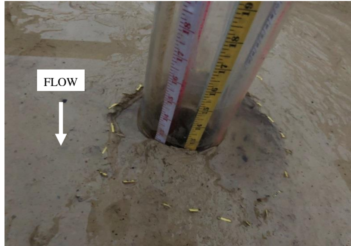
Figure 4.5. Scour hole development and the soil removal erosion pattern at the wake zone of the pier: run 14, V = 80.10 cm/s, WC = 38.12\% .
