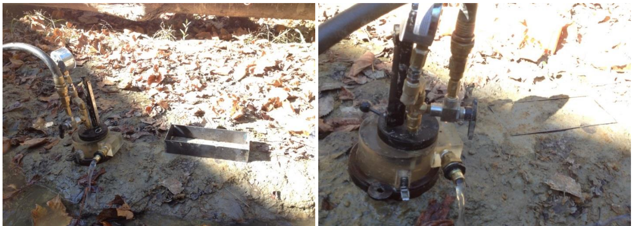
Fig. 4. In-situ mini-jet testing and sample collection at the Black Creek site.
