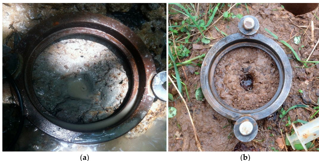
Figure 11. Photos of scour hole formation in different soil physical conditions (a) wide and shallower, and (b) narrow and deeper.
