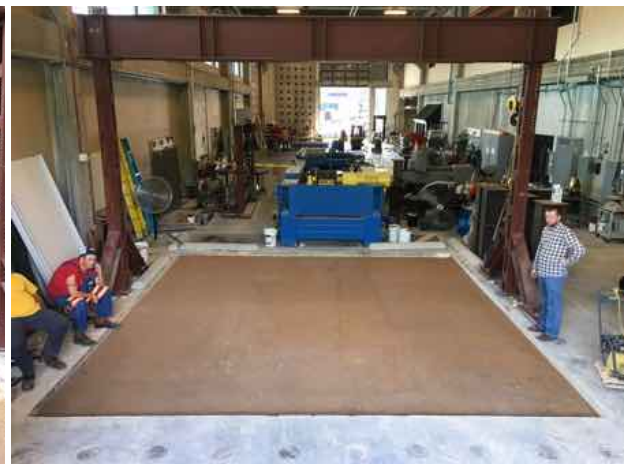
(b) Aggregate Base Compaction
