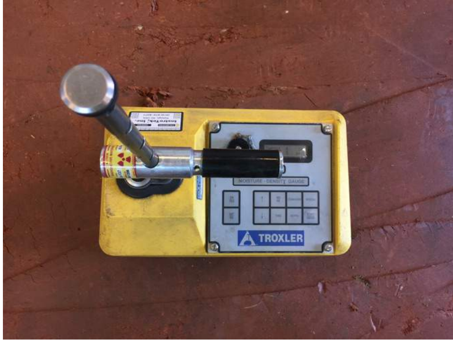
Figure 5.6: Checking Subgrade Density with a Nuclear Gauge
