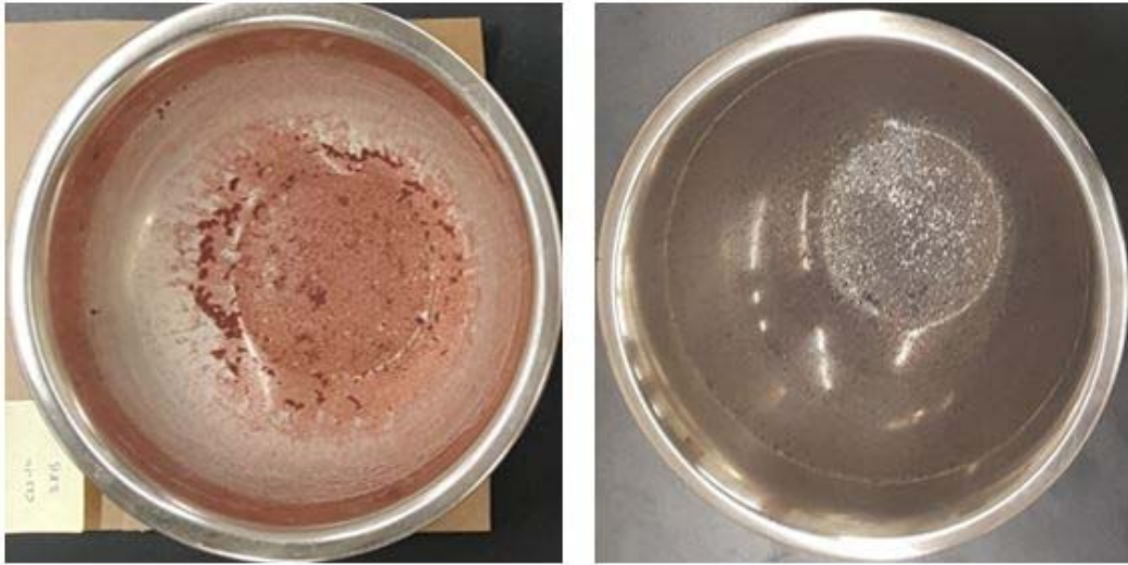
Figure 10. Photograph of WTA residue for CSS-1h (left) and LD-7 (right) specimens.
