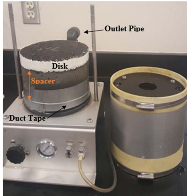
Figure 16. Photograph of Gilson permeameter with disk specimen spacer.
