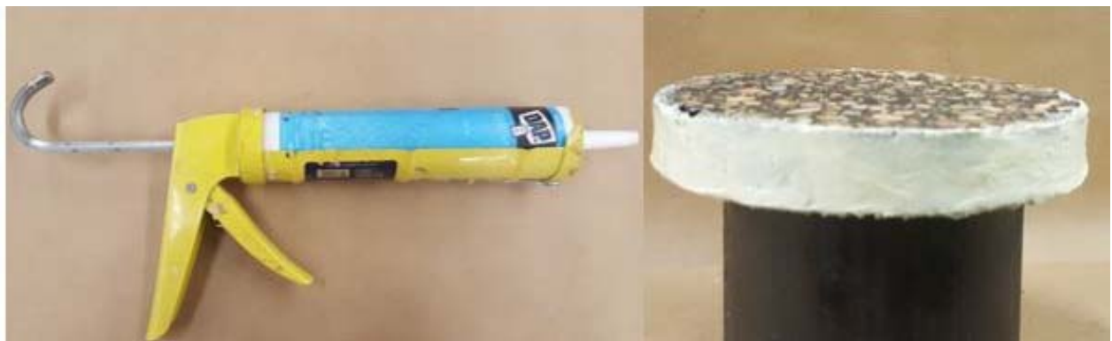
Figure 18. Silicone caulk (left) and silicone applied at the disk edges (right).
