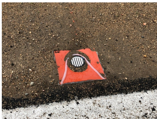
Figure 3.3 Photograph showing debris collected on runoff sampler surface that caused sampling issues (Photo courtesy: Mark Daly, Fairbault County).
