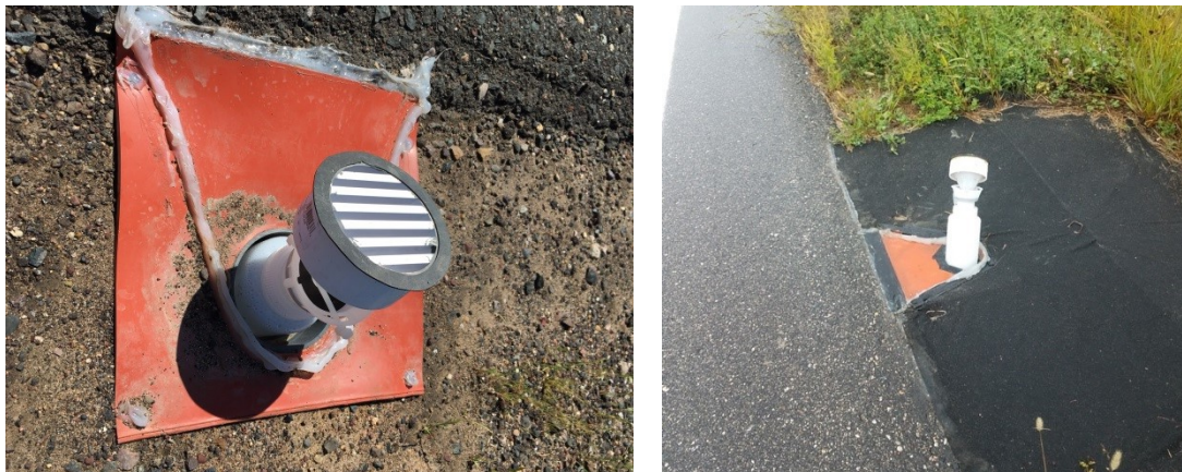
Figure 3.5 Photographs showing the sample bottle displaced from the runoff sampler after a rainfall event (photos taken at a Chisago County site by Poornima Natarajan (left) and at the Clearwater county site by Dan Sauve (right)).
