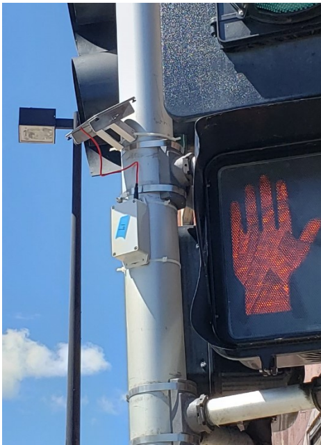
Figure 2.11 Images of Bluetooth Devices Attached to Signal Poles at Greeley & Hwy 36.
