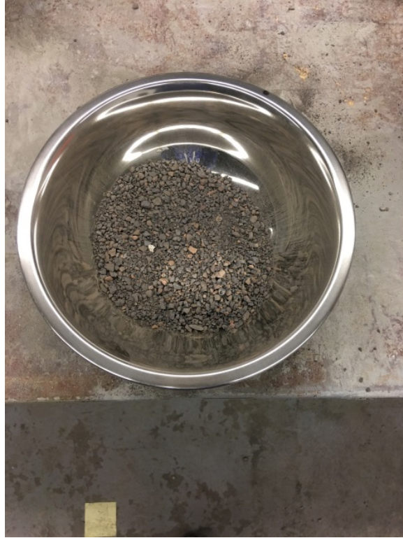
Figure 7. Photo. Total moisture sample.
