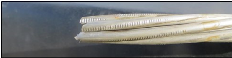
Figure 17. Fracture at Wedge Tip Location With Strand Breaking Before Completing Fabrication of First Set of Stainless Reinforced Concrete Piles
