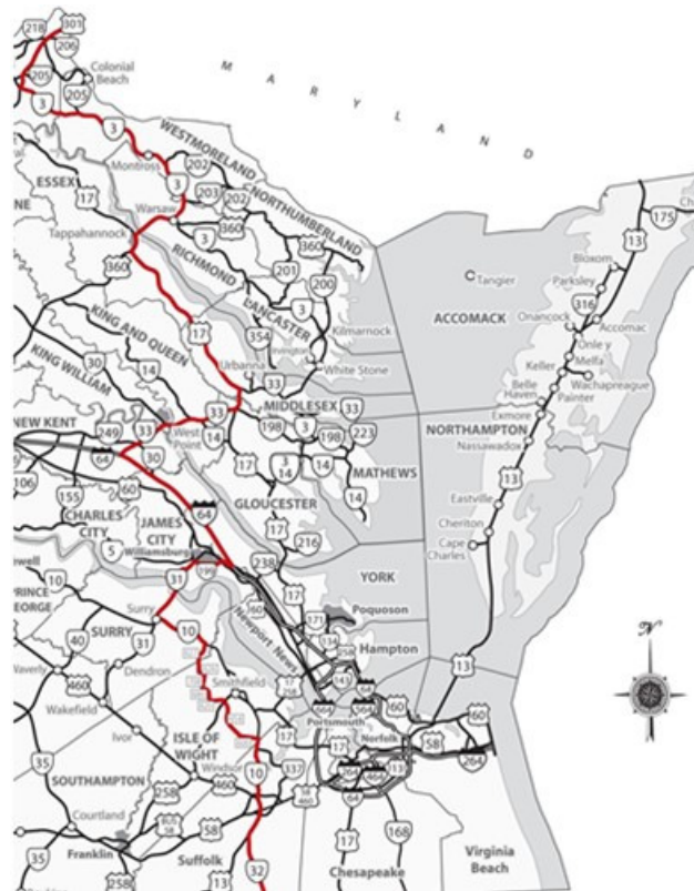
Figure 21. Region Requiring Use of CFRP or SCW2205 Steel Strands in Piles. Region to the east (right) of the red line requires CFRP or SCW2205 steel reinforcement (VDOT, 2018). CFRP = carbon fiber reinforced polymer
