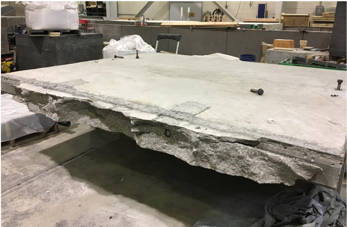
Figure 4.17: Grout Shear Key Bond Failure (Specimen F-M)
