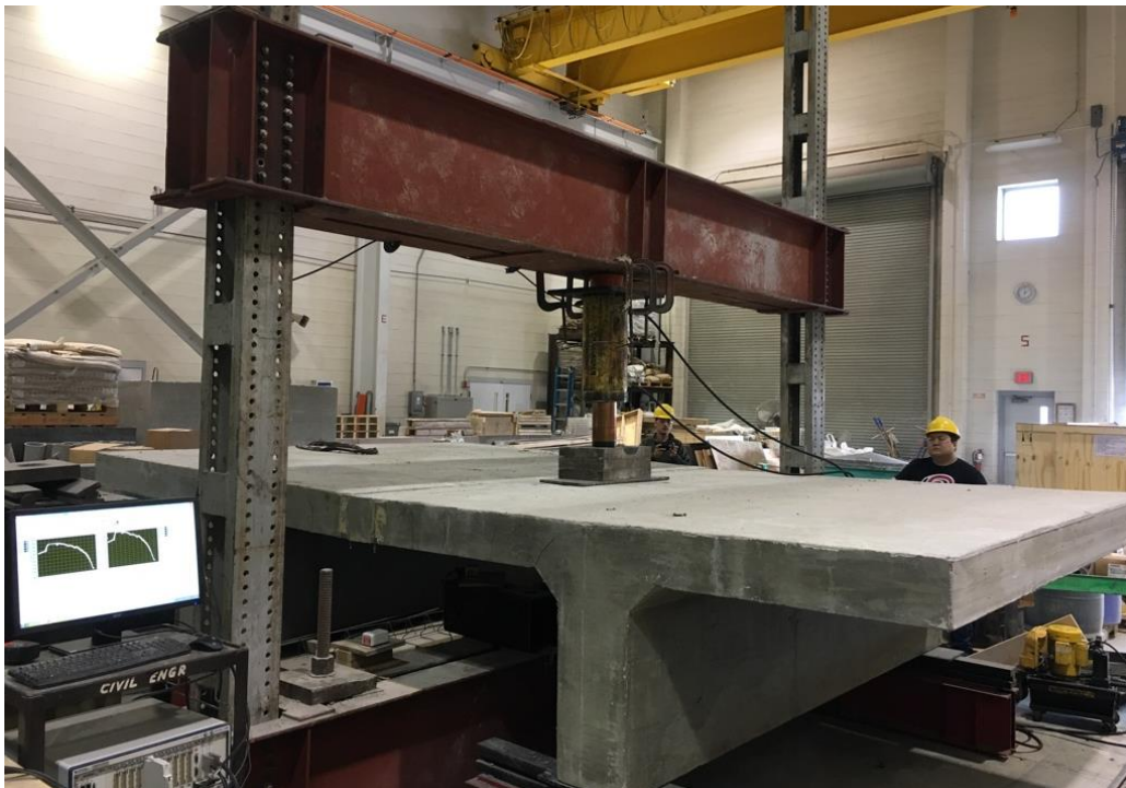
Figure 4.21. Test Setup and Loading of Specimen F-R-SHPC
