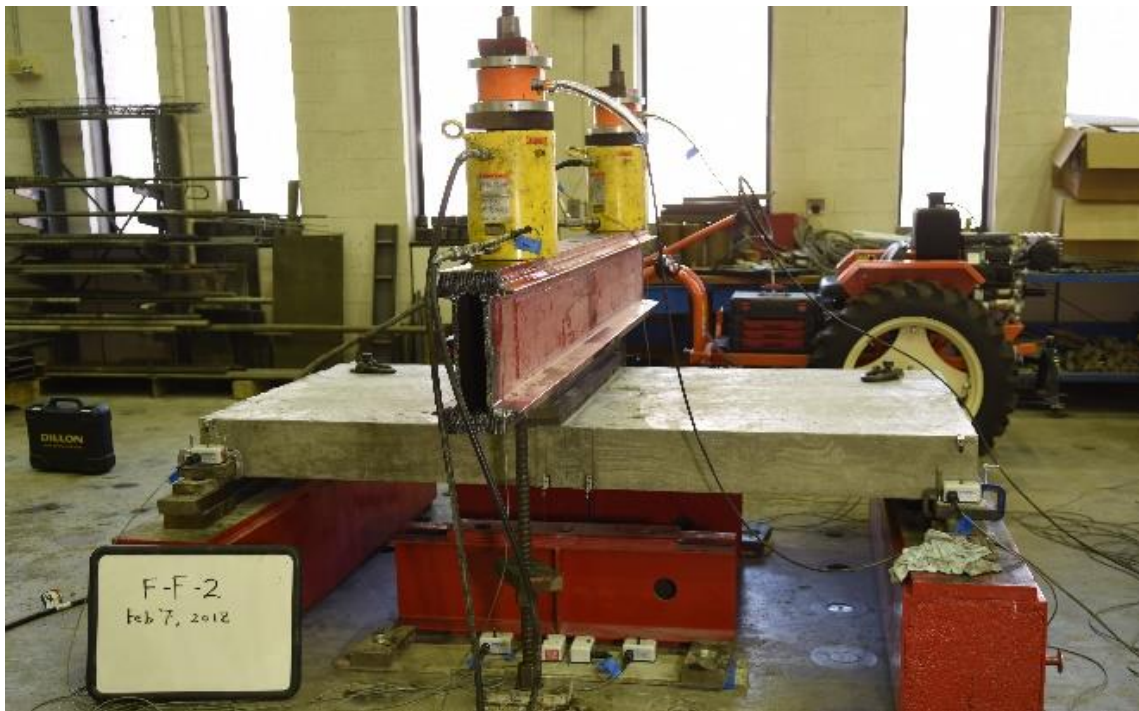
Figure 3.35: Three-point Bending Test Setup (Specimen F-F-2)
