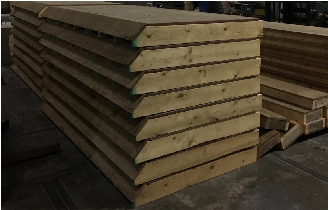
Figure 4.2: Formworks for Full-Scale Bridge Specimens
