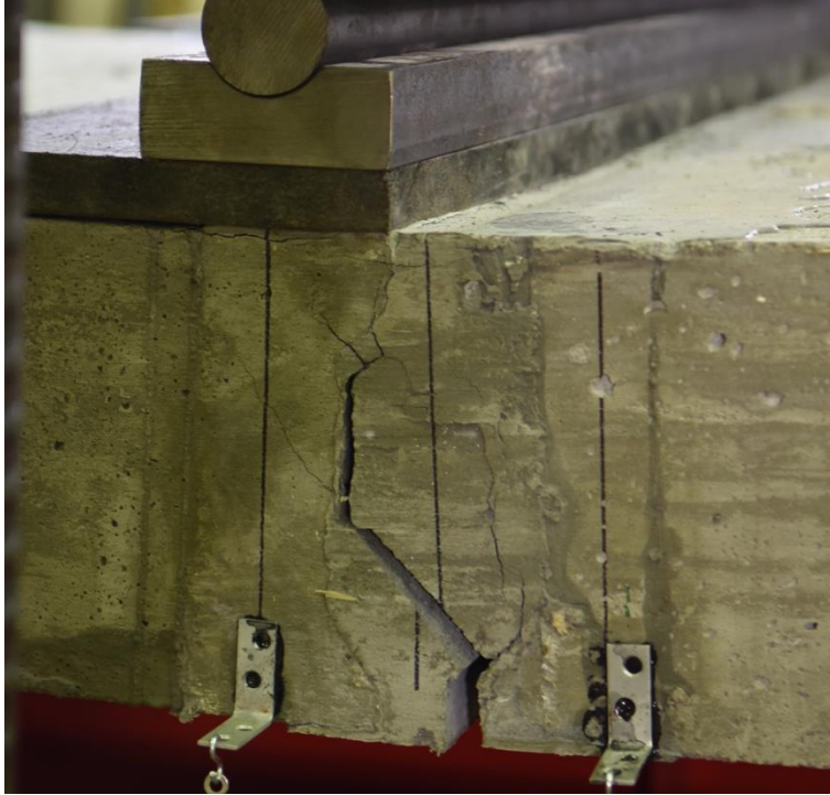
Figure 3.38: Grout Joint Close-up Photo (Specimen F-F-2, South view)
