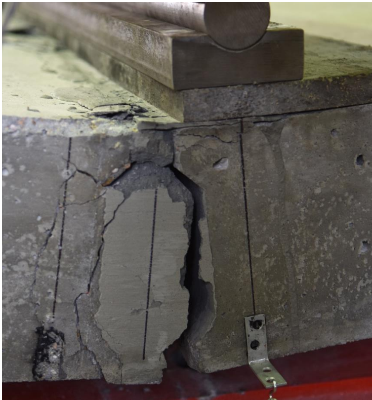
Figure 3.39: Shear Key before Failure (Specimen F-F-2, North view)
