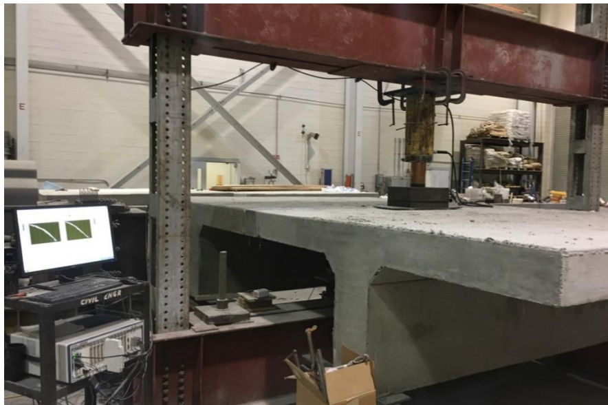
Figure 4.24. Test Setup and Loading of Specimen F-N-SHPC
