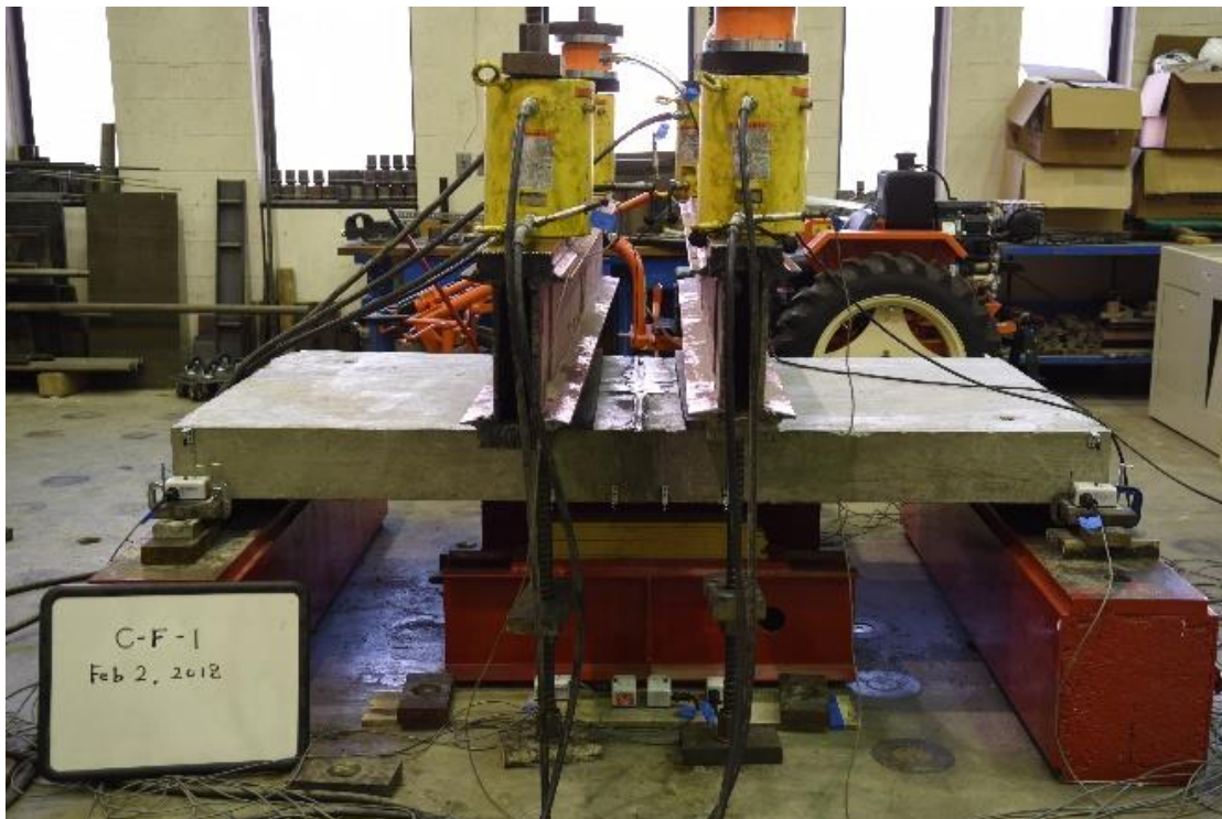
Figure 3.25: Four-point Bending Test Setup (Specimen C-F-1)
