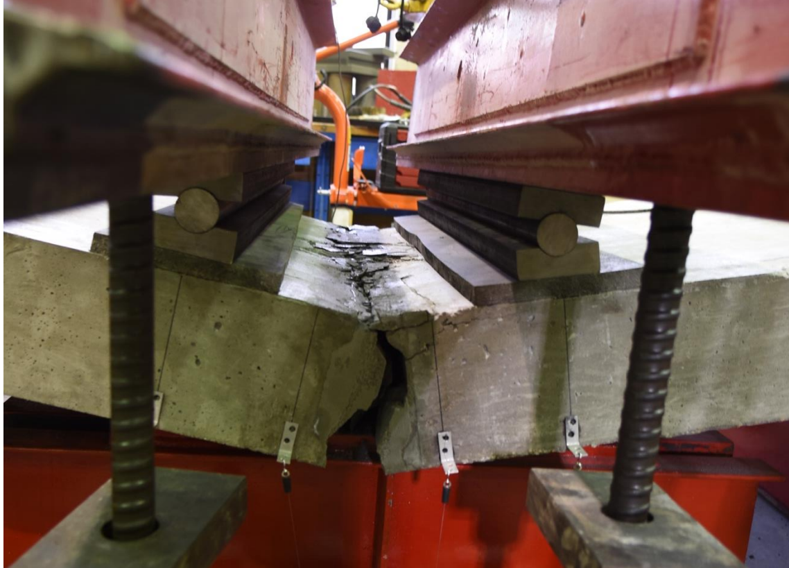
Figure 3.22: Specimen C-C-1 at Failure (view from North side)
