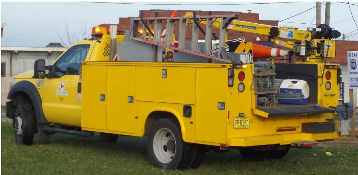
Figure 3.1 Sign Truck Equipped with Tools and Material for Sign Replacement
