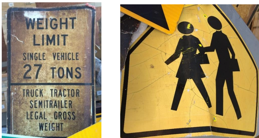
Figure 1.6 Example of damaged Signs: Dirty, Faded, Cracked, and Bent
