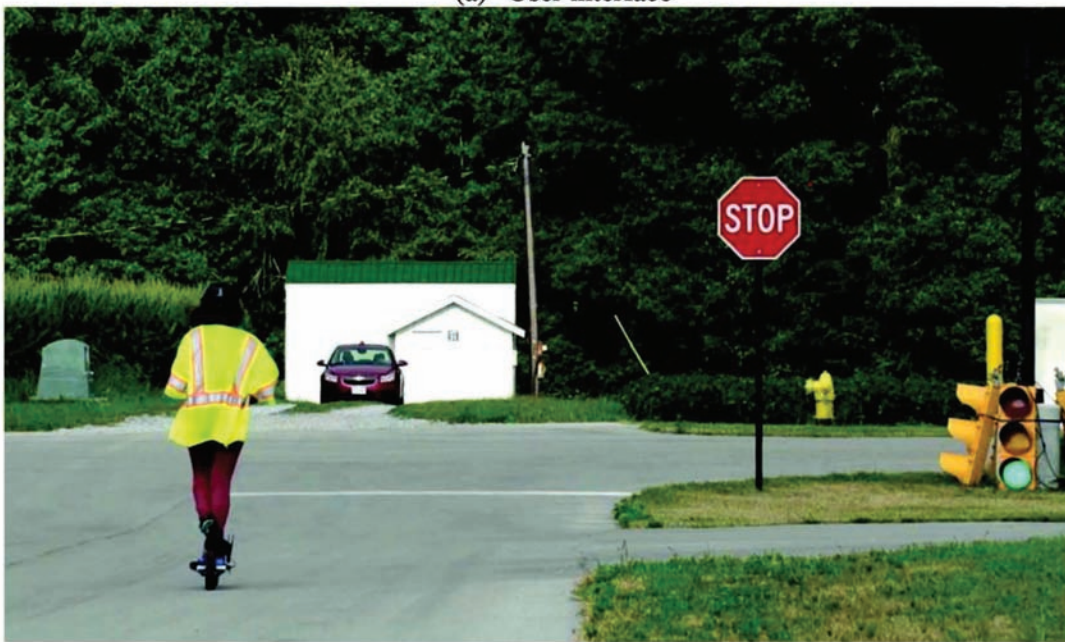
(b) An E-scooter placing virtual calls on the traffic signal controller
