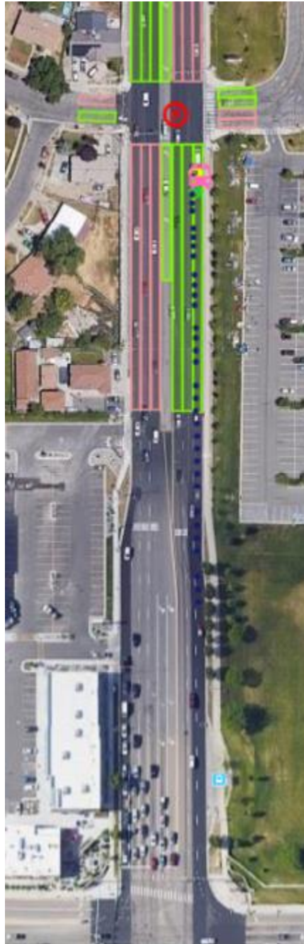
Figure 3-23: DSRC OBE UI map when 10-second refresh rate affects TSP operations.
