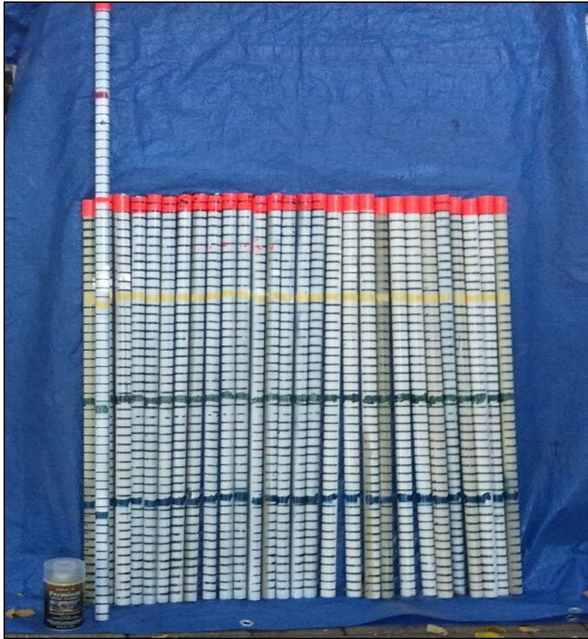
Figure 36. Photo. Sample painted measuring stakes.
