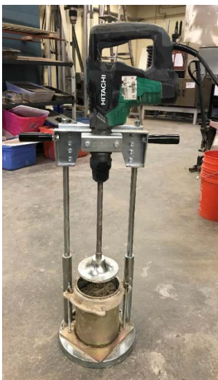
Figure 8-2: Impact Hammer Setup and Circular Steel Tamping Plate and Metal Shaft.
