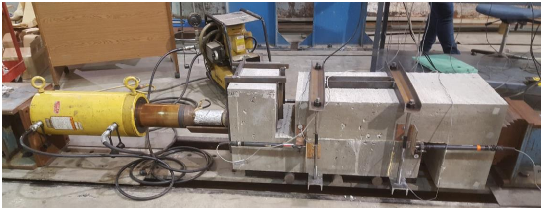
Figure 12. Horizontal Shear Push-off Specimen Testing Apparatus
