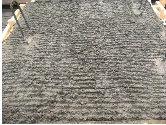
Figure 19. Raked Surface Finish above Extended Web Region
