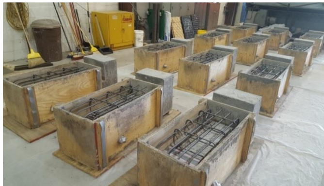
Figure 11. Forms and Reinforcing for Push-off Specimens for Top Section
