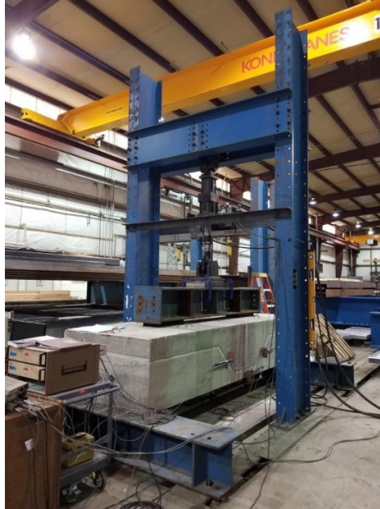
Figure 26. Test Set-up for Virginia Inverted T-Beam Bridge System Sub-assembly Specimen
