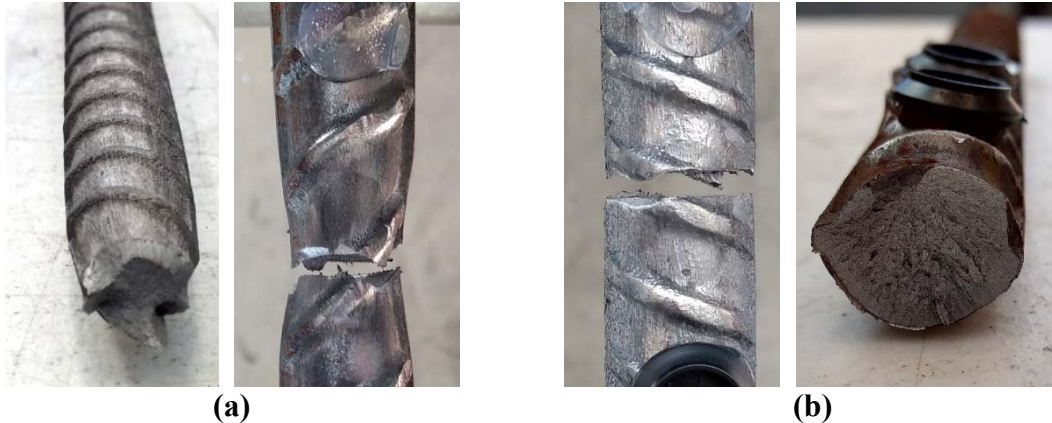
Figure 7-4. (a) “Ductile” rebar fracture; (b) “Brittle” rebar fracture
