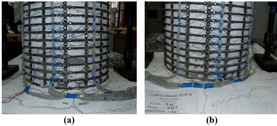
(a) (b) Figure 4-75. Onset of footing concrete “uplift”: (a) South, \mu_4^{1+} ; (b) North, \mu_3^{1-}
