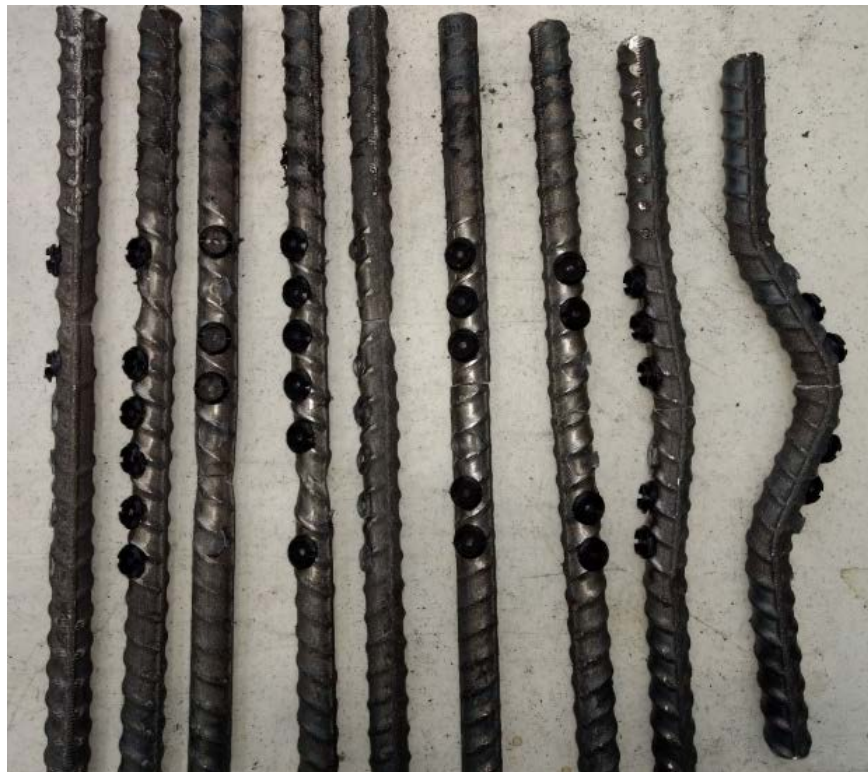
Figure 7-7. BBT test specimens after fracture
