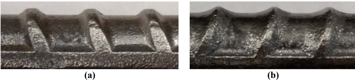
Figure 7-10. (a) Mill 1 bar profile; (b) Mill 2 bar profile
