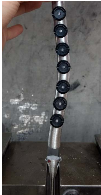
Figure 7-17. Brittle failure of turned down bar in undesired location
