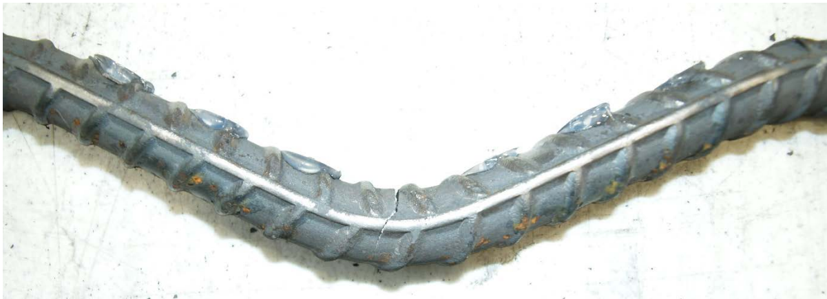
Figure 7-6. Onset of bar fracture after buckled bar tension test
