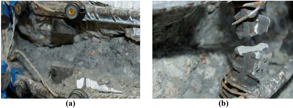
Figure 4-5. (a) Flat bar fracture surface (S4); (b) Uneven bar fracture surface (N4)
