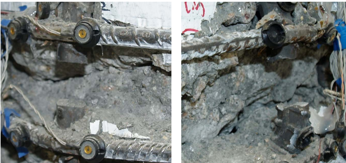
Figure 7-5. Column test bar fracture surfaces
