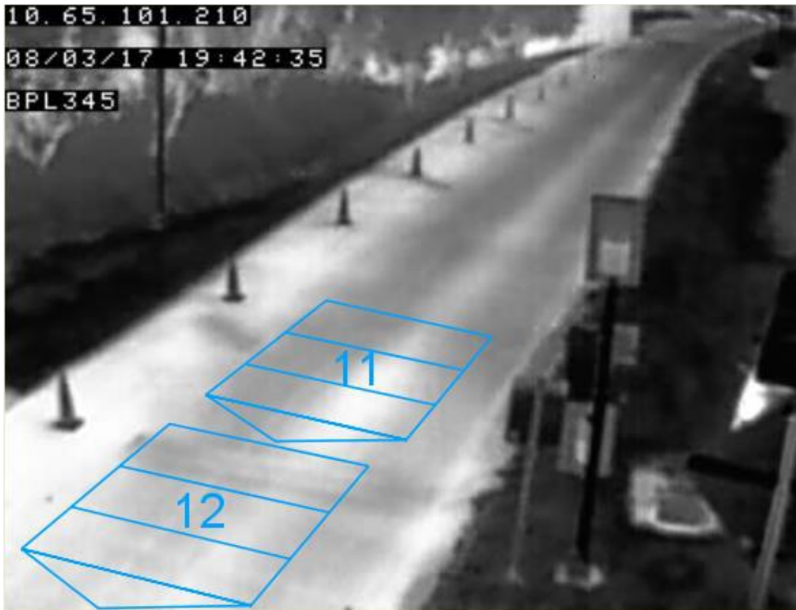
Figure 4-12. FLIR Video Camera Detection Zones for Vehicle Counts and Occupancies
