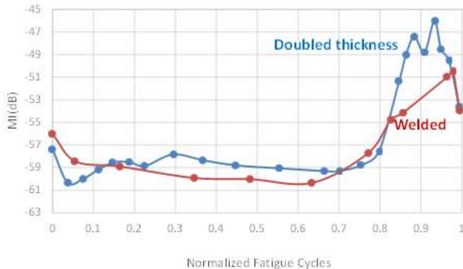
Figure 39. Modulation Index vs number of fatigue cycles ratio for doubled thickness and welding
