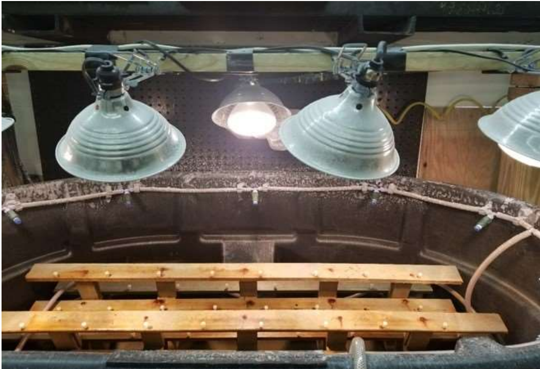
Figure 35. Corrosion equipment using UV at Rutgers University
