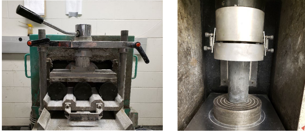
Figure 3.9 Cylinder end grinding and compressive strength test setup
