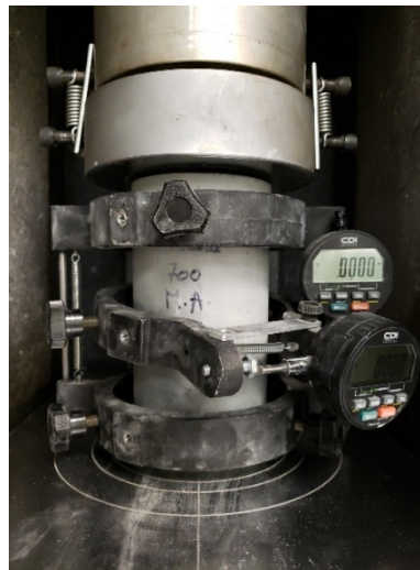
Figure 3.10 Modulus of elasticity test setup
