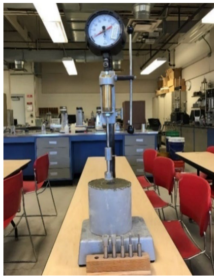
(a) Penetration resistance test
