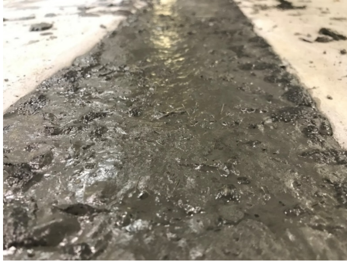
Figure 7.2 Elephant skin on the surface of UHPC allowed to rest
