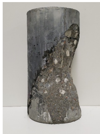
(b) CC failure
