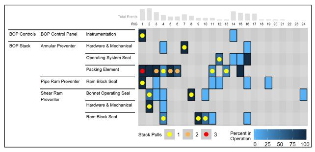
Figure 12: Components Involved in In-Operation Events Leading to a Stack Pull, by Rig, 2016-2018
