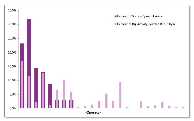
Figure 9: Surface System Events and Rig Activity by Operator
