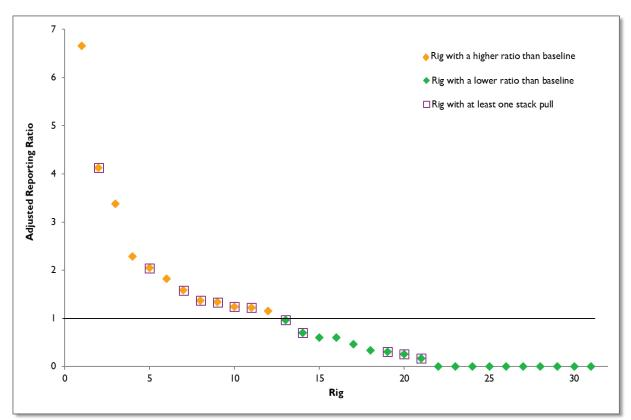
Figure 11: Surface System In-Operation Events Relative to Rig Activity, 2017 & 2018
