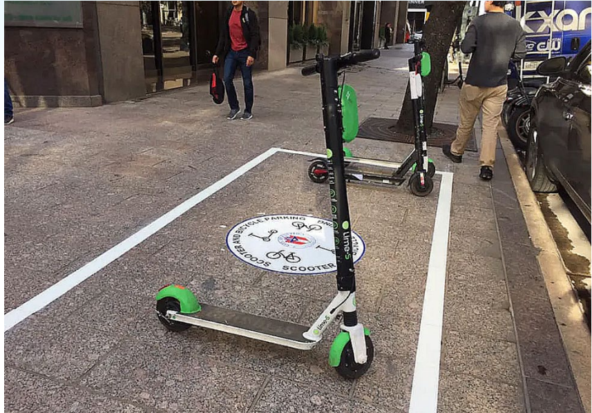
Figure 2: E-scooters parked inside a designated dockless mobility parking box in Central Austin. (Image courtesy of Austin Transportation Department)
