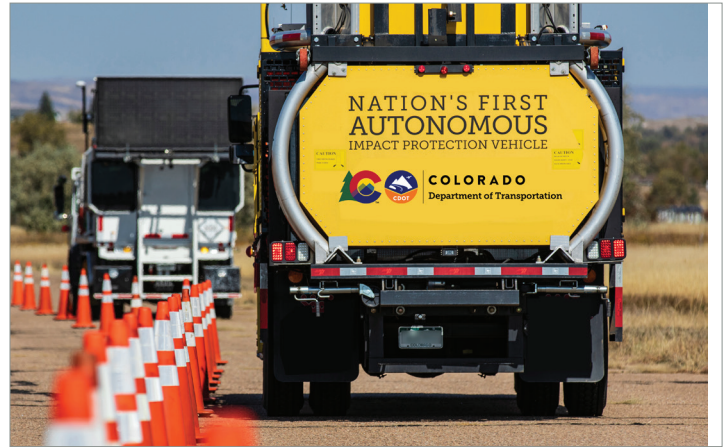
Colorado Department of Transportation tests the autonomous truck mounted attenuator in live work zones to evaluate the safety benefits of autonomous impact protection vehicles in road maintenance. © Colorado Department of Transportation
