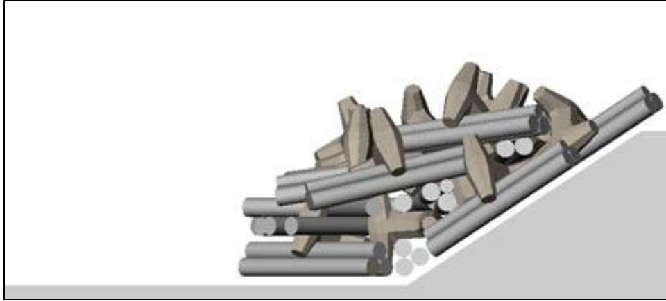
Figure 62. Graphic. Cross-sectional view of the CFD geometry of an ELJ unit.
