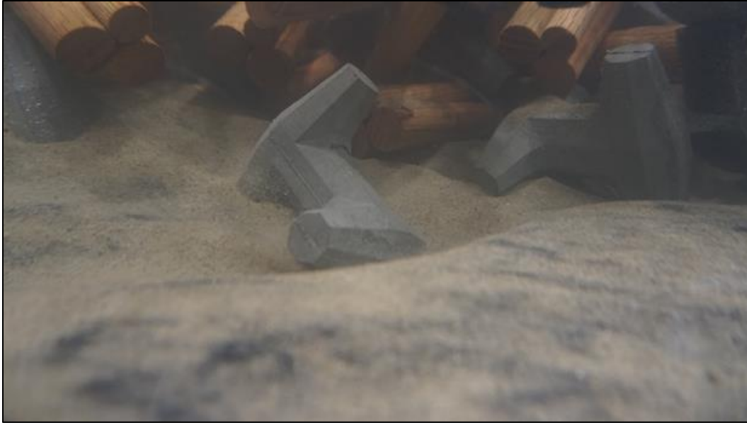
Figure 32. Photo. Total edge failure of key dolosse in run I-2.
