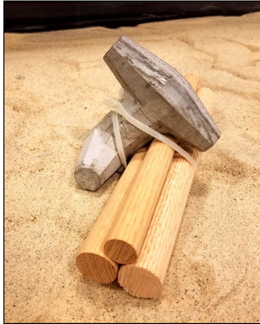
Figure 18. Photo. Fabricated log-dolos bundle (model scale 1:25).
