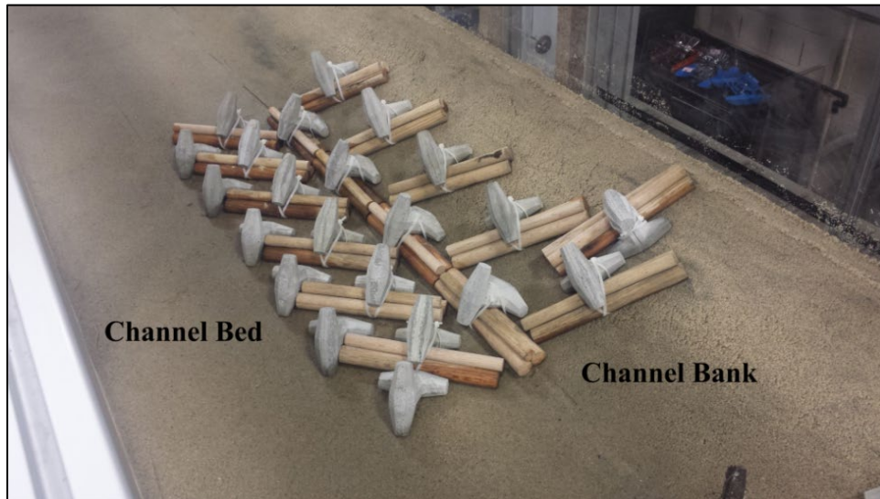
Figure 25. Photo. Installation of the initial layer of log-dolos bundles and key dolosse on the channel bed for run I-3.
