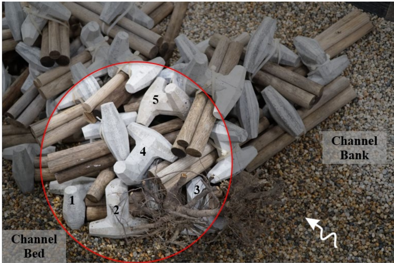
Figure 59. Photo. Close-up view of some single key dolosse (numbered) used to reinforce the upstream face of the ELJ units for run III-9.
