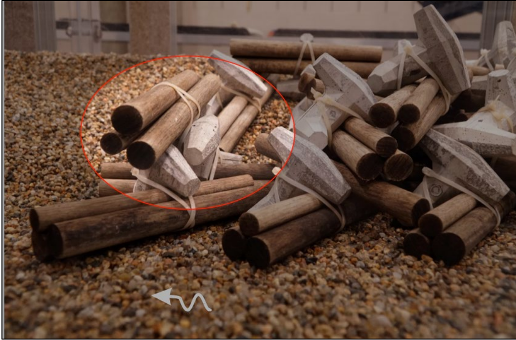
Figure 48. Photo. Log-dolos bundle from ELJ1 (upstream unit) turned upside down.
