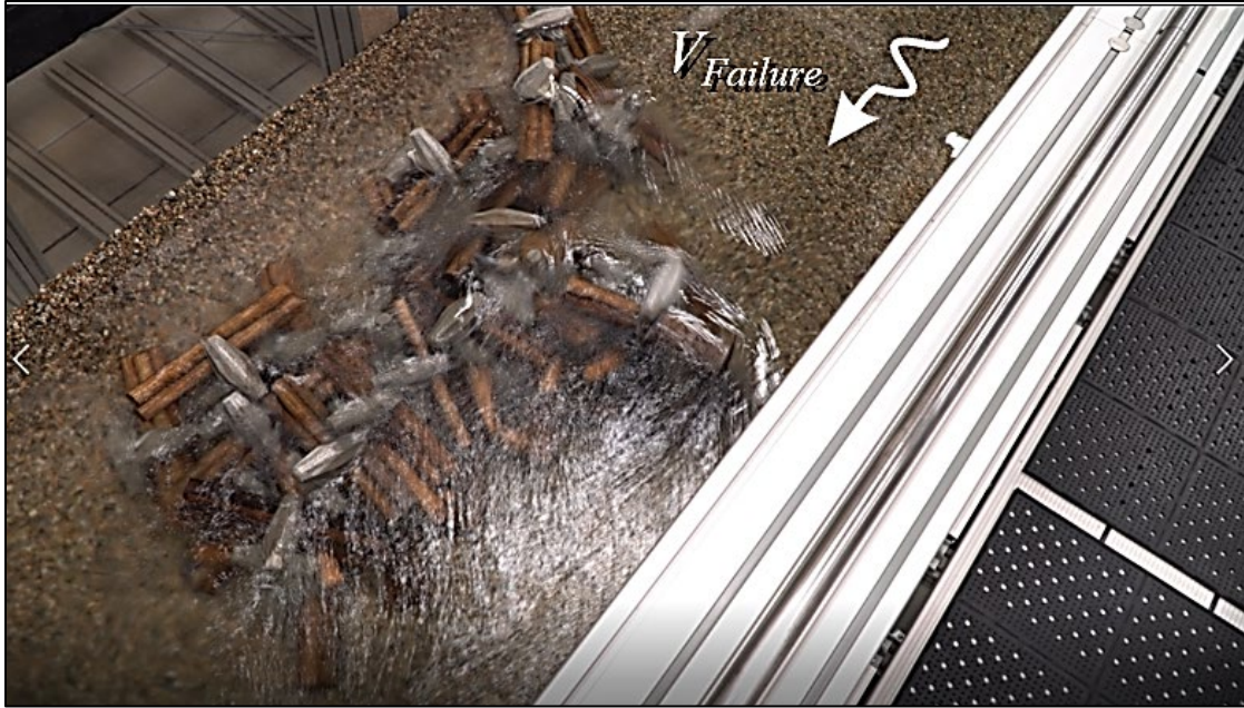
Figure 51. Photo. Advancing failure of ELJ1 during run III-6.
