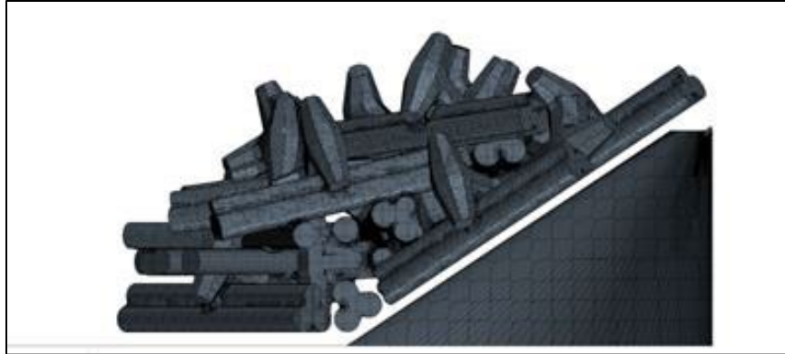
Figure 64. Graphic. Cross-sectional view of an example mesh used for the CFD model.
