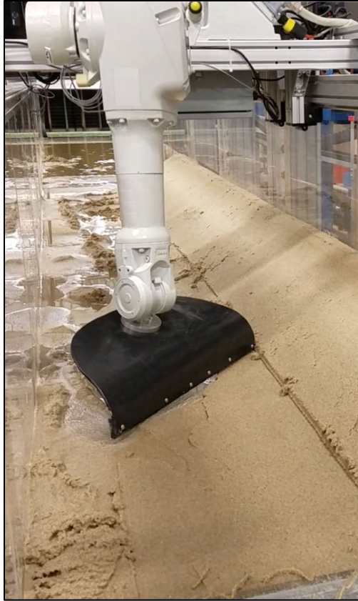
Figure 11. Photo. Robotic arm leveling the channel bed.
