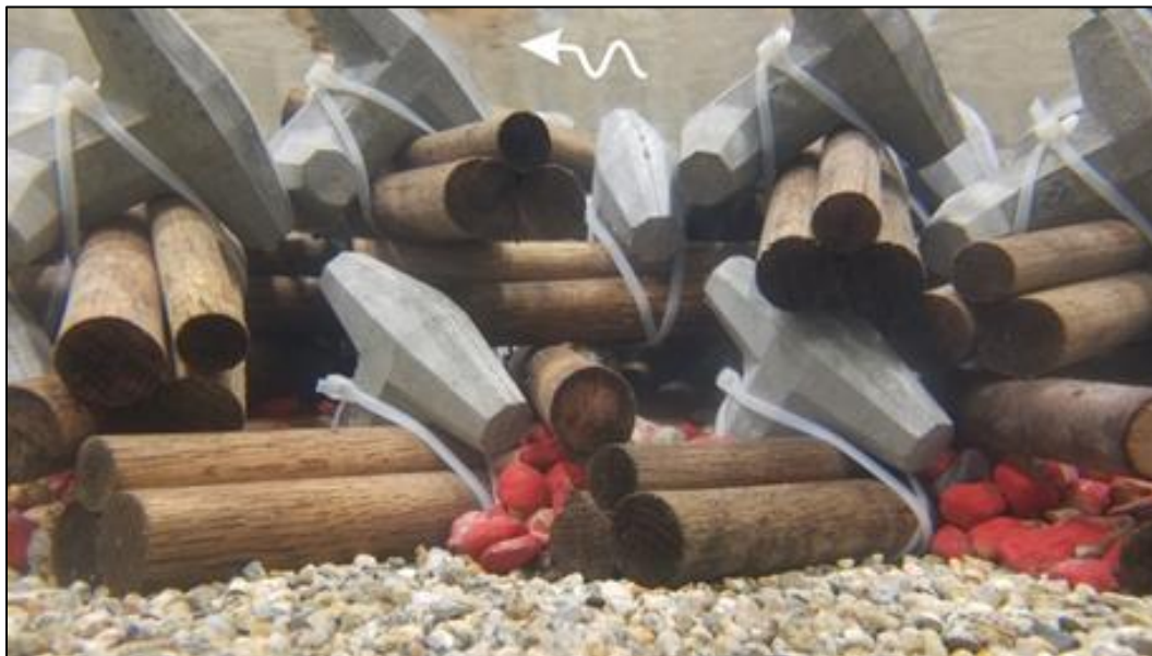
Figure 55. Photo. Close-up of the final installation with layer B on top of layer A for run III-7.
