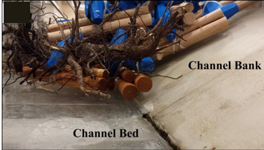
Figure 35. Photo. Close-up view of the suspended ELJ model showing the respective clearances to the channel bed and bank.
