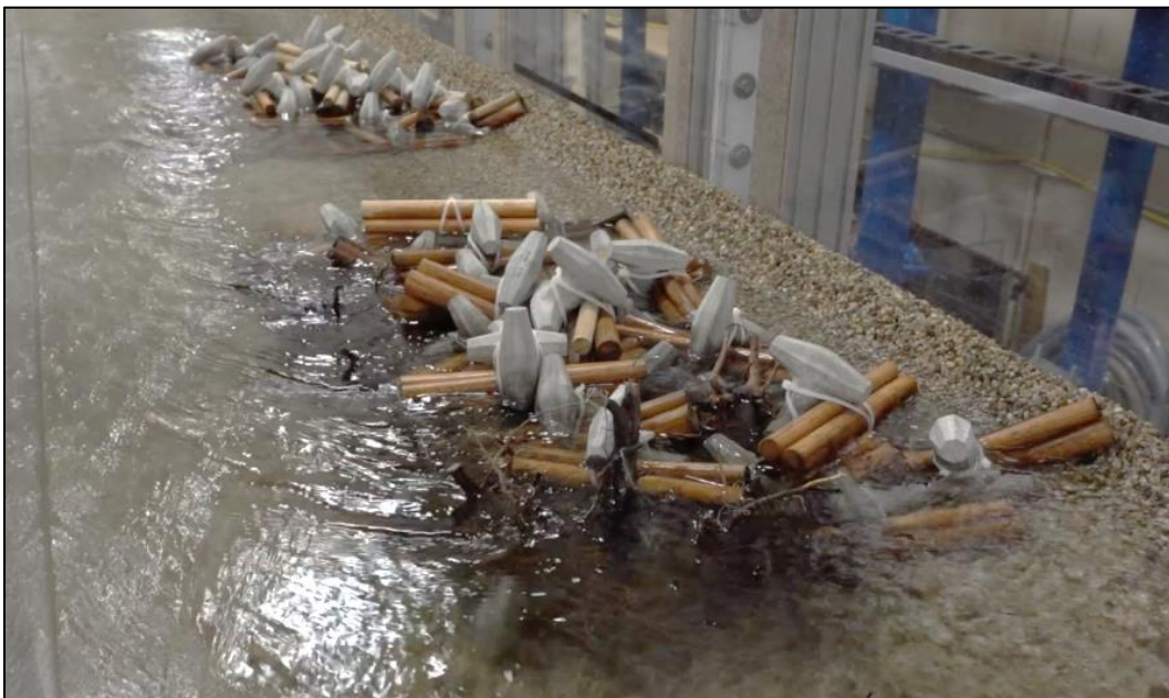
Figure 40. Photo. As-built ELJ installations on the erodible channel for run III-3.
