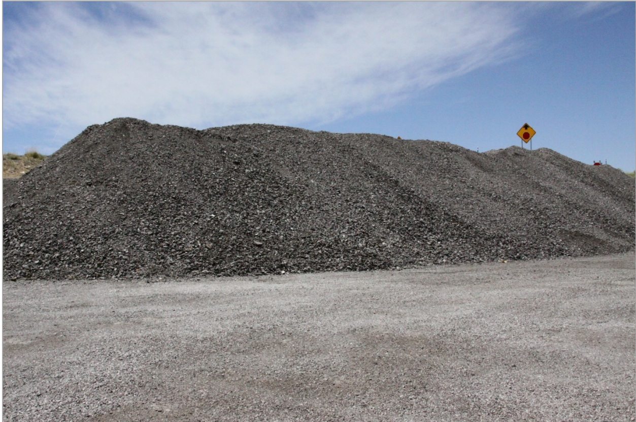
Figure 20. Photo. RAP stored at a ROW on NM 124 prior to crushing and fractionating.
