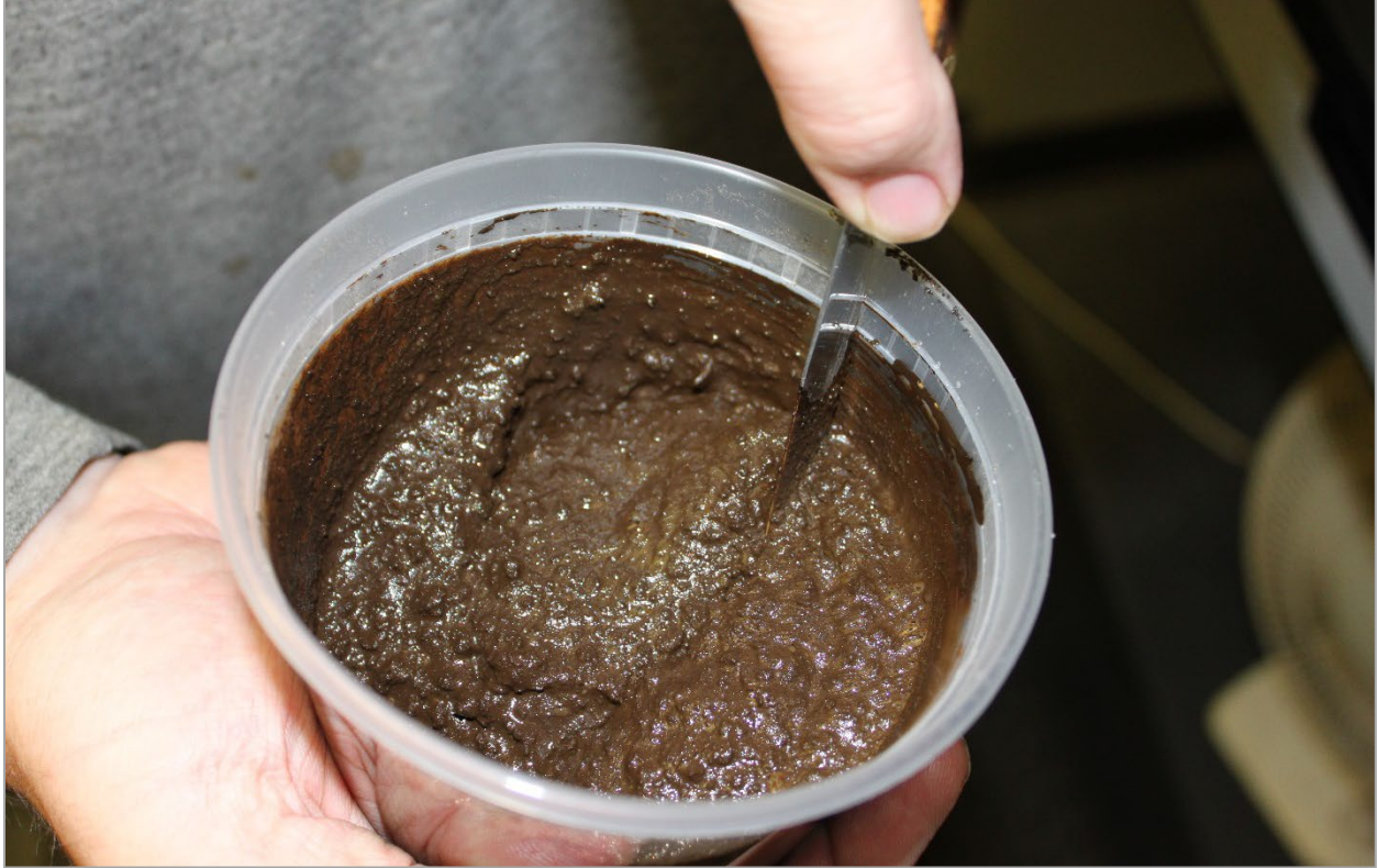
Figure 31. Photo. RAP hand mixed with a trial emulsion.
