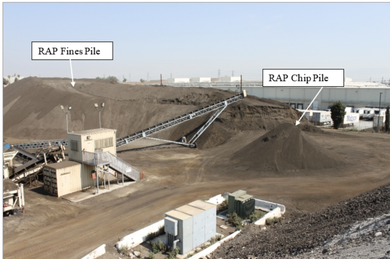
Figure 44. Photo. Market demand causes an imbalance between coarse chip and fine fraction availability.
