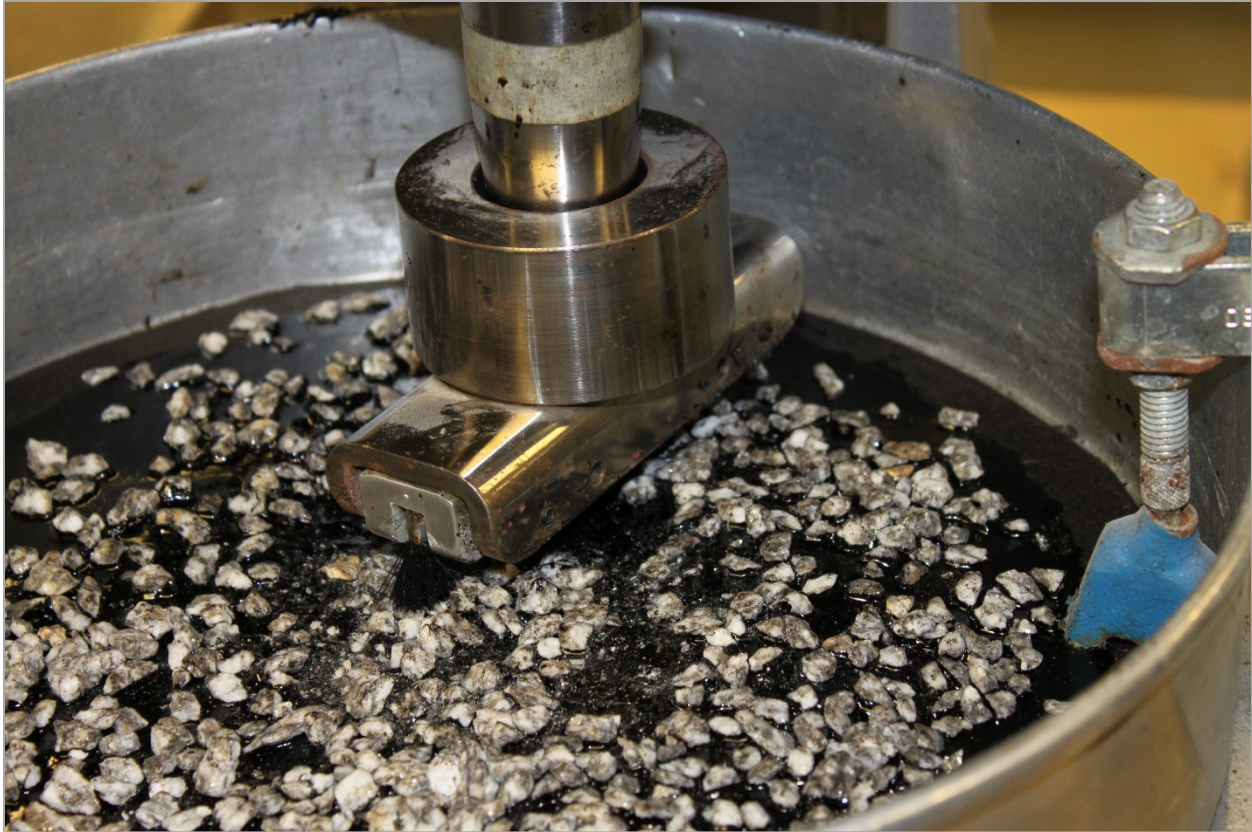
Figure 30. Photo. Testing the bond between asphalt binder and chips.
