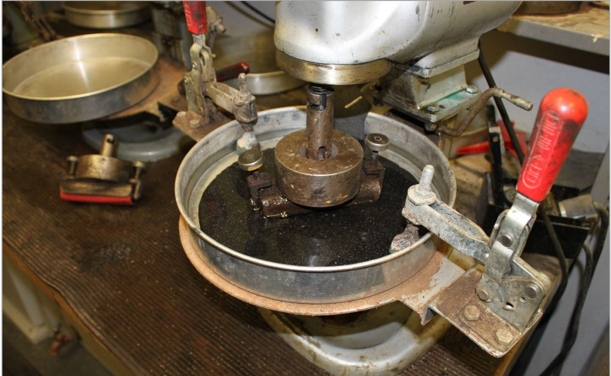
Figure 32. Photo. RAP slurry seal tested using the WTAT.
