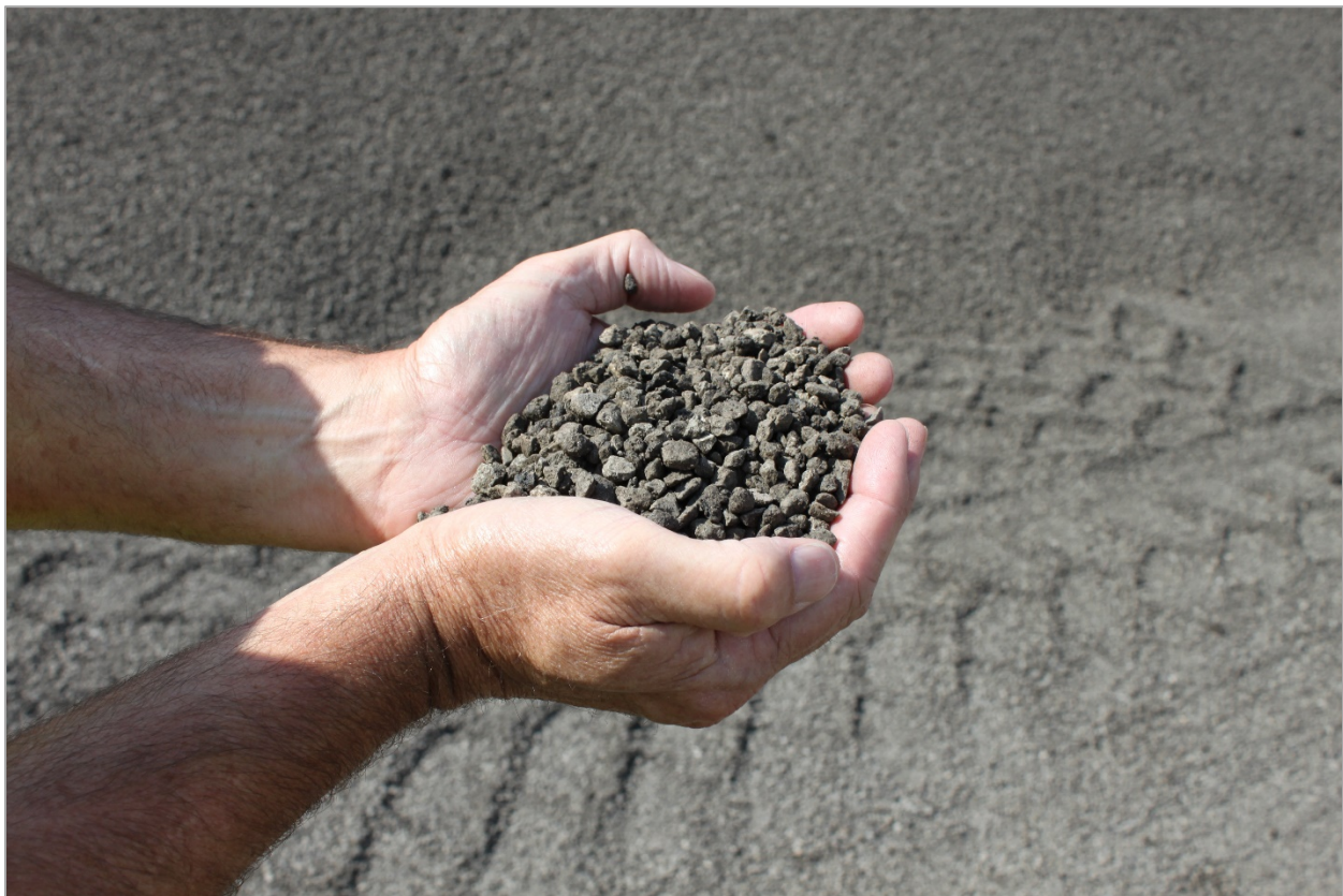
Figure 40. Photo. RAP chips with a partial coating of asphalt and fine aggregate.
