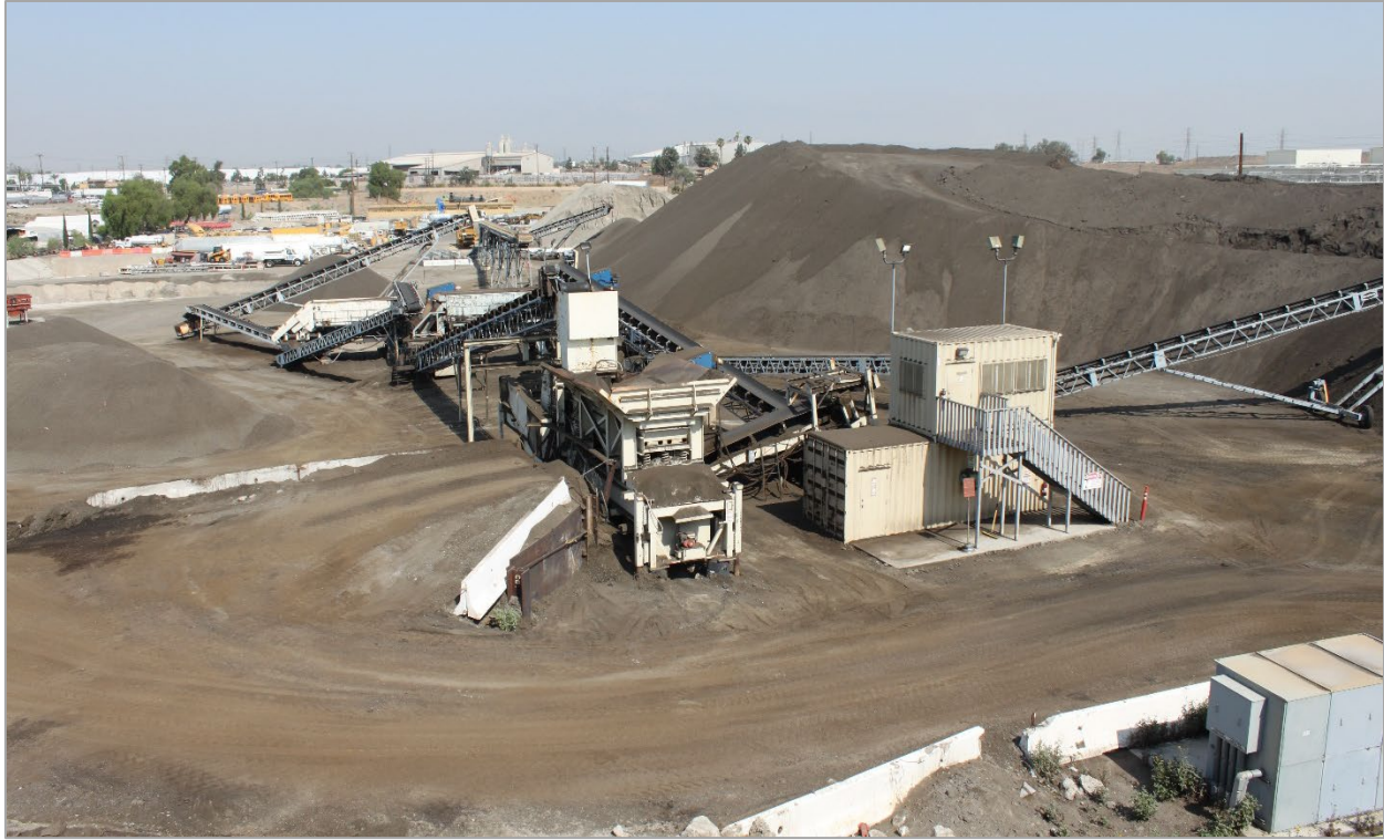
Figure 42. Photo. RAP staging yard with a fractionation plant near San Bernardino, CA.
