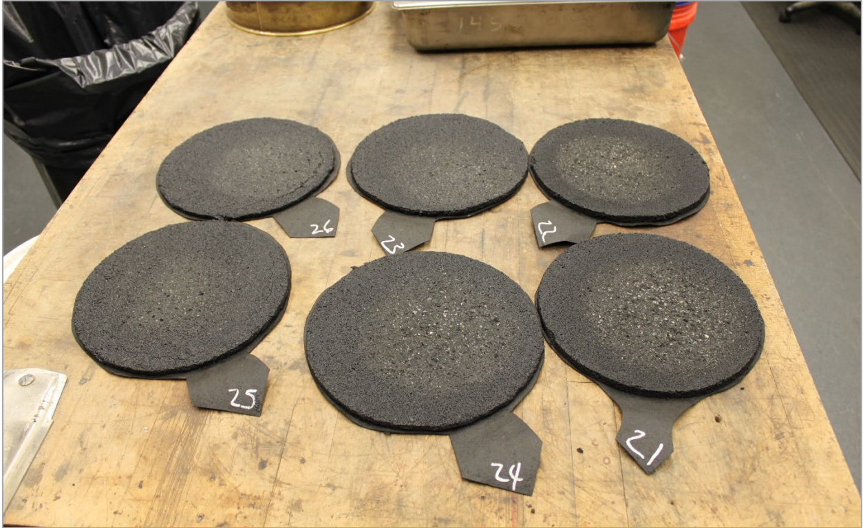
Figure 33. Photo. Slurry seal samples tested using the WTAT to determine the potential for stone loss.
