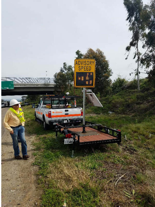
Figure 4.7 Traffic Logix Safespace 650 Variable Message Sign on the roadside
