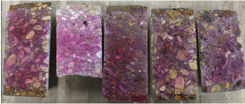
(a) Split Specimens with Phenolphthalein Indicator Sprayed
