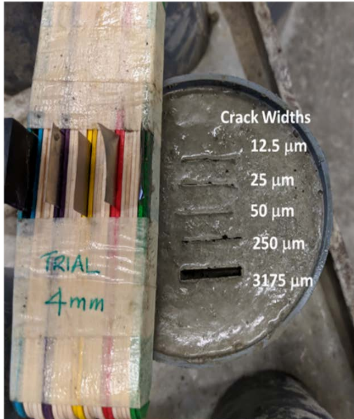
(c) After Removal of Shims
