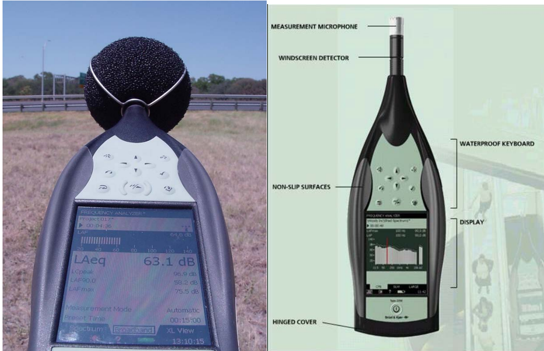
Figure 4.1: Sound pressure level meter
