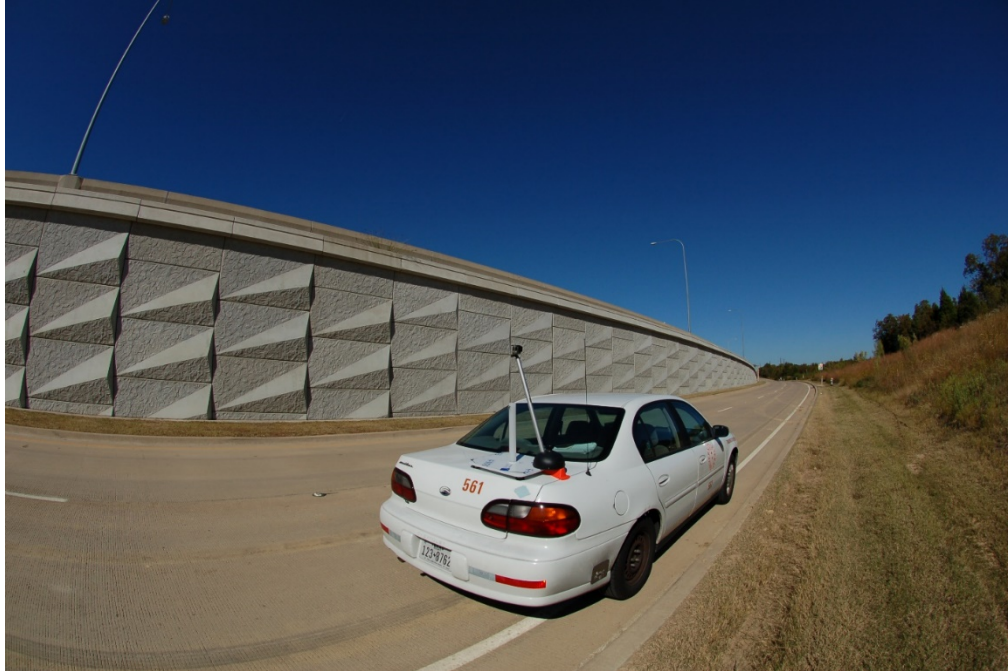
Figure 3.2: GoPro camera mounted on research vehicle on SH 190 prior to recording survey videos
