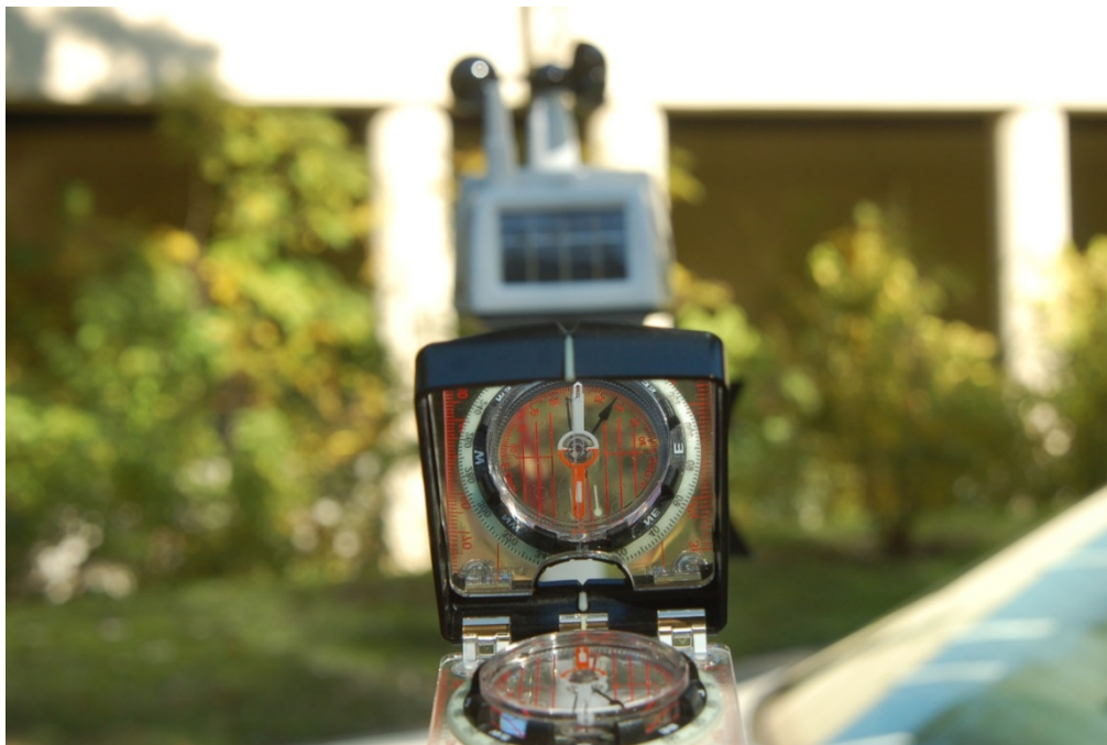
Figure 4.7: Use of the mirror compass for orientation of the weather station: the solar panel of the weather station, in the background, is positioned so that it faces south
