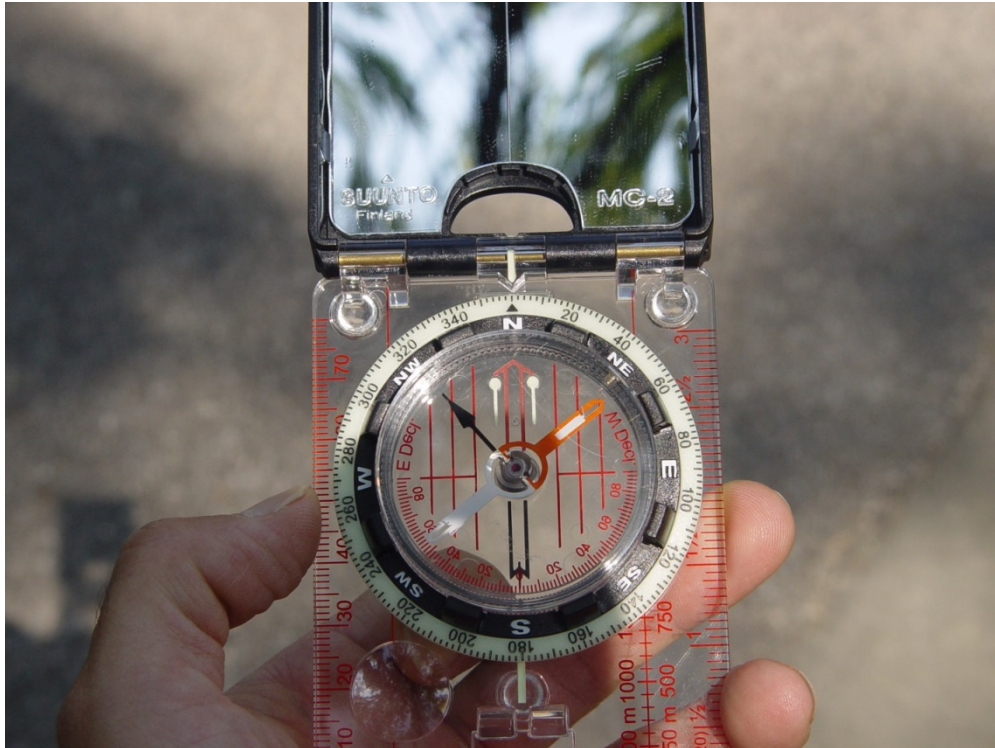
Figure 4.6: Mirror compass utilized for orientation of the weather station
