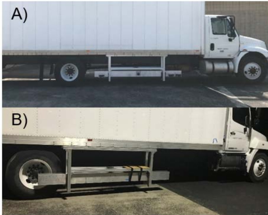
Figure 2-18 DMD locations: A) DMD positioned away from deflection basin, B) DMD positioned to the rear in the deflection basin.
