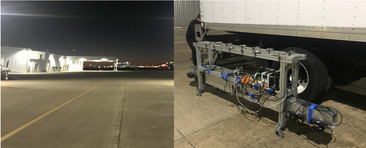
Figure 4-3 Field testing: (Left) section measured with FSF; (Right) DMD assembled with wiring and sensors
