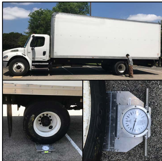
Figure 2-13 Obtaining the weight of the commercial vehicle
