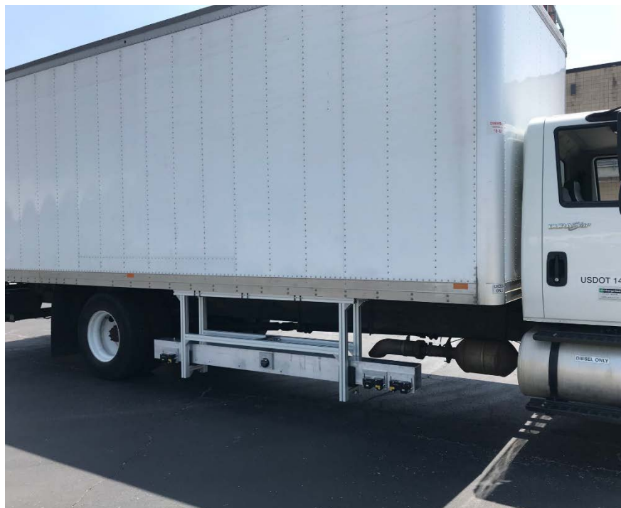
Figure 2-16 Commercial truck with DMD installed
