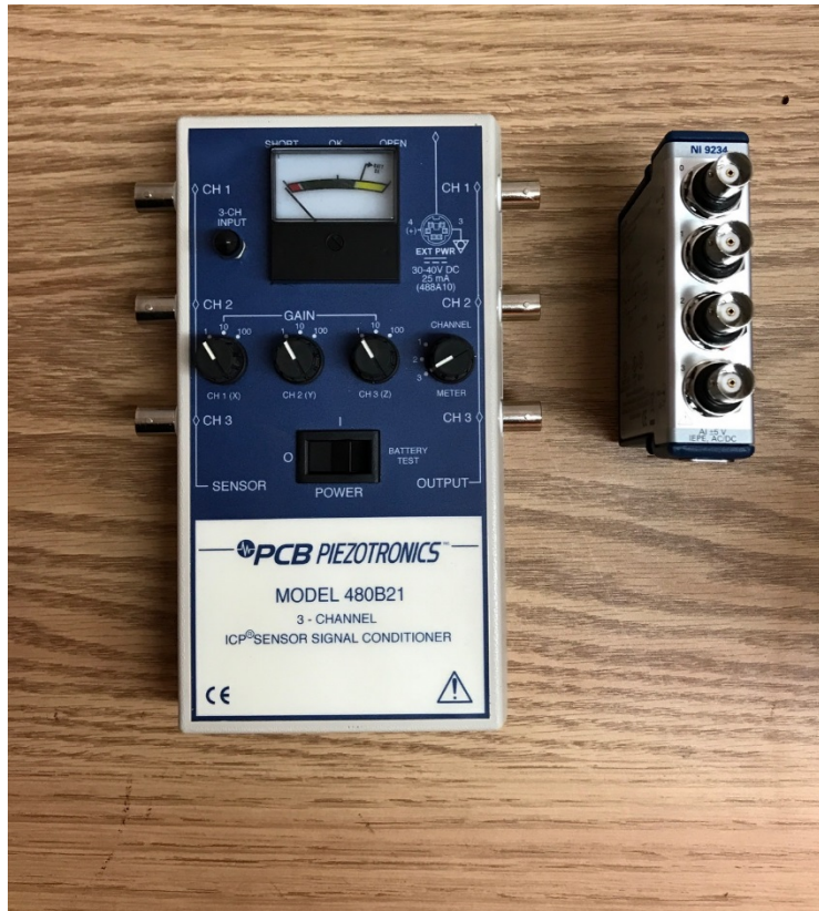
Figure 3-2 Conditioner on the left and DAQ on the right
