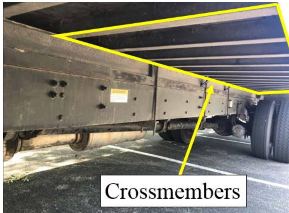
Figure 2-14 View of the undercarriage of a truck
