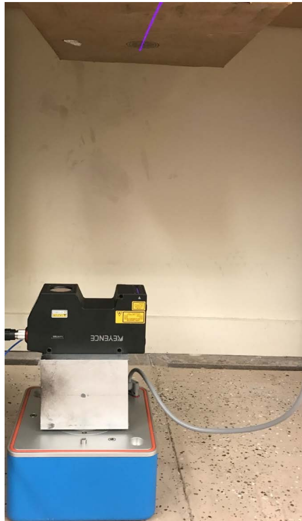
Figure A-3 Laser-sensor fixed to shaker table
