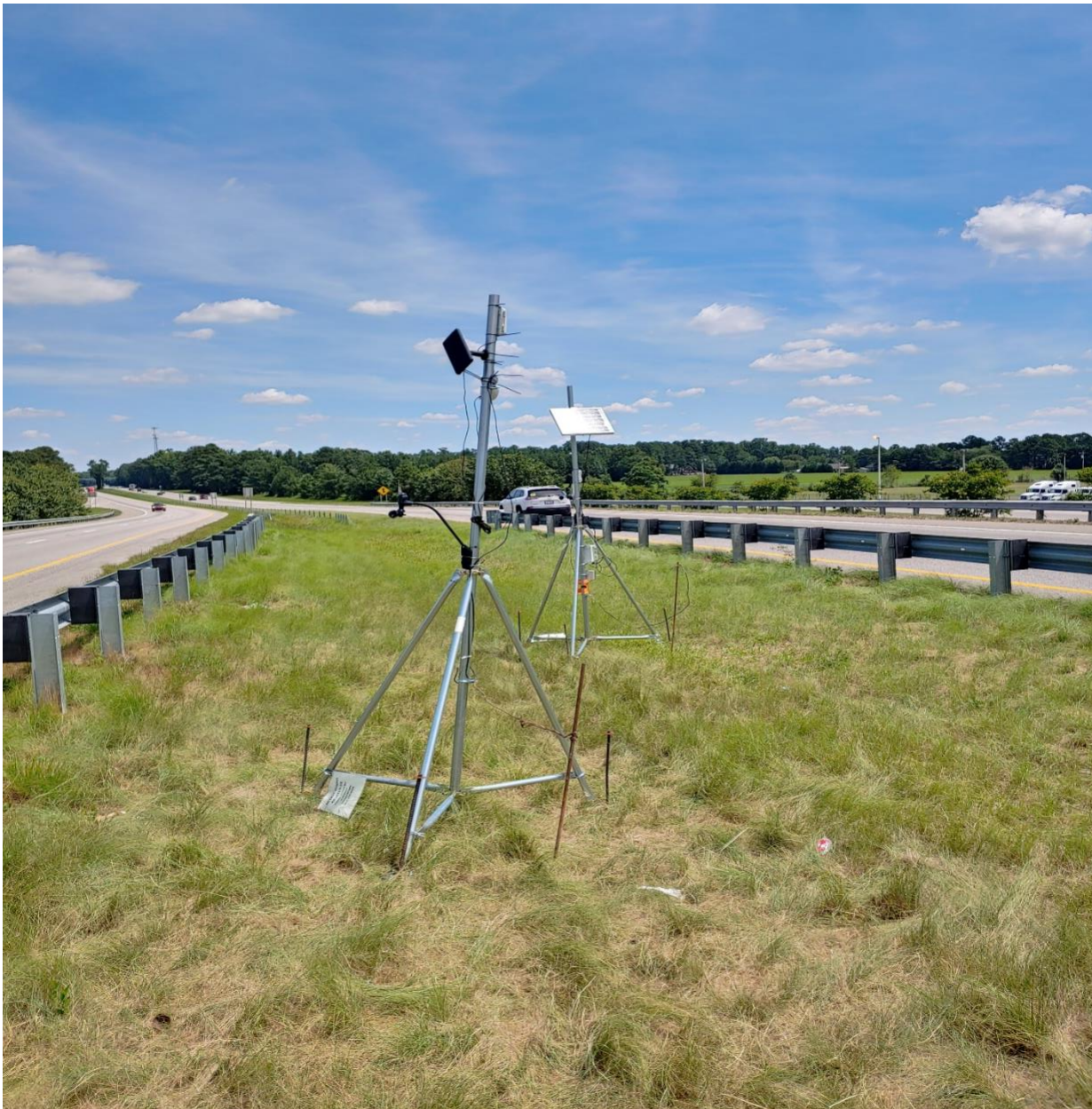
Figure 2-4 Anemometer Installation – NCDOT Highway Division 6, Interstate 95 Median - St. Pauls, Robeson County
