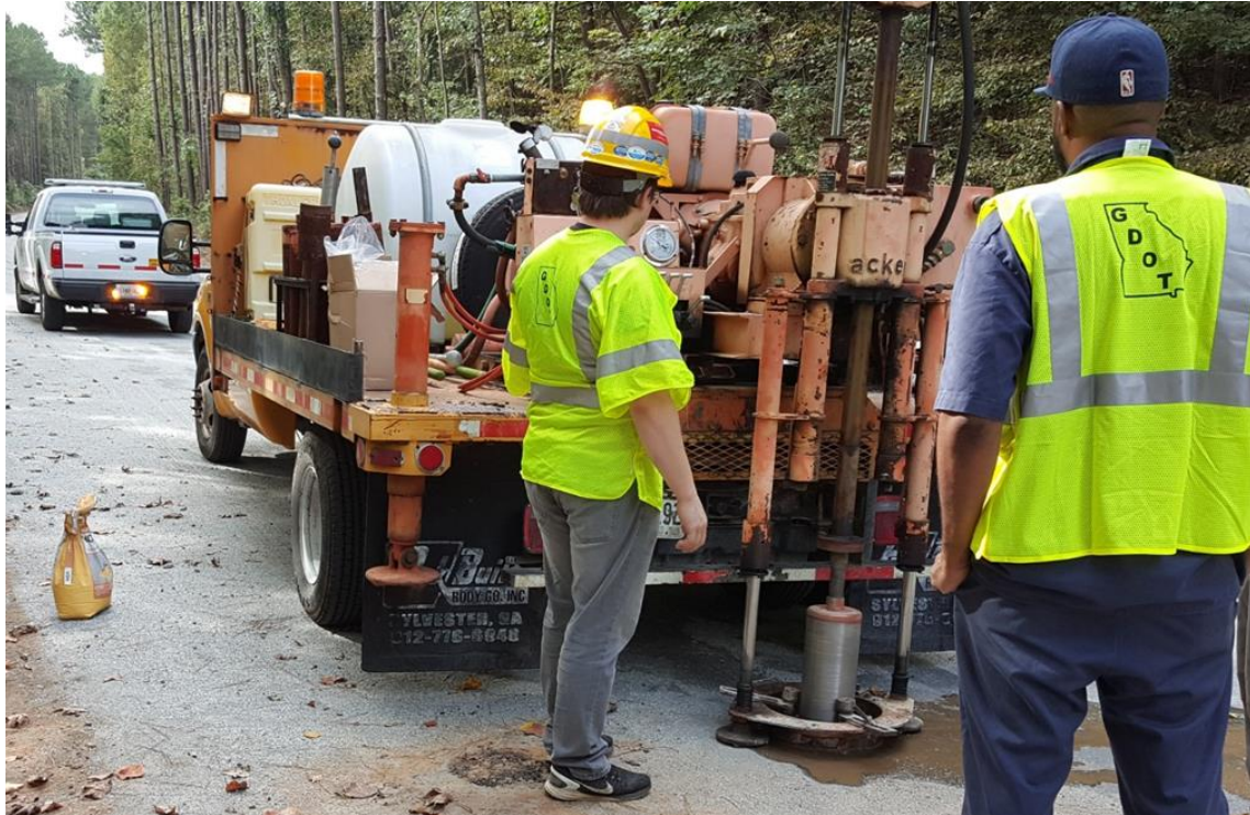
Figure 12. Photo. FDR core sampling for GPR calibration.
