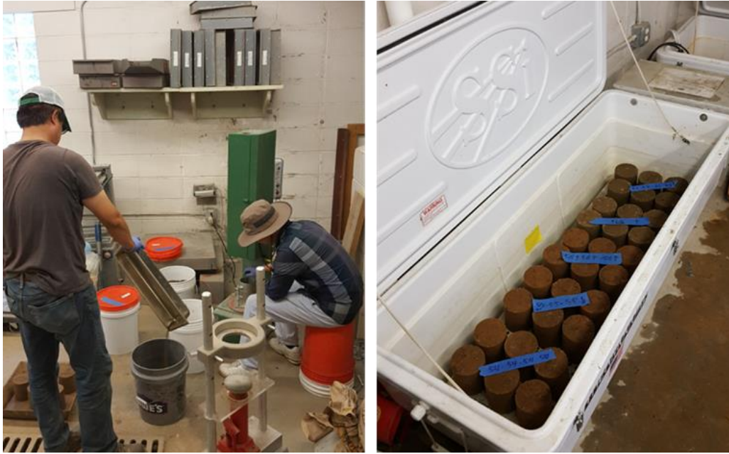
Figure 8. Photos. UCS sample preparation.
