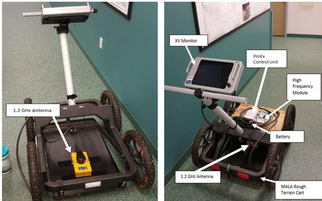
Figure 18. Photos. GPR assembly.
