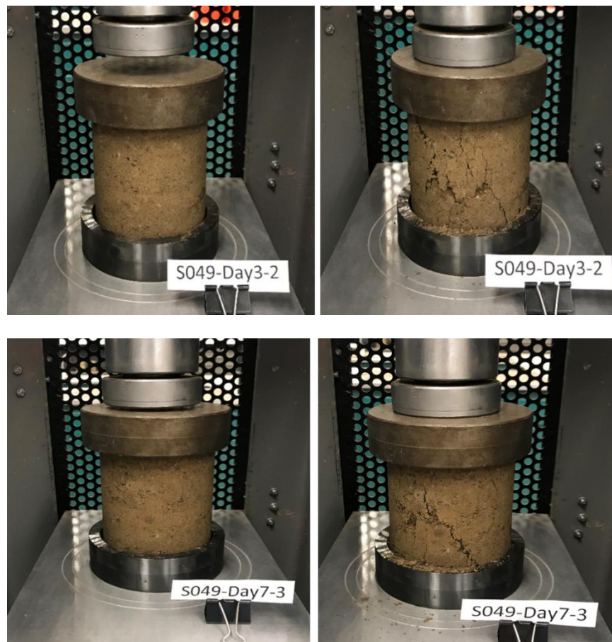
Figure 14. Photos. UCS test.
