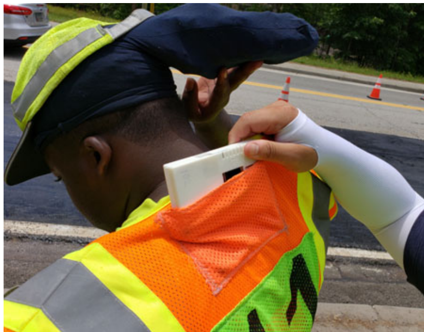
Figure 6. Photo. Placing a PPU to a worker's safety vest.
