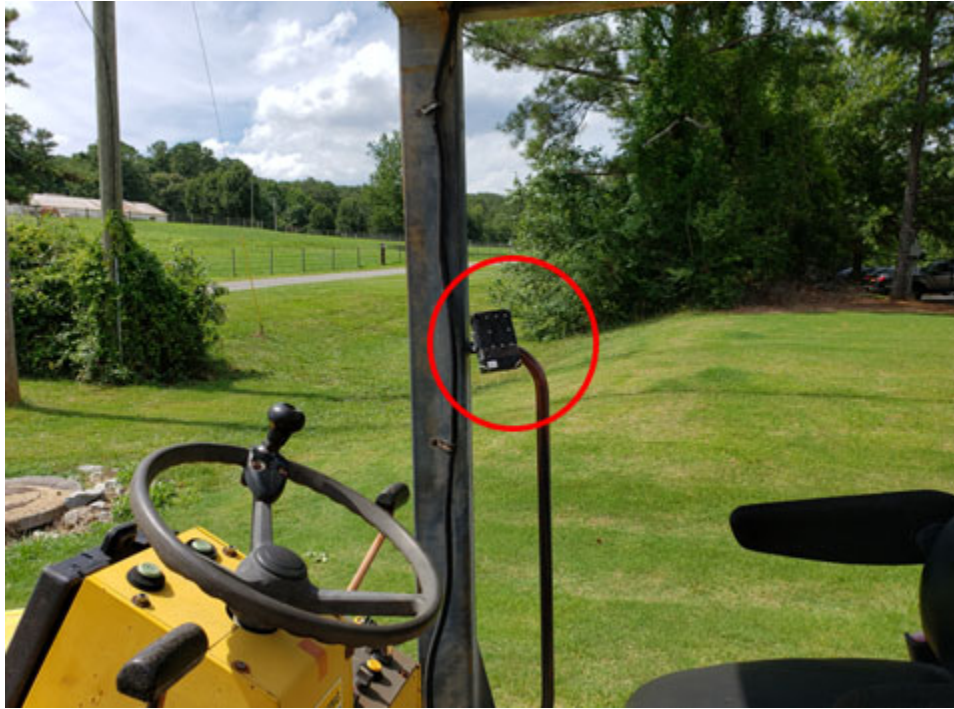
Figure 7. Photo. EPU mounted on the equipment.
