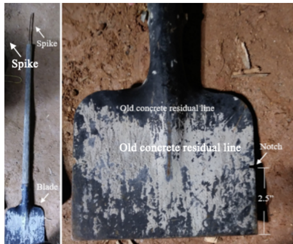
Figure 6. Photo. Modified shovel used to measure concrete cover consisting of a blade end and a spiked end. An expanded view of the blade shows the right-side notch, which is located 2.5 inch from the blade's edge.
