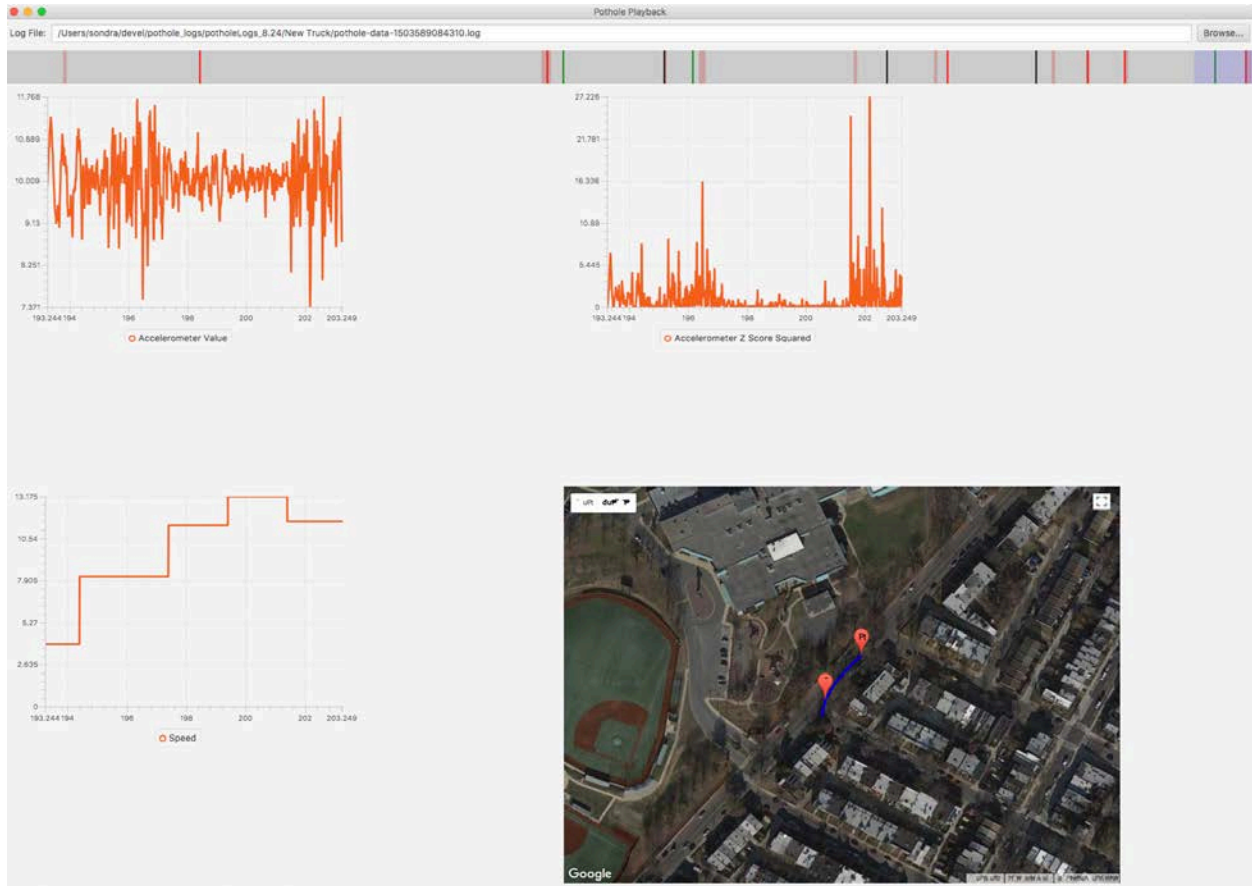
Figure 14: Pothole Detection Speed and Accelerometer Charts
