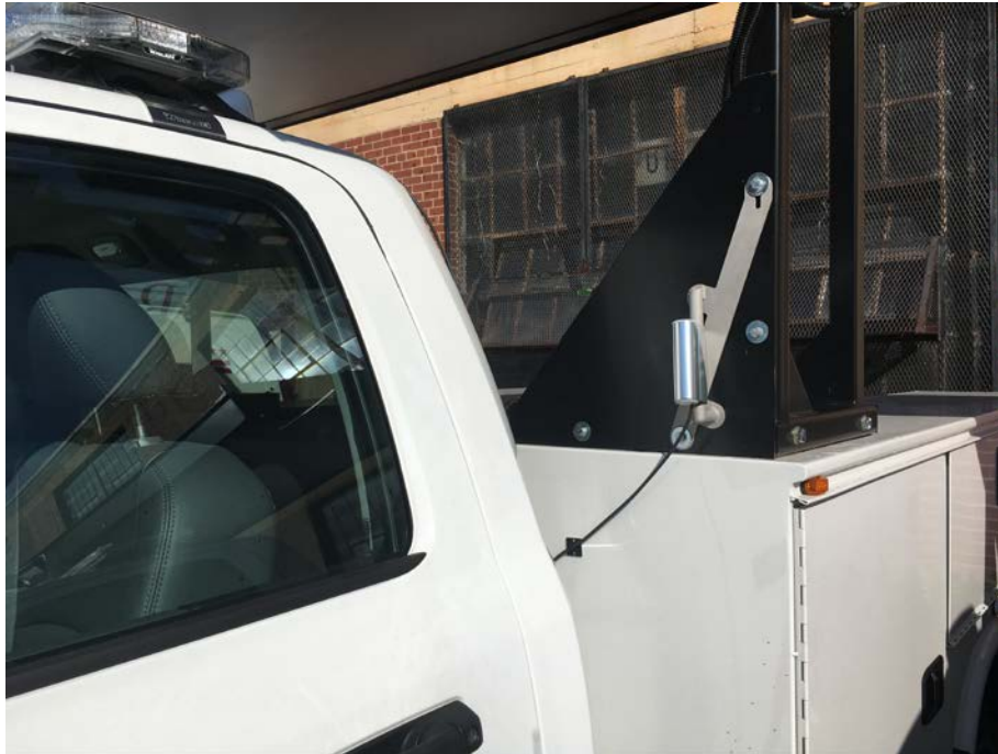
Figure 7: Installed Road Watch Weather Sensor
