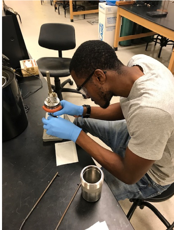
Figure 41. Photo. Calorimeter (energy) analysis of switchgrass.
