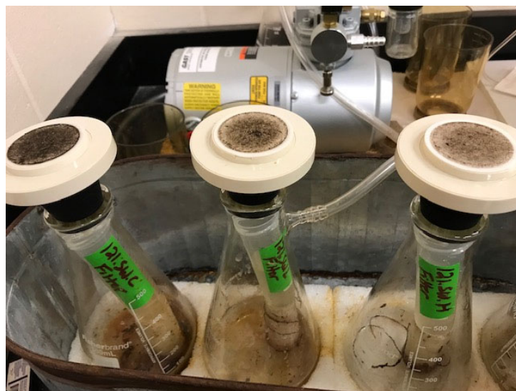
Figure 42. Photo. Total suspended solid analysis on water samples collected beneath feedstocks.
