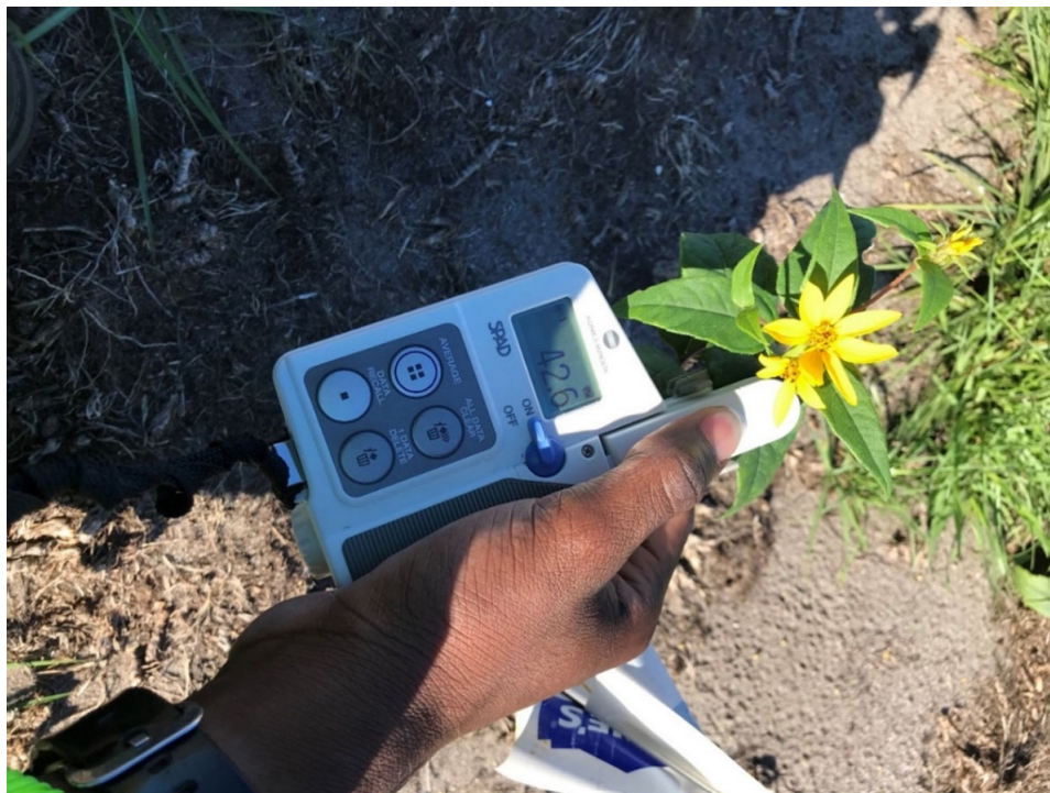
Figure 38. Photo. Soil pant analysis development (SPAD) measurements of woodland sunflower.
