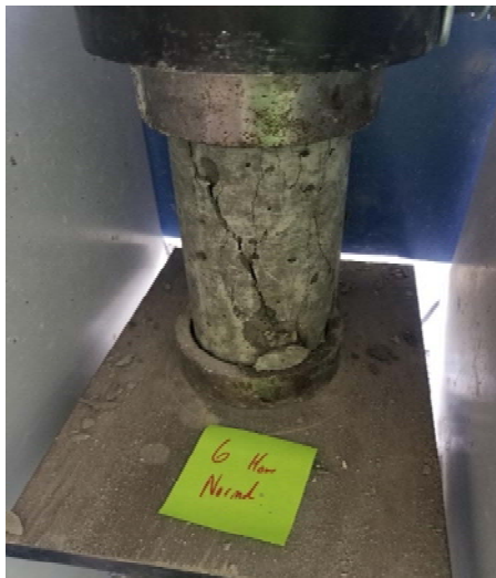
(a) Air-Dry Specimen (b) Oven Dry Specimen Figure 40. Specimens Tested after 6 Hour Curing
