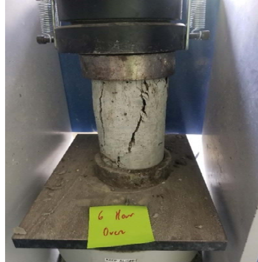
(a) Air-Dry Specimen (b) Oven Dry Specimen Figure 40. Specimens Tested after 6 Hour Curing
