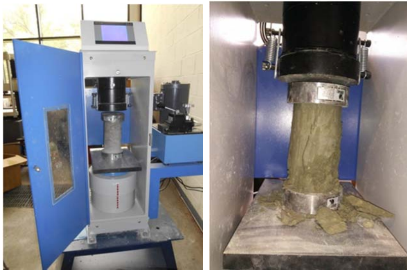
Figure 6. Compression Tester and 4-hour Compression Test
