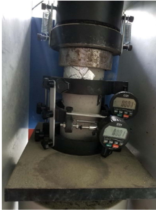
Figure 48. Test Set-up for the Elastic Modulus of Concrete Cylinder
