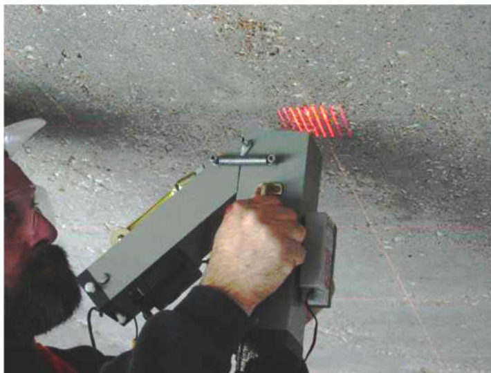
Figure 2-7. Laser Profilometer (Holdener et al. 2004)
