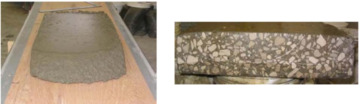
Figure 2. Concrete slab produced by the mini paver test set up (left) and the cross section of the slab (right) [3]
