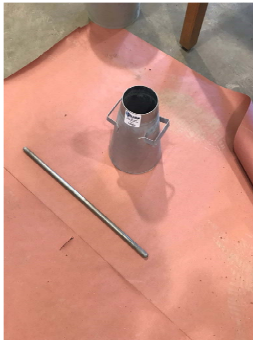
Figure 9. Slump test apparatus
