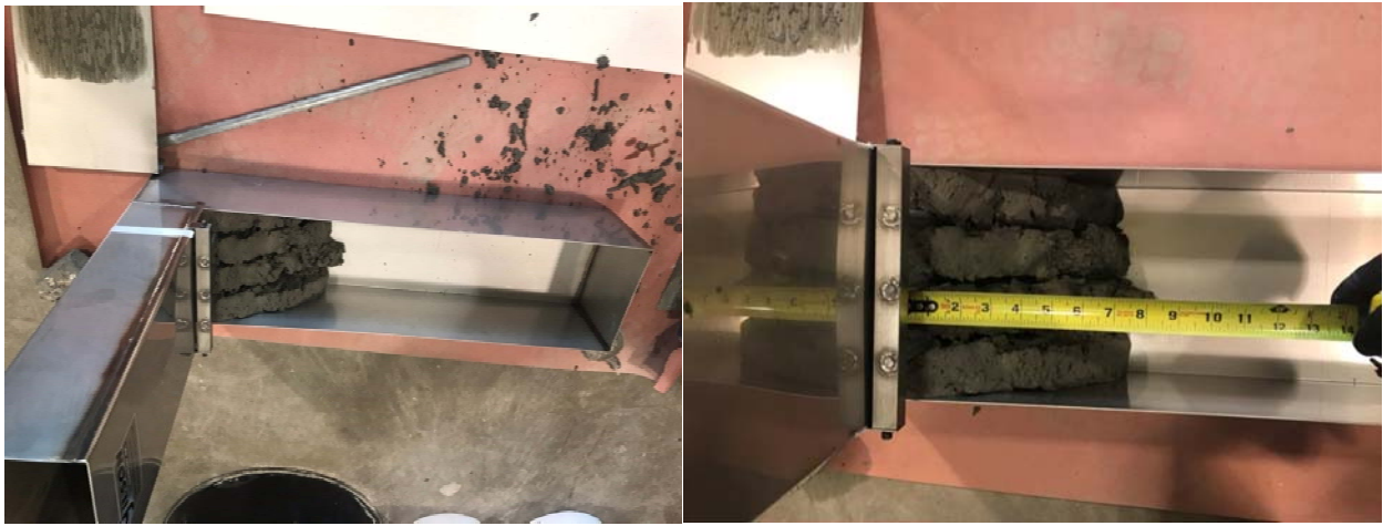
Figure 17. L Box test (Mixing design AC)
