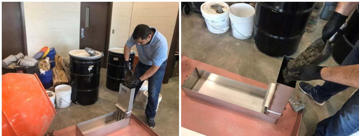
Figure 16. L Box test (Mixing design SL-B-AC)
