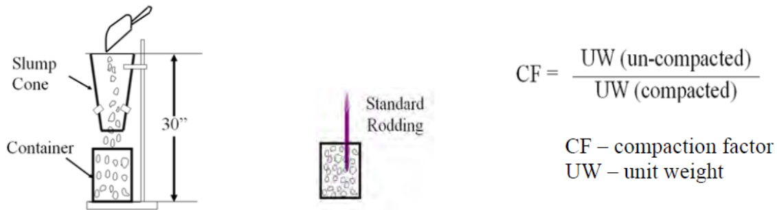
Figure 10. Compaction factor test setup [6].
