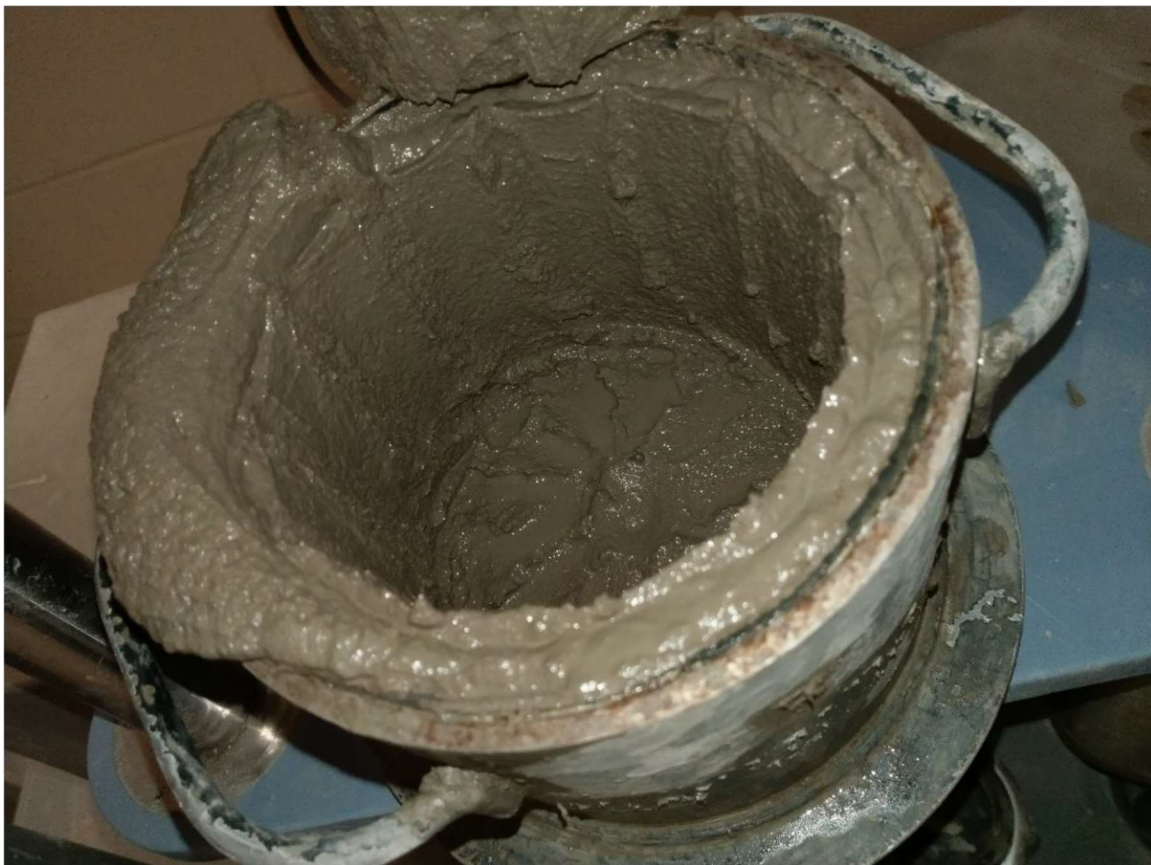
Figure 45. Vertical standing walls of mortar inside the rheometer after the test indicate the test might be invalid.
