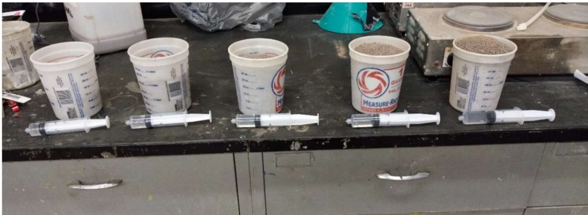
Figure 42. Prepared quantities of sand and water for different volume fractions.
