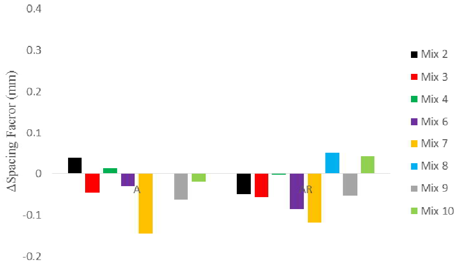
Figure 129. Change in spacing factor due to pumping with a reducer (right), compared to omitting the reducer (left) for mixtures 2-10.
