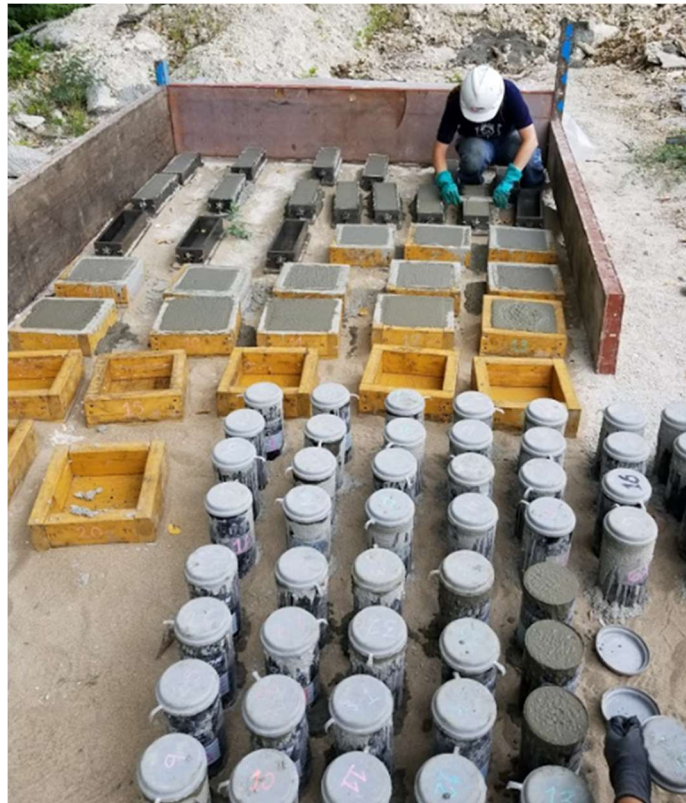
Figure 57. Production of cylinders, freeze-thaw bars and scaling slabs in the field. After completion of all specimens, they were covered with a plastic sheet to minimize evaporation.
