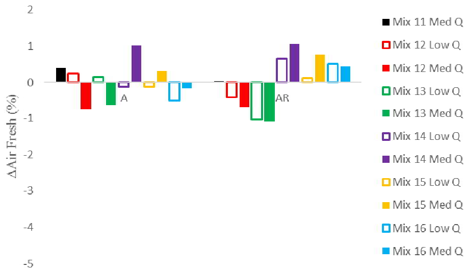
Figure 102. Change in fresh air content in A configuration (left) and A-R configuration (right) for mix designs 11-16.
