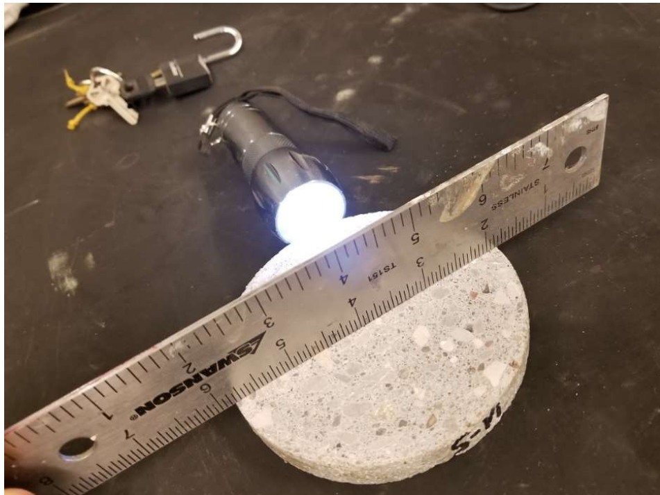
Figure 52. Verification of flatness of surface after each polishing step.
