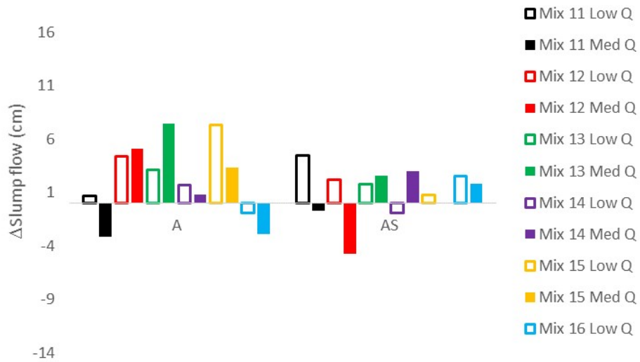
Figure 73. Change in slump flow when submerging the hose at different flow rates (left A, right A-S) for mixtures 11-16.
