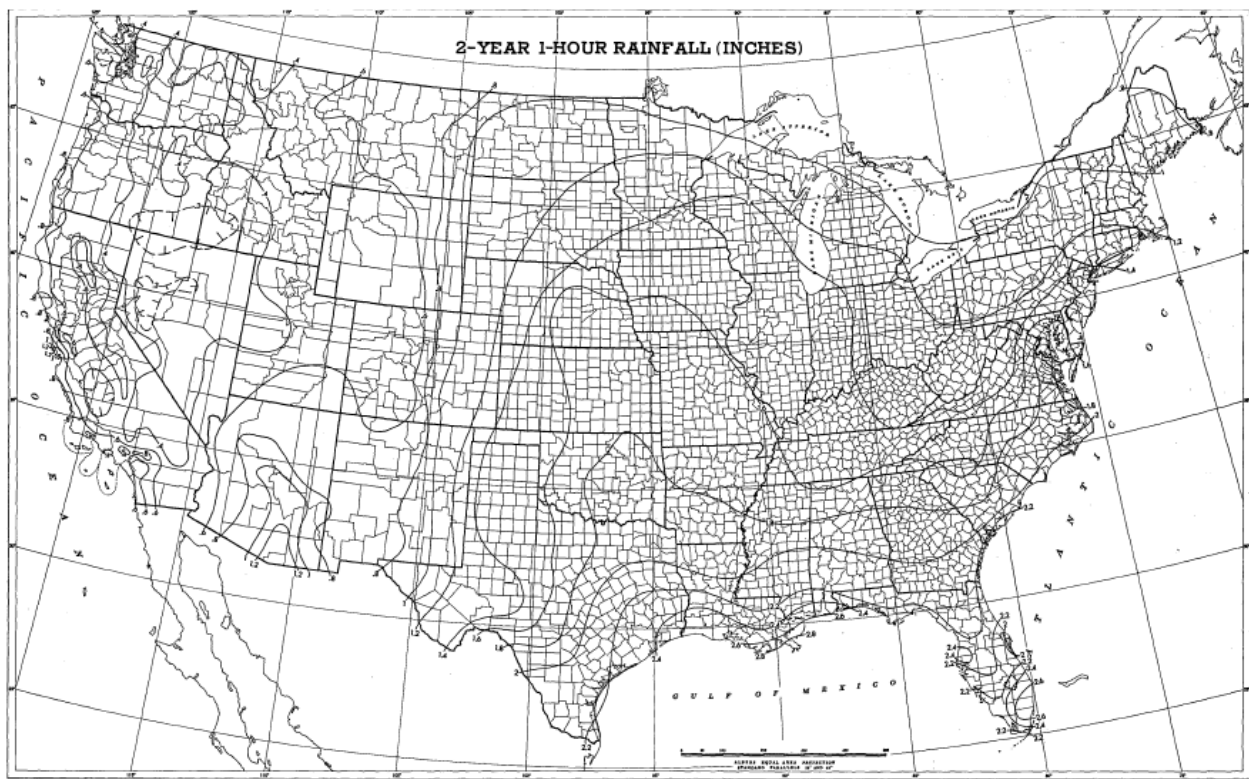
Figure 7. 2-Year, 1-Hour Precipitation Depth Contour Map from Rainfall Frequency Atlas of the United States.
