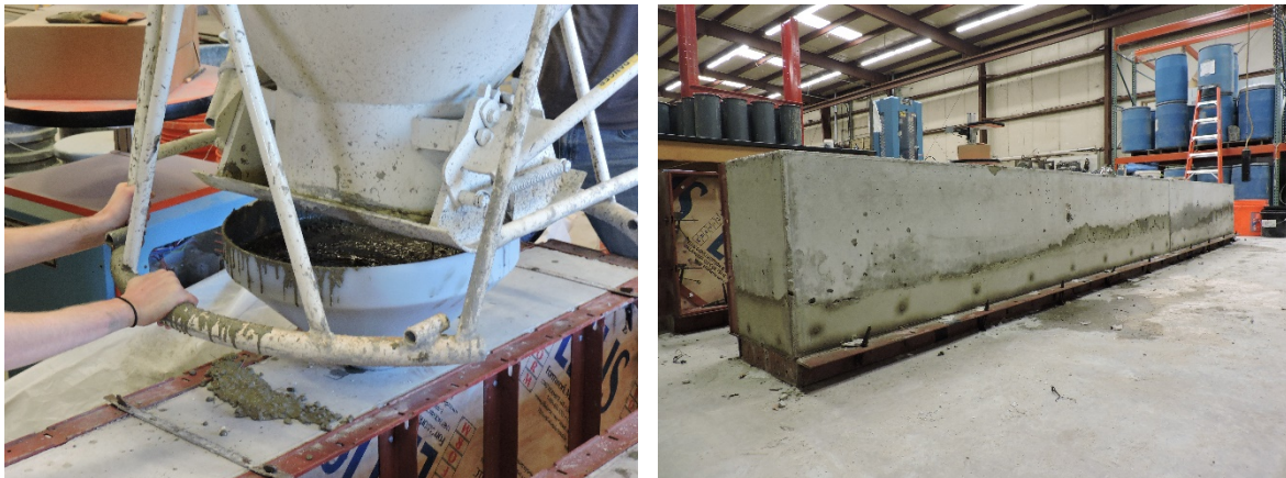
Figure 5.12: Placement of FR-SCC Repair Material (l) and Completed Specimen (r)
