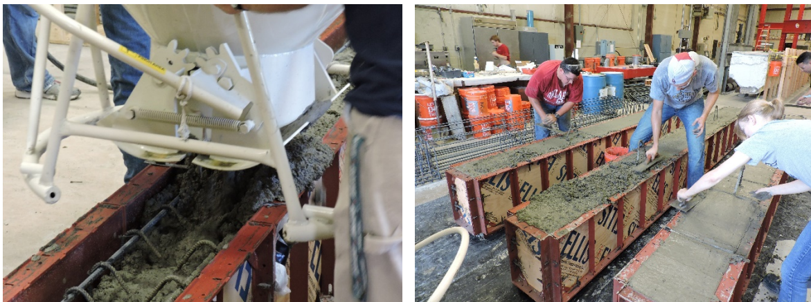
Figure 5.4: Full-Scale Control Beam Specimen Concrete Placement (l) and Finishing (r)
