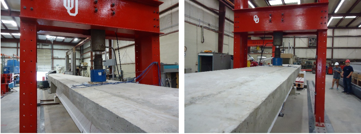
Figure 6.7: AASHTO Girder C1 Test Setup
