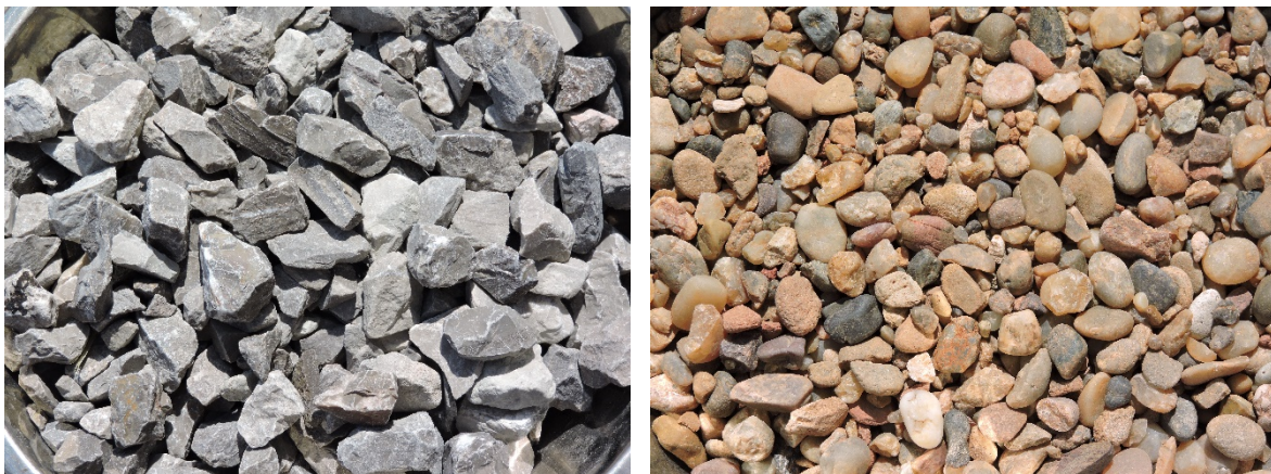
Figure 2.2: #57 Limestone (l) and #7 River Gravel (r) Coarse Aggregates
