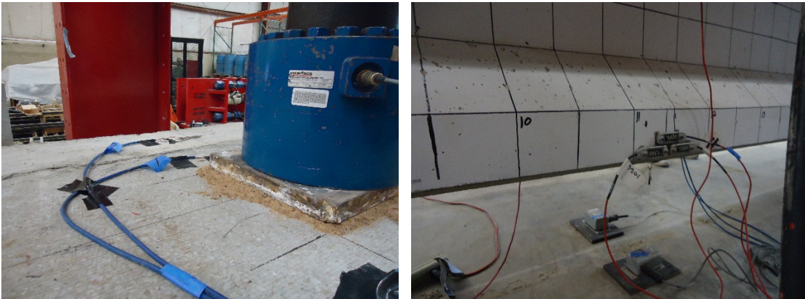
Figure 6.8: AASHTO Girder Instrumentation, Load Cell (l) and Wire Pots (r)
