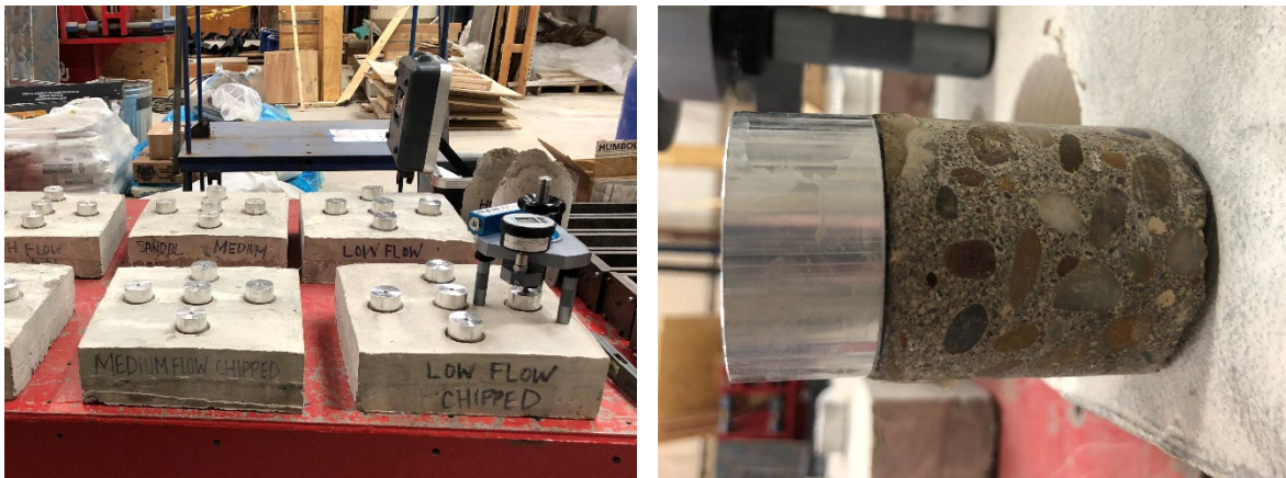
Figure 4.2: Pull-off Test Setup (l) and Pull-off Test Specimen (r)
