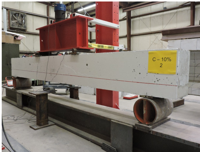
Figure 5.14: Photograph of Full-Scale Beam Specimen Test Setup
