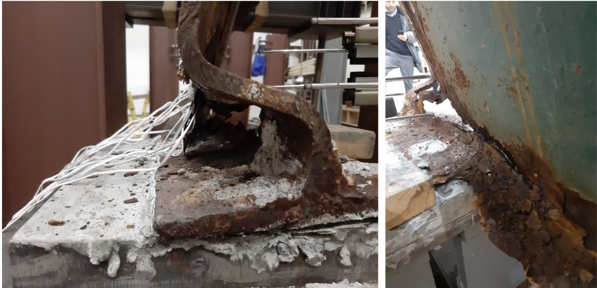
Figure 6.33: Residual deformation of corroded end after unloading.
