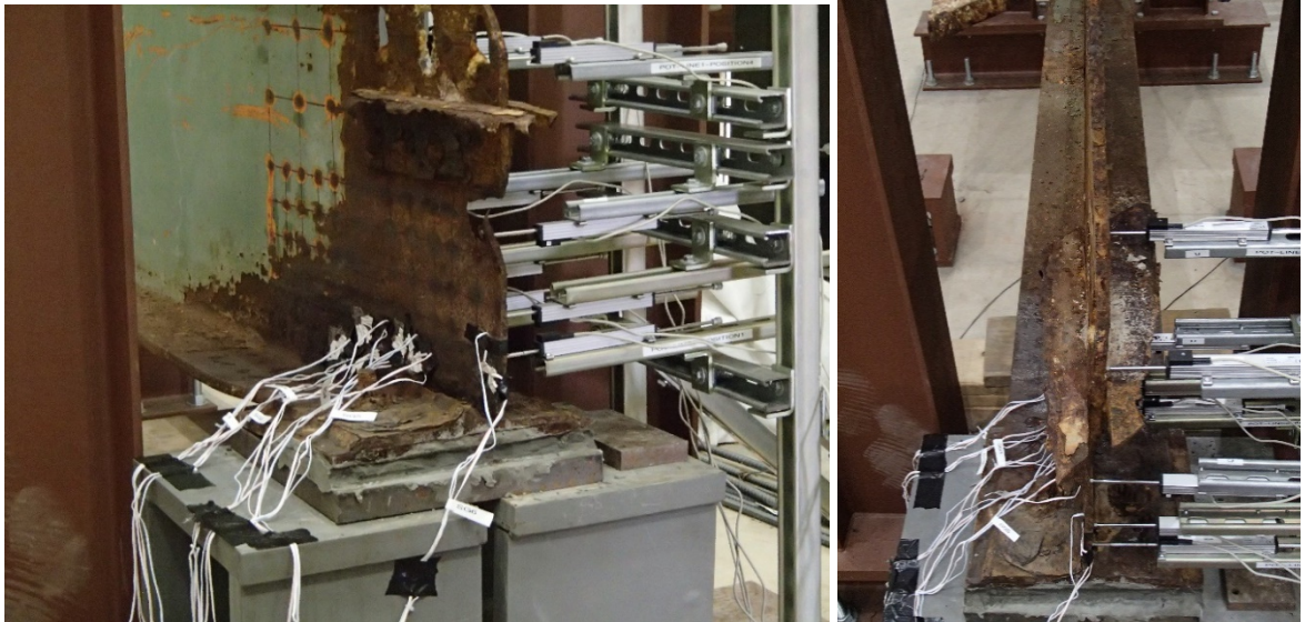
Figure 3.18: Instrumentation configuration at corroded end of Specimen 1.
