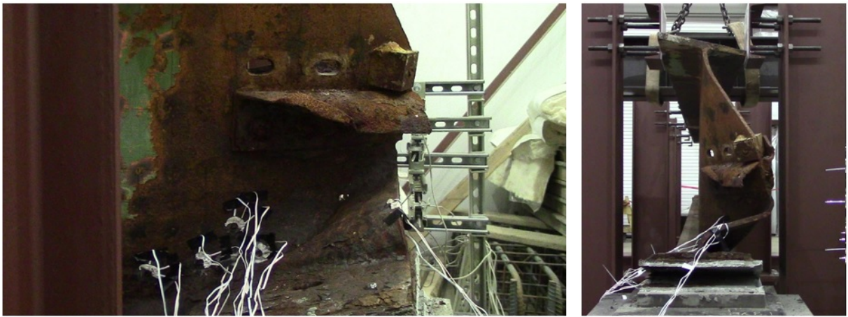
Figure 6.10: Side-by-side images showing side view of web and profile view of beam during experiment. Letters A-E correspond to Figure 6.8a.
