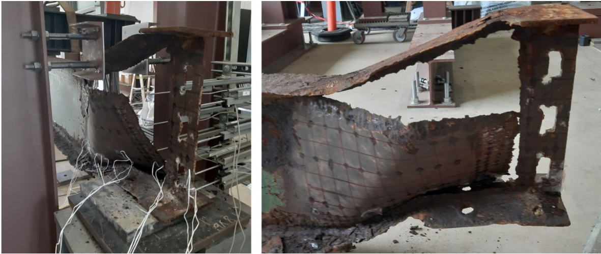
Figure 6.41: Residual deformation of Specimen 6.
