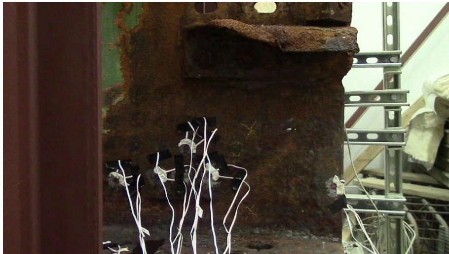
Figure 3.26: Instrumentation configuration at the end of Specimen 2.
