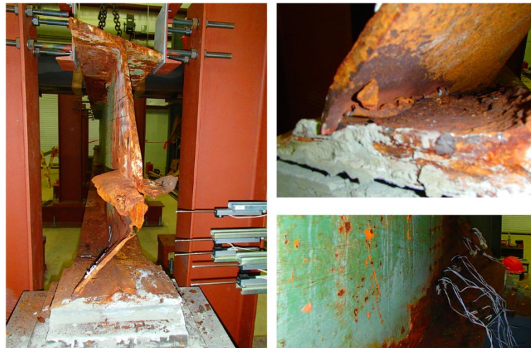
Figure 6.19: Residual deformation after unloading Specimen 3.
