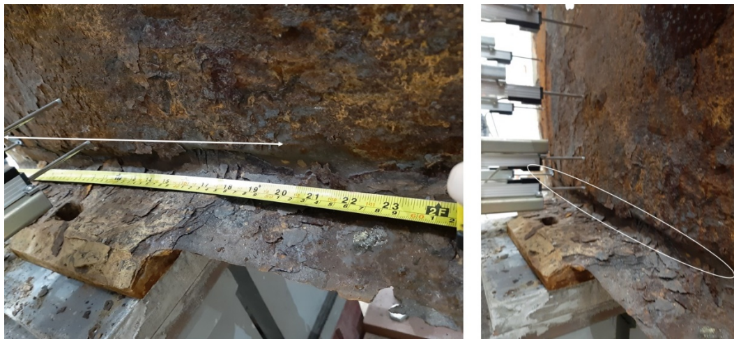
Figure 6.26: Residual deformation of studied end.
