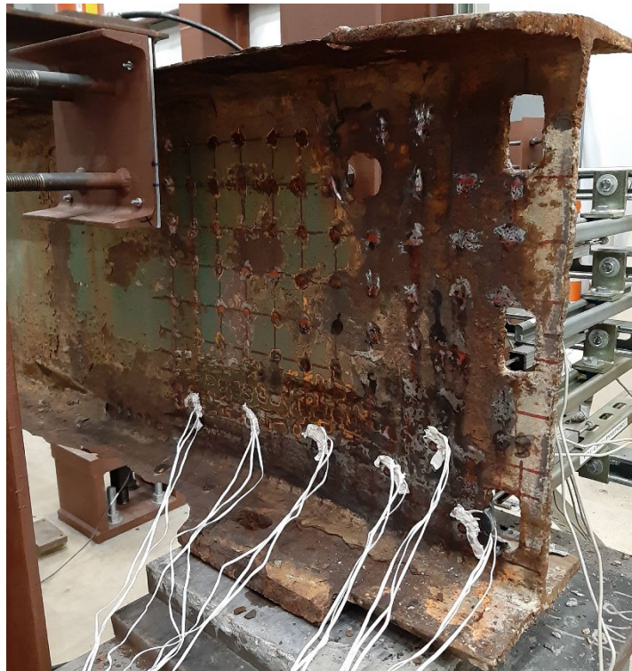
Figure 3.38: Instrumentation configuration for Specimen 4.
