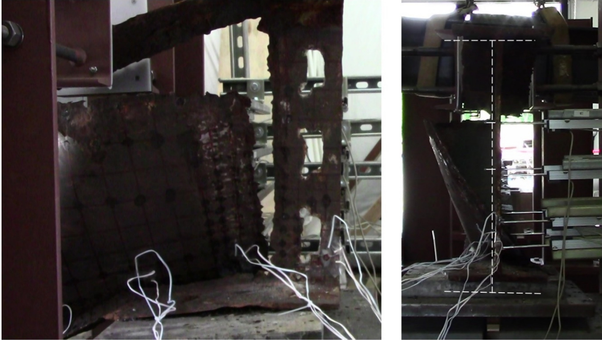
Figure 6.39: Side-by-side images showing side view of web and profile view of beam during experiment. Letters A-C correspond to Fig. 6.37a. White dashed lines illustrate cross-section location at loading initiation.
