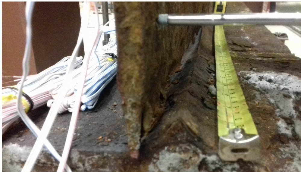
Figure 3.29: Area with 100% section loss above flange.
