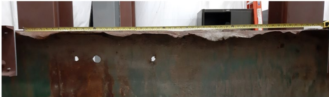
Figure 3.35: Top view of the specimen (a) and side view of the buckled web (b).
