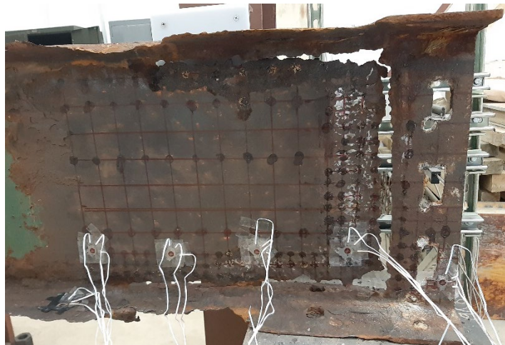
Figure 3.46: Instrumentation configuration of Specimen 6.
