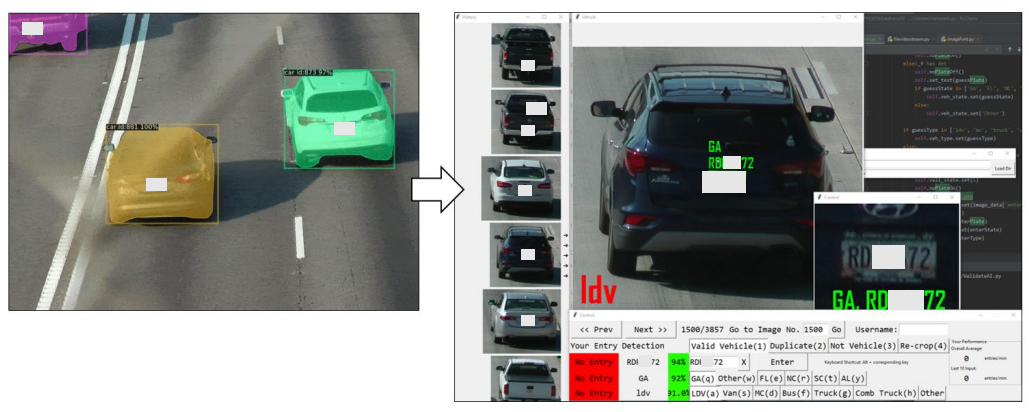
Figure 19 – Automatic System for Vehicle and License Plate Capture
