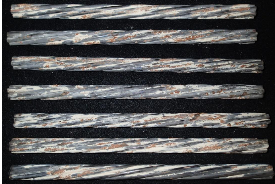
Figure 8-15. Corroded strands near port C dried TSG specimen
