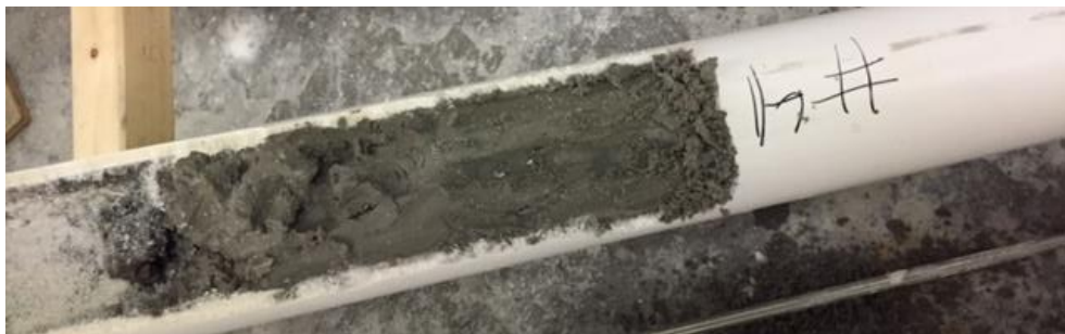
Figure 4-3. Dissection of tube for mini-inclined testing
