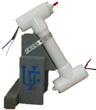
Figure 11-7. Corrosion specimen placed at 60^\circ inclination
