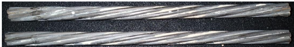
Figure 8-17. Non-corroded strands near port C control TSG specimen
