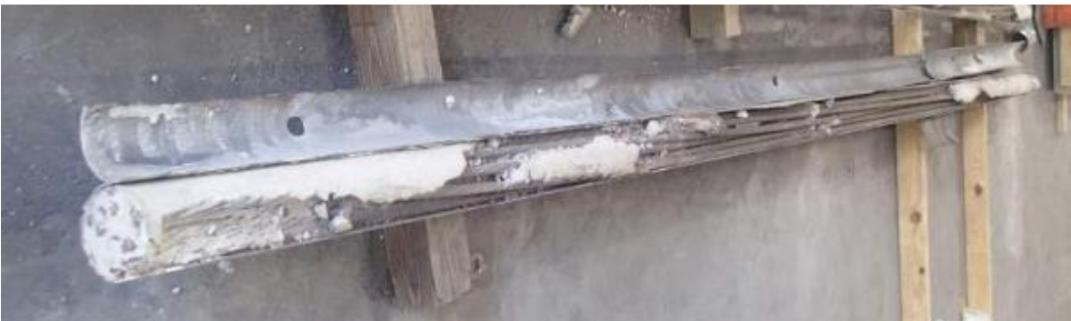
Figure A.3-17. Visual Inspection of 19S20PC-10 PC after grout removal
