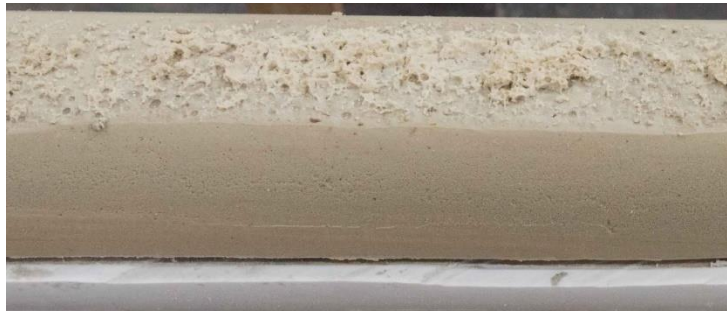
Figure 8-8. Pores on grout surface
