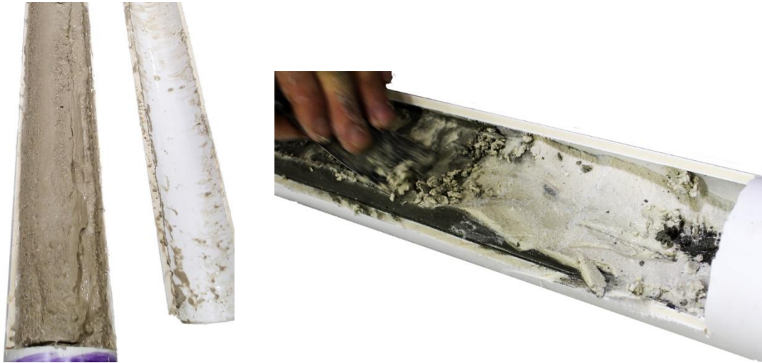
Figure A.3-9. Verification of soft grout
