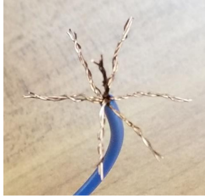
Figure 12-3. Separated stranded wire
