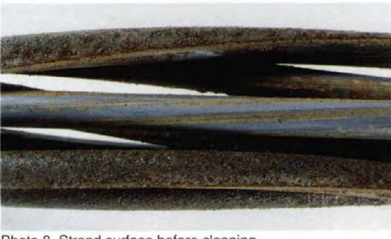
Photo 8. Strand surface before cleaning.
