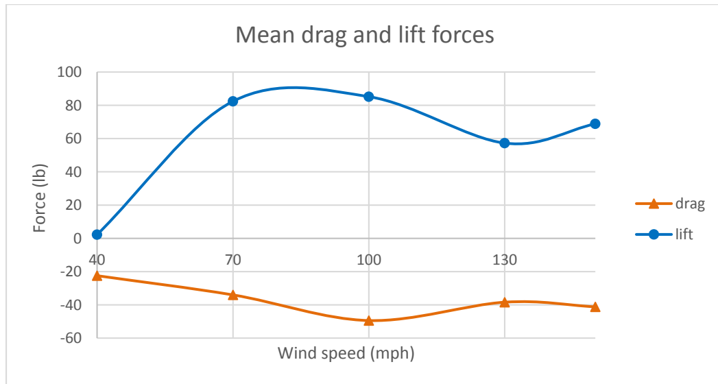
Figure H 7: Mean drag and lift forces on the traffic signals at 100 degrees wind direction
