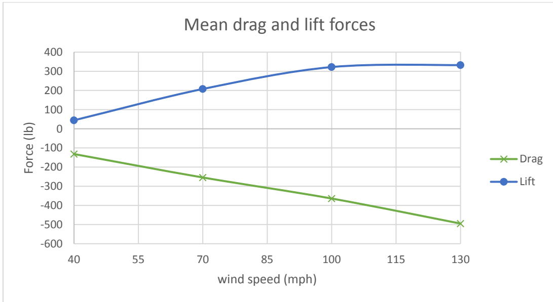
Figure J 13: Mean drag and mean lift forces on the traffic signals at 180 degrees wind direction
