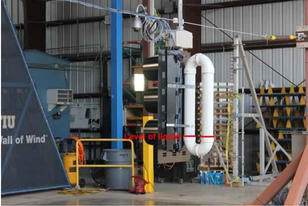
Figure 258: Close up of liquid damper with 2 L installed in rear of signal housing
