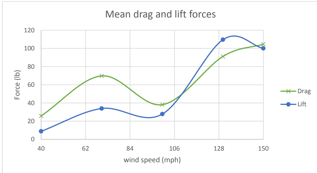
Figure B 4: Mean drag and mean lift forces at 80 degrees wind direction on the traffic signals
