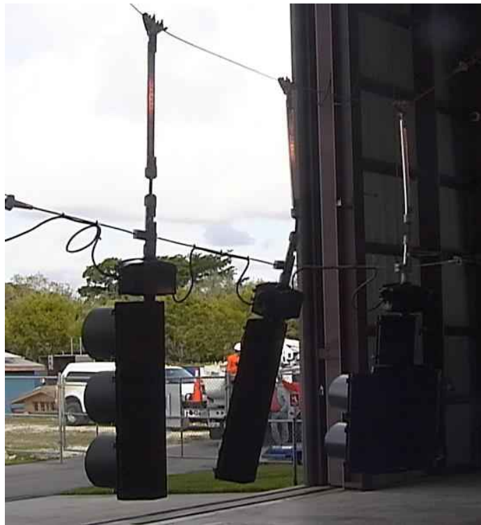
Figure 113: Traffic signals after full range of wind speed test
