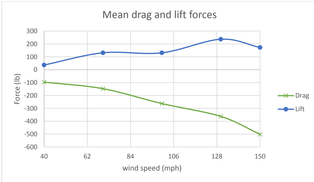
Figure B 10: Mean drag and mean lift forces at 135 degrees wind direction on the traffic signals
