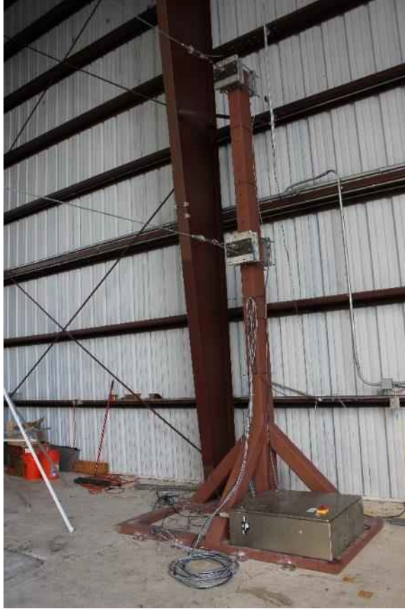
Figure 198: Column rig (full-scale, long-span)
