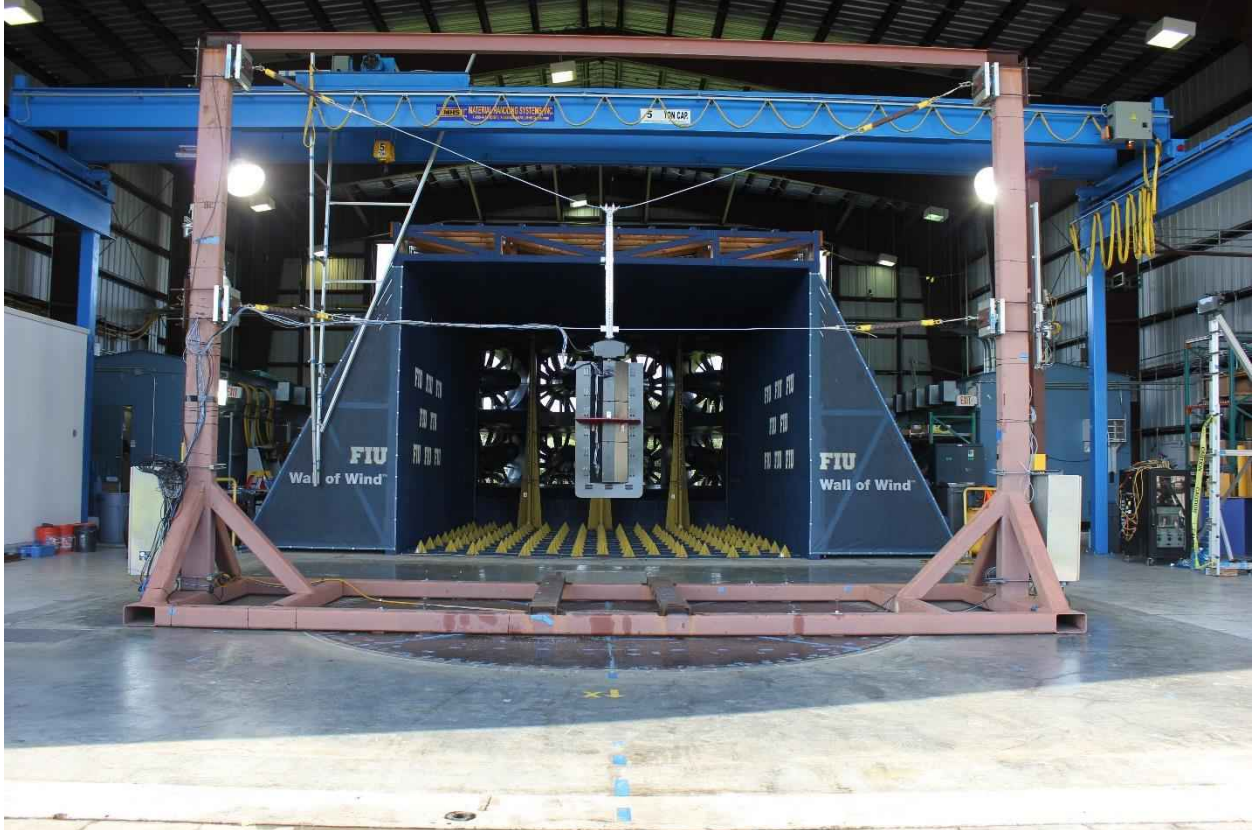
Figure 262: Signal assembly installed on test rig (before testing) with fin located at middle of signal housing
