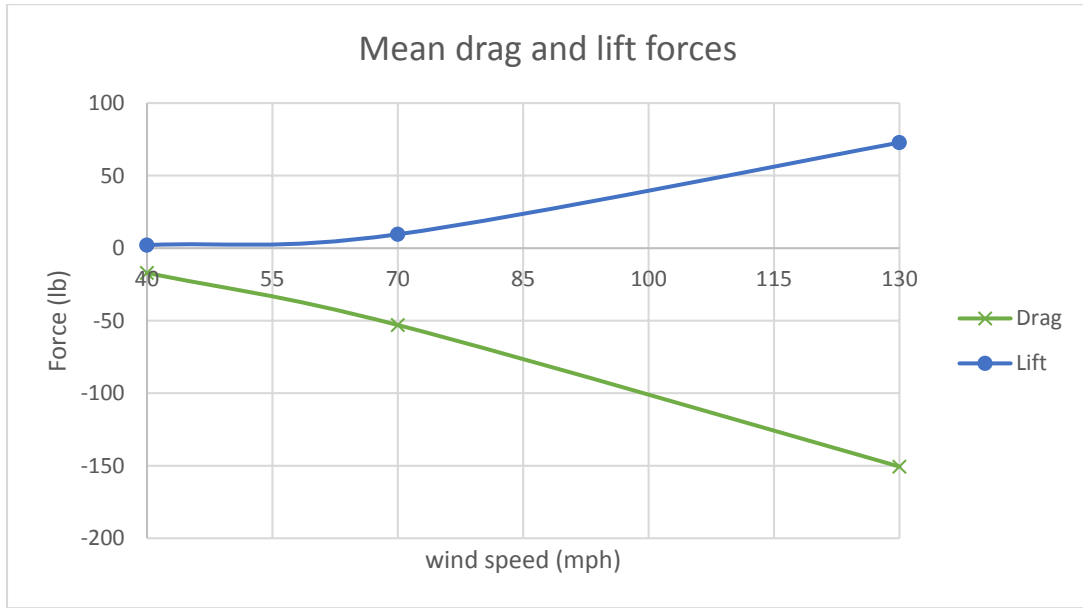
Figure J 7: Mean drag and mean lift forces on the traffic signals at 100 degrees wind direction
