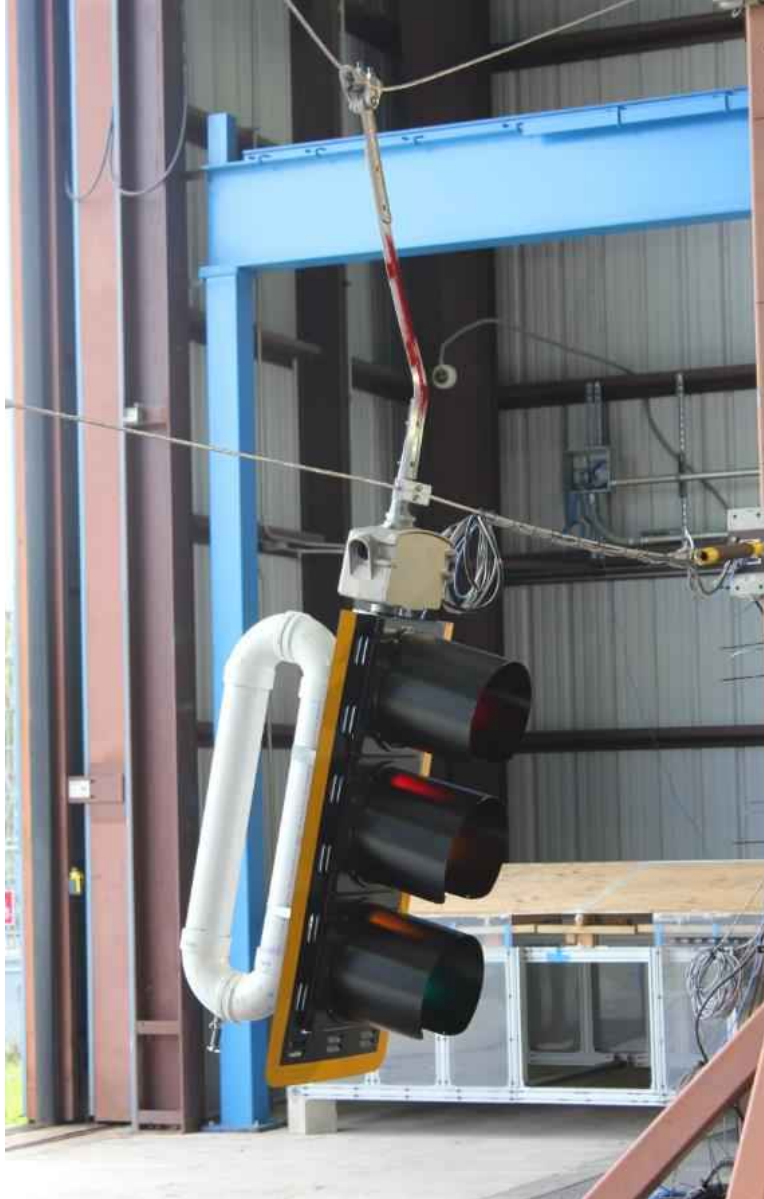
Figure 281: "Liquid-damper-with-OL case" after 150 mph at 0 degrees
