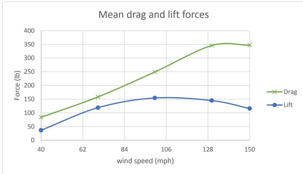
Figure G 1: Mean drag and lift forces on the traffic signals at 45 degrees wind direction
