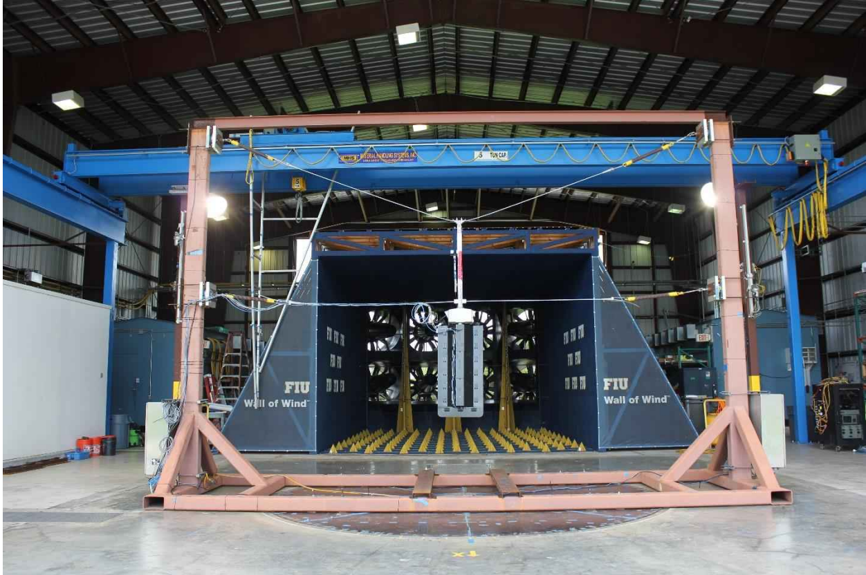
Figure 256: Signal assembly installed on test rig (before testing) with no mitigation device
