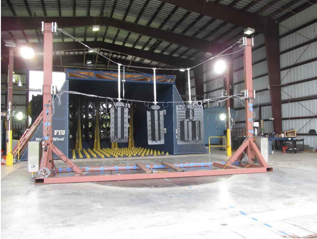
Figure 182: Picture of test rig frame with the signals and the “tri-stud adjustable hanger” (also known as base configuration)
