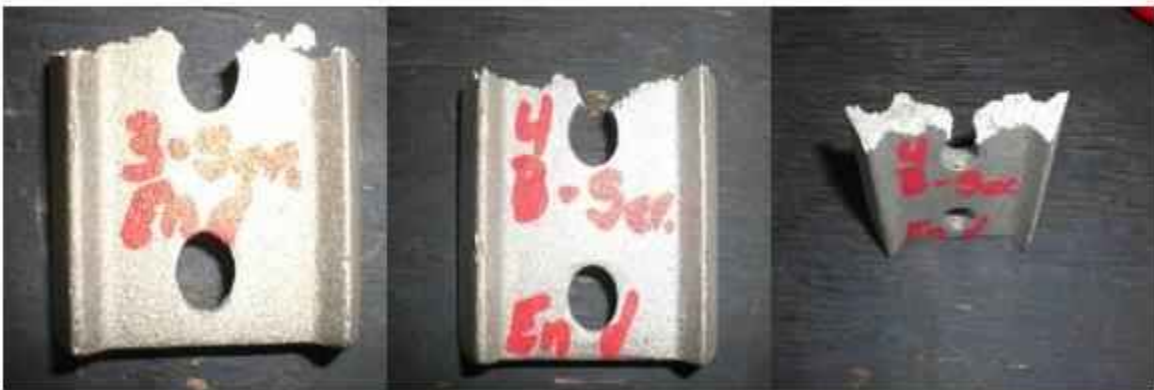
Figure 52: Tri-stud adjustable hanger after Test 2 showing location of damage. No noticeable damage to the aluminum messenger clamp. Sections of the bottom bracket that were sheared off
