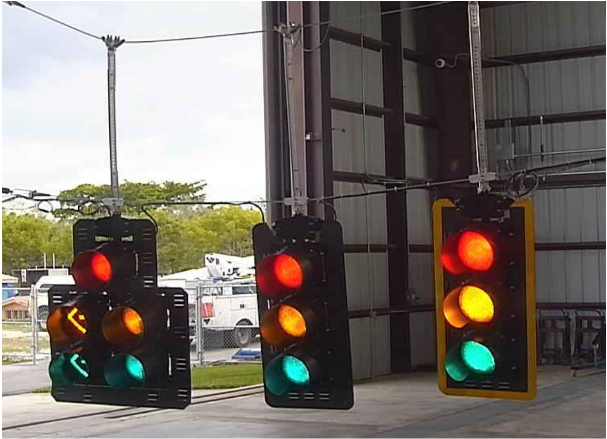
Figure 116: Picture showing a portion of the test rig frame with the tri-stud adjustable hanger system
