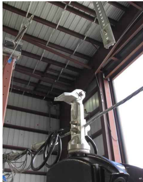
Figure 68: Pivotal adjustable hanger sheared off above pivotal portion
