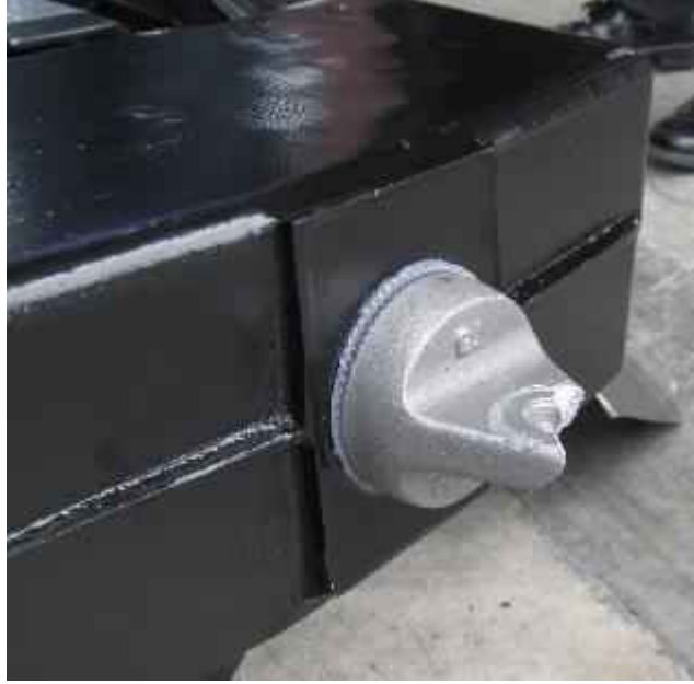
Figure 96: Cracked hook on top of 5-section signal disconnect box
