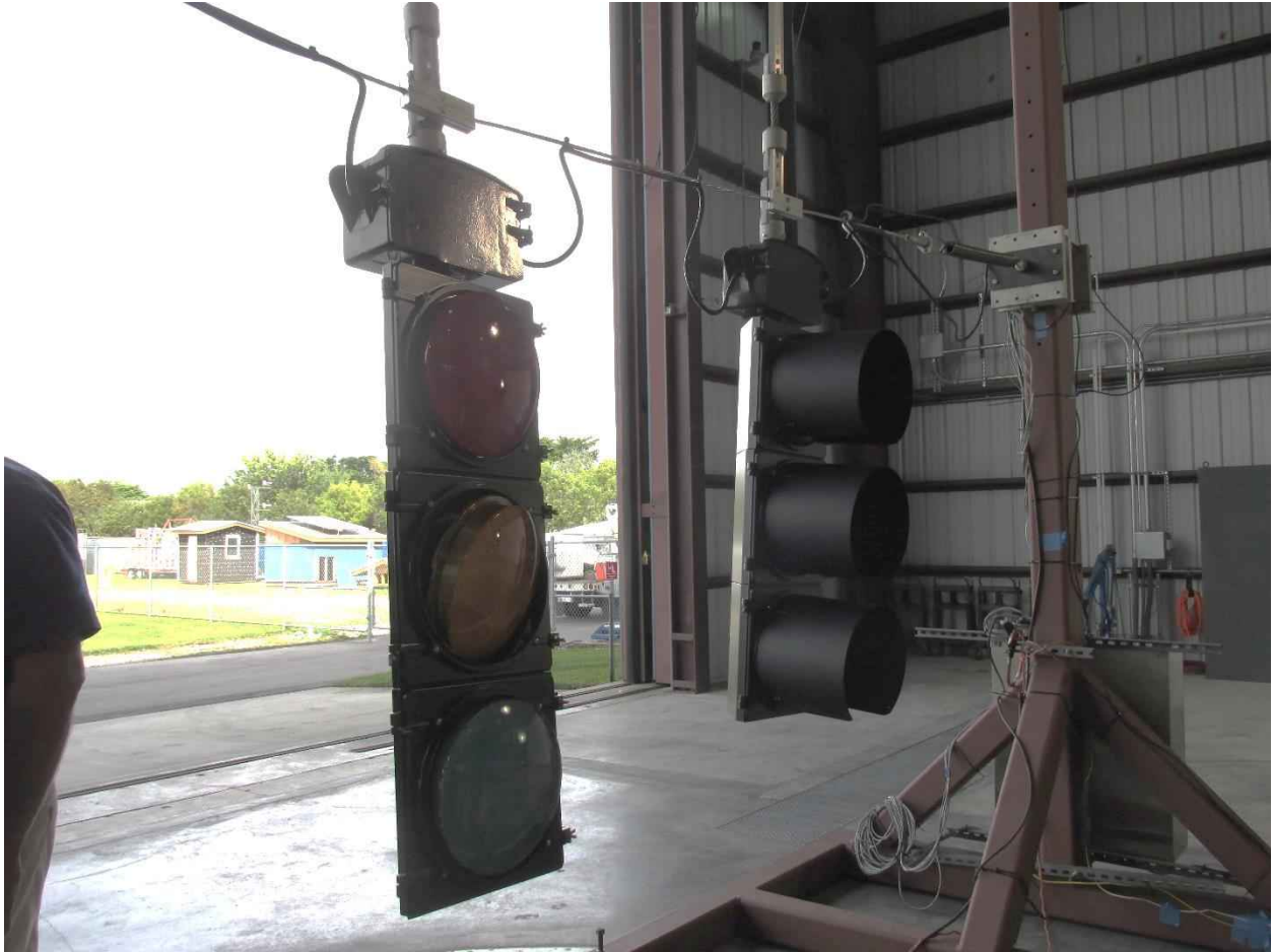
Figure 100: Picture showing a portion of the test rig frame with the 3-section traffic signals
