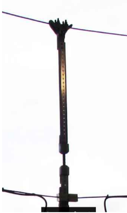
Figure 112: Pelco adjustable hanger assembly with cable dampener after full range test
