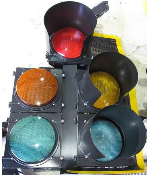
Figure 196: 5-section signal after full test
