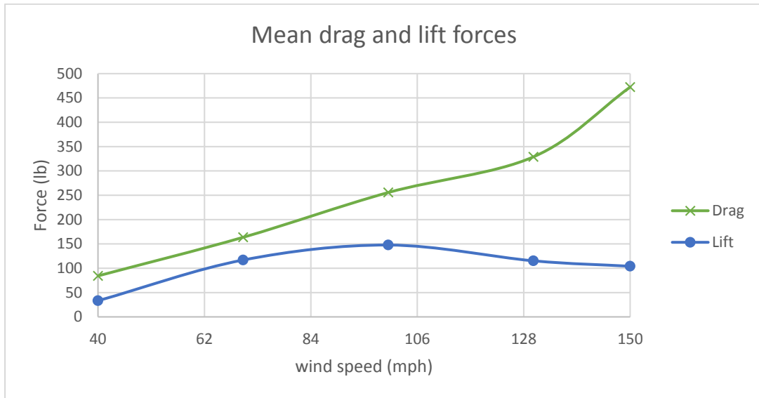
Figure B 1 Mean drag and mean lift forces at 45 degrees wind direction on the traffic signals
