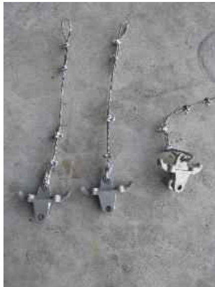
Figure 99: Steel cable hangers after full wind test
