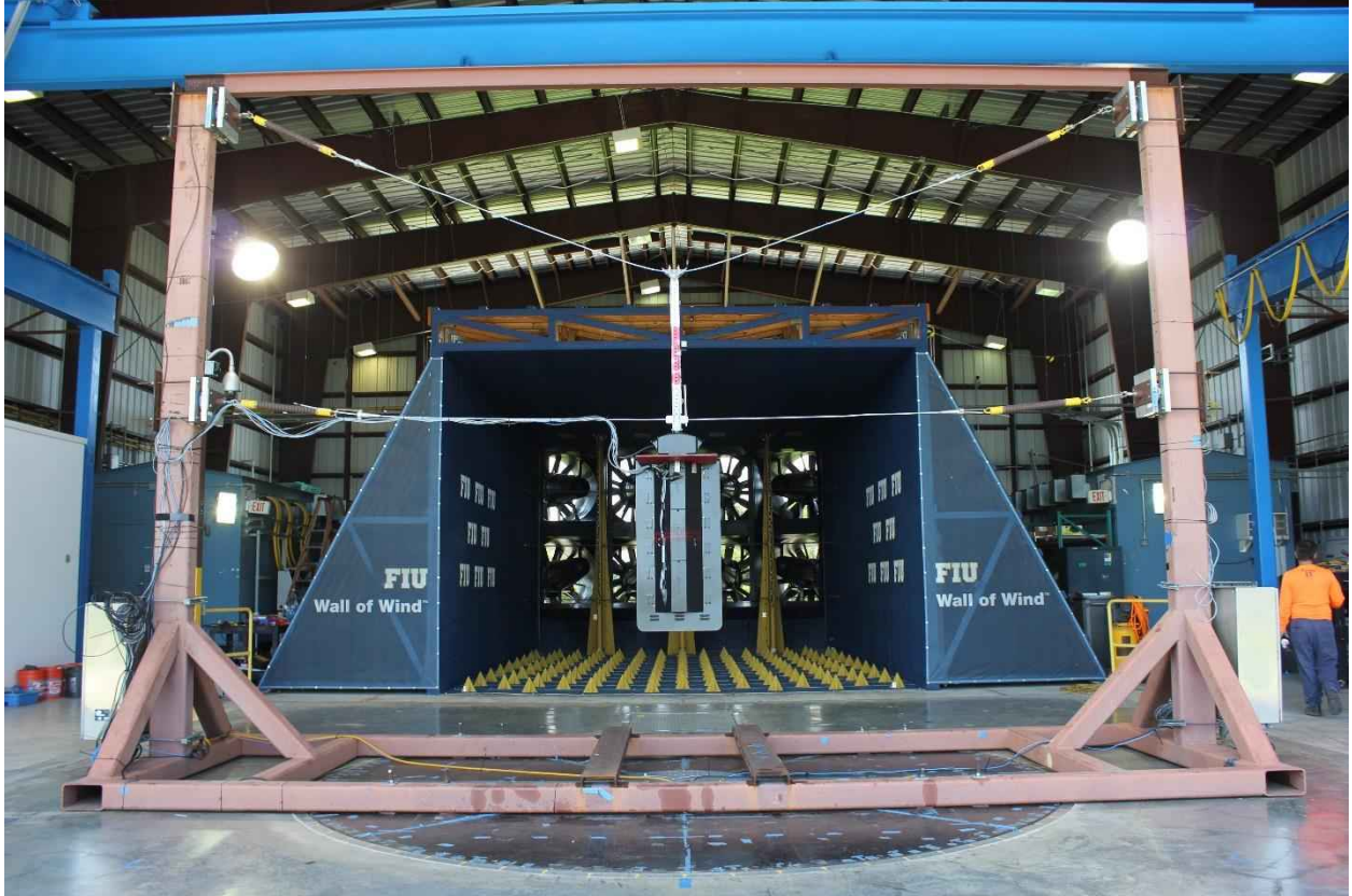
Figure 260: Signal assembly installed on test rig (before testing) with fin located at top of signal housing
