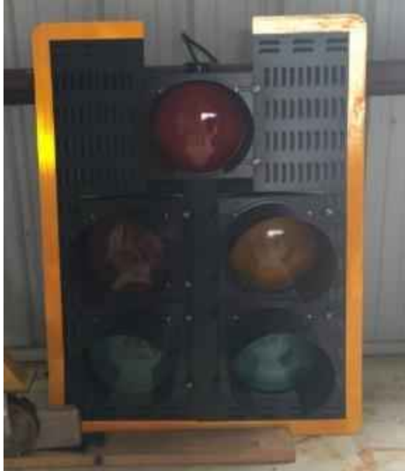
Figure 32: 5-section signal with visors after Test 1 showing no noticeable damage
