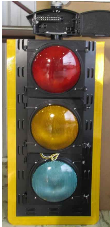
Figure 195: 3-section signal after full test
