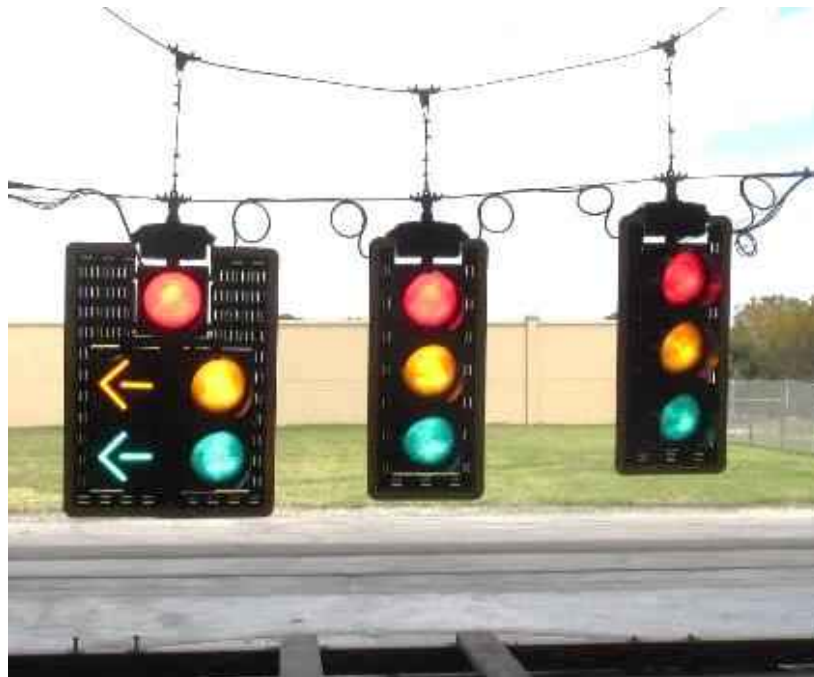
Figure 85: Traffic signal set up: a) 3-section signal showing the steel cable hanger assembly with reinforced disconnect hanger (vendor: Engineered Castings); b) traffic signal assembly facing the wind
