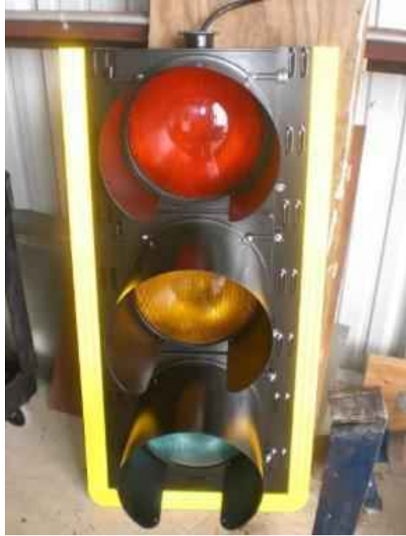
Figure 31: 3-section signal with visors after Test 1 showing no noticeable damage
