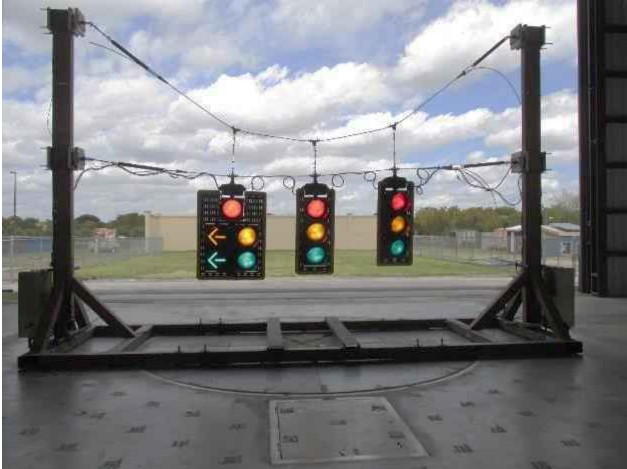
Figure 84: Picture of test rig frame with the signals and the steel cable hanger assembly
