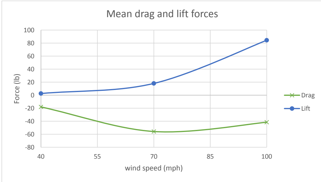
Figure F 7: Mean drag and lift forces on the traffic signals at 100 degrees wind direction
