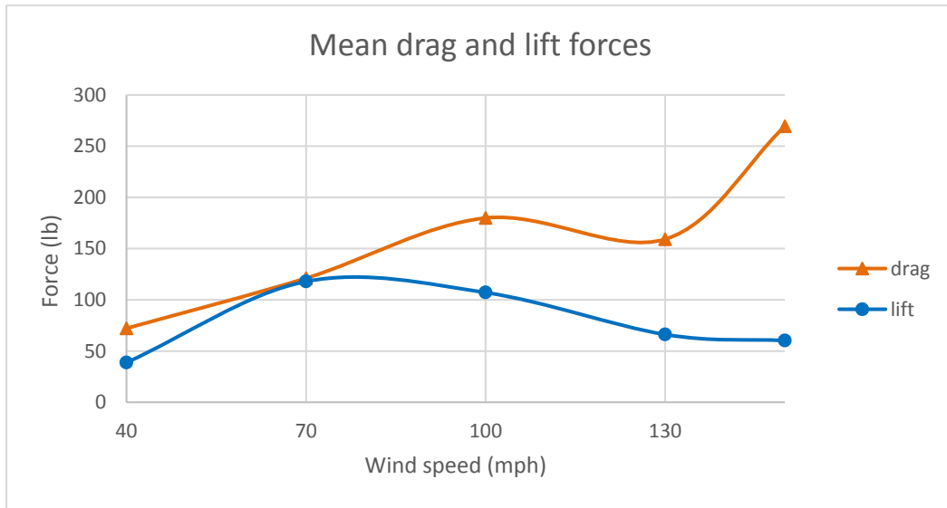
Figure H 1: Mean drag and lift forces on the traffic signals at 45 degrees wind direction
