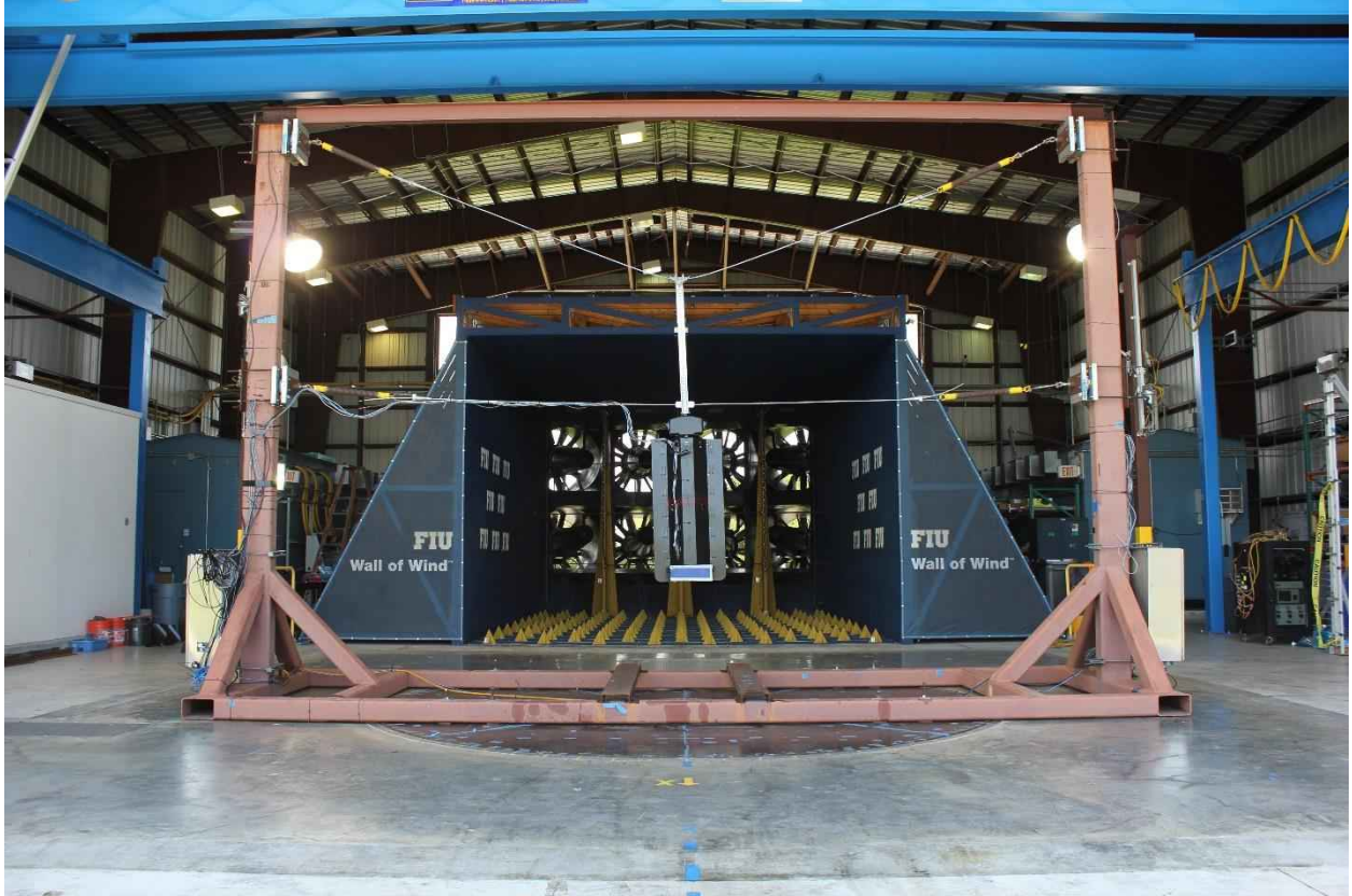
Figure 264: Signal assembly installed on test rig (before testing) with metal-box and iron-ball
