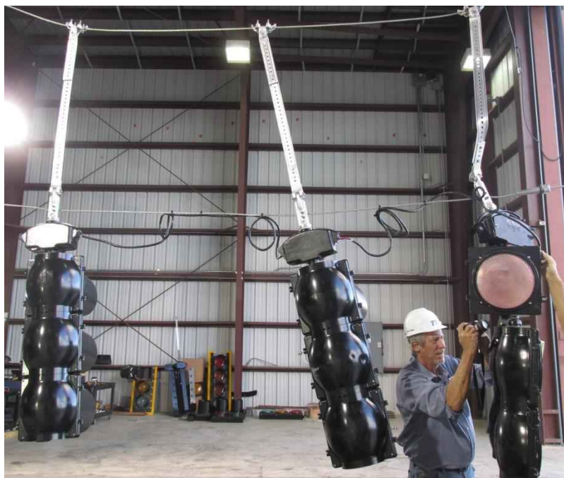
Figure 82: Signal assembly after full wind speed test
