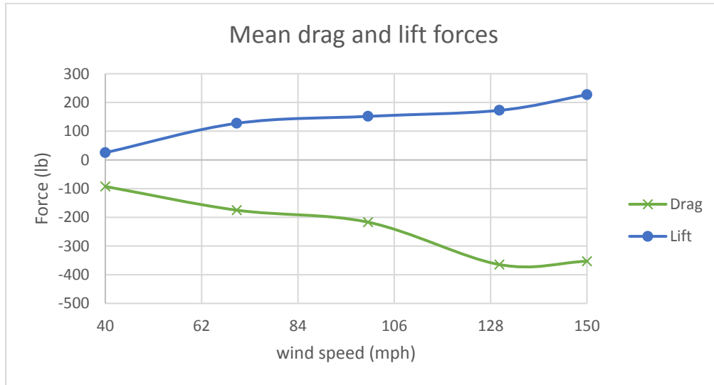
Figure E 10: Mean drag and lift forces on the traffic signals at 135 degrees wind direction
