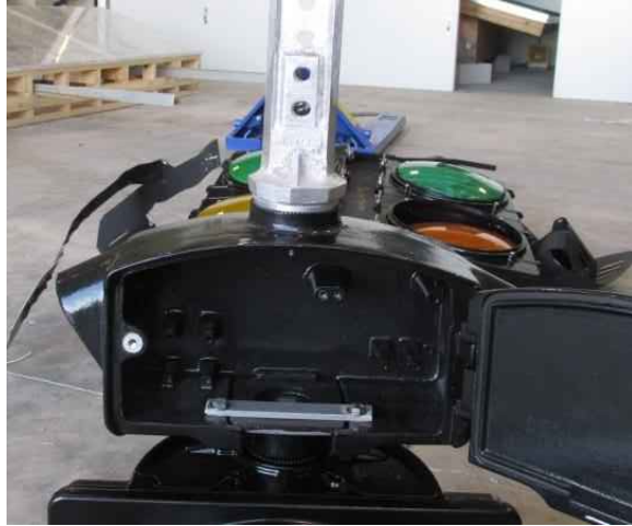
Figure 130: Disconnect box for 5-section signal with no visible damage (all wiring removed)
