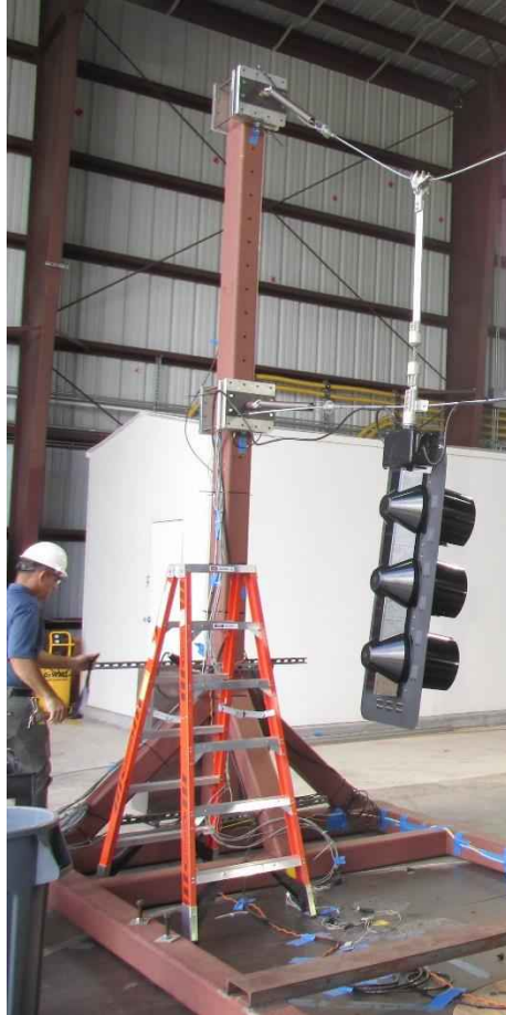
Figure 132: Picture of a part of the test rig frame with the 3-section signal and the adjustable hanger assembly
