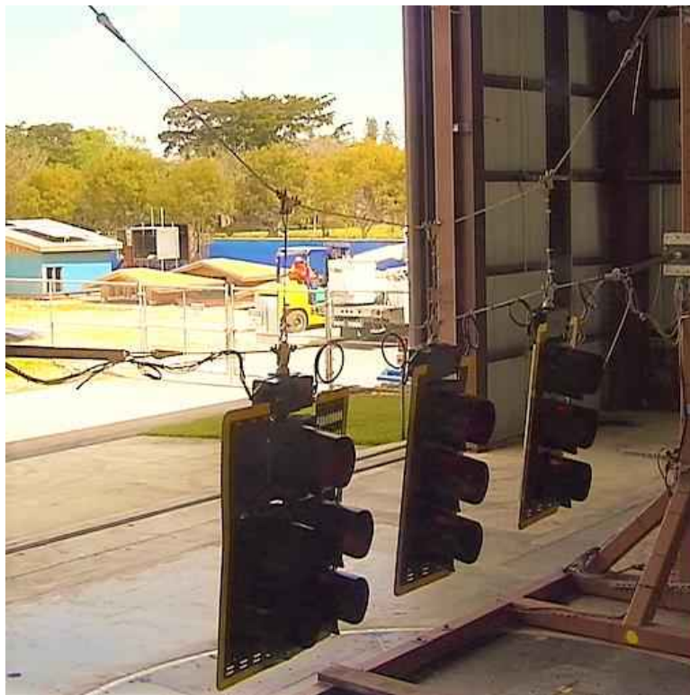
Figure 149: Traffic signal set up: a) 3-section signal showing the steel cable hanger assembly with reinforced disconnect hanger (vendor: Engineered Castings); b) traffic signal assembly facing the wind
