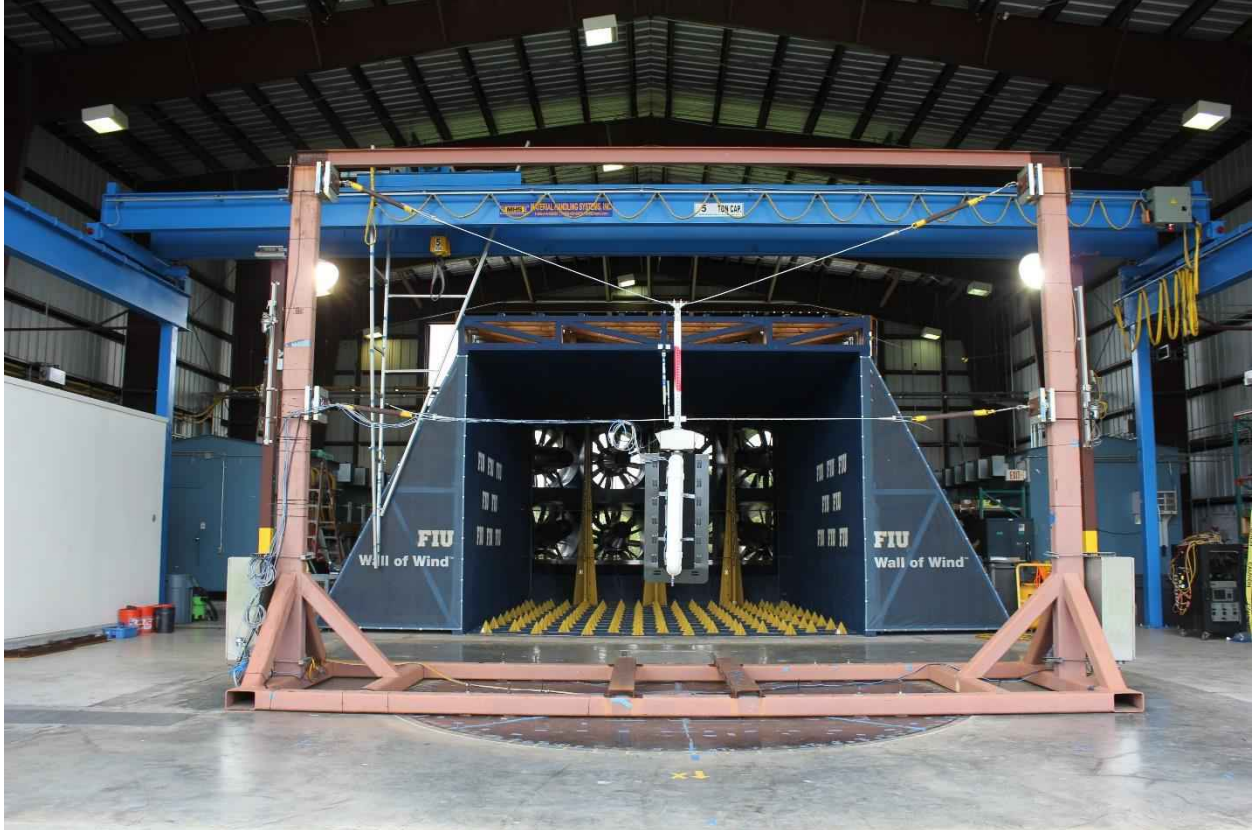
Figure 259: Signal assembly installed on test rig (before testing) with liquid damper (with zero liters of water)
