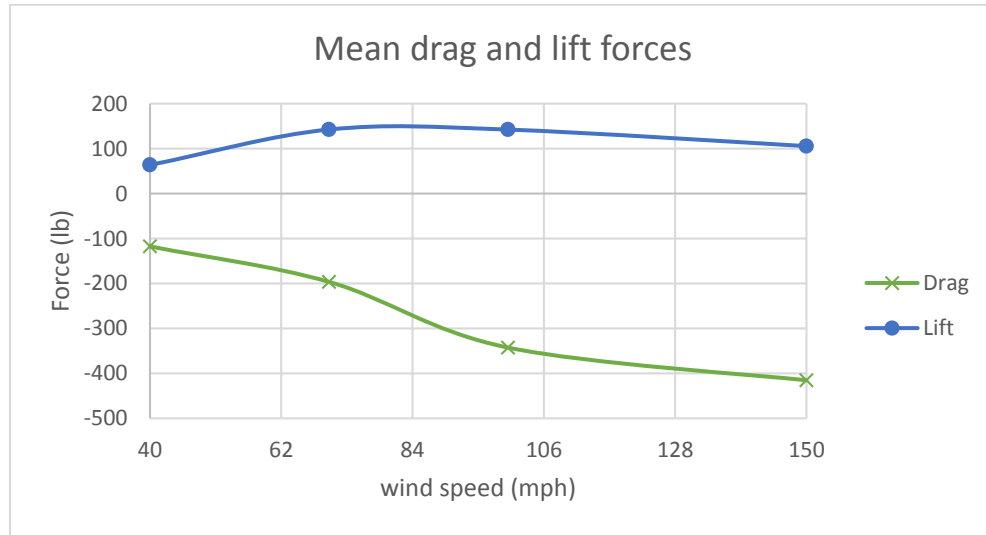
Figure B 13: Mean drag and mean lift forces at 180 degrees wind direction on the traffic signals
