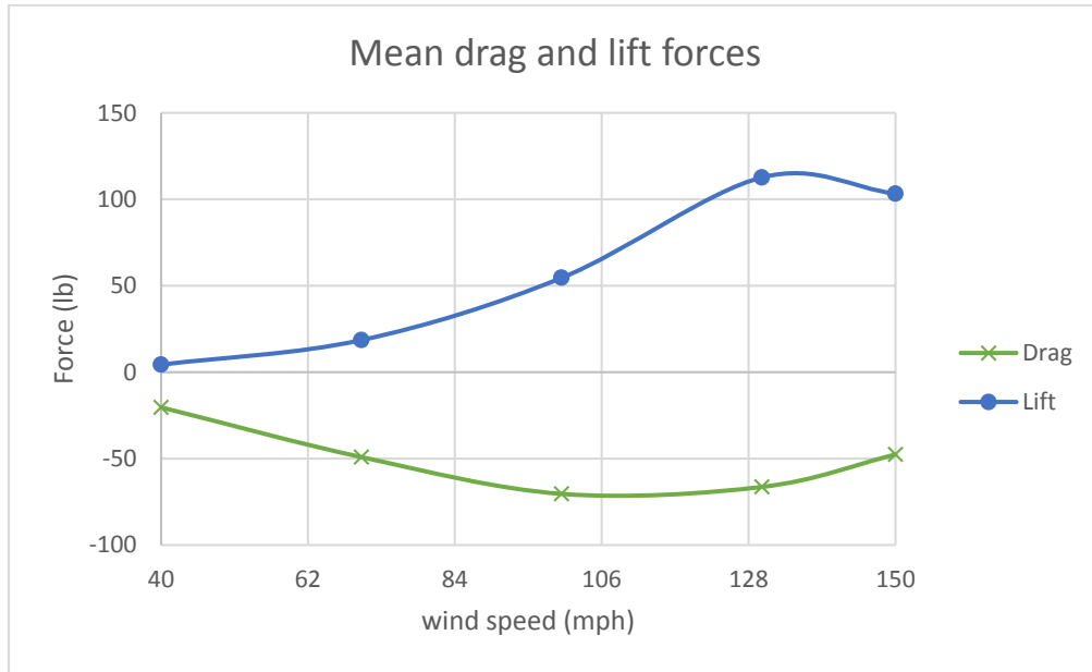
Figure G 7: Mean drag and lift forces on the traffic signals at 100 degrees wind direction
