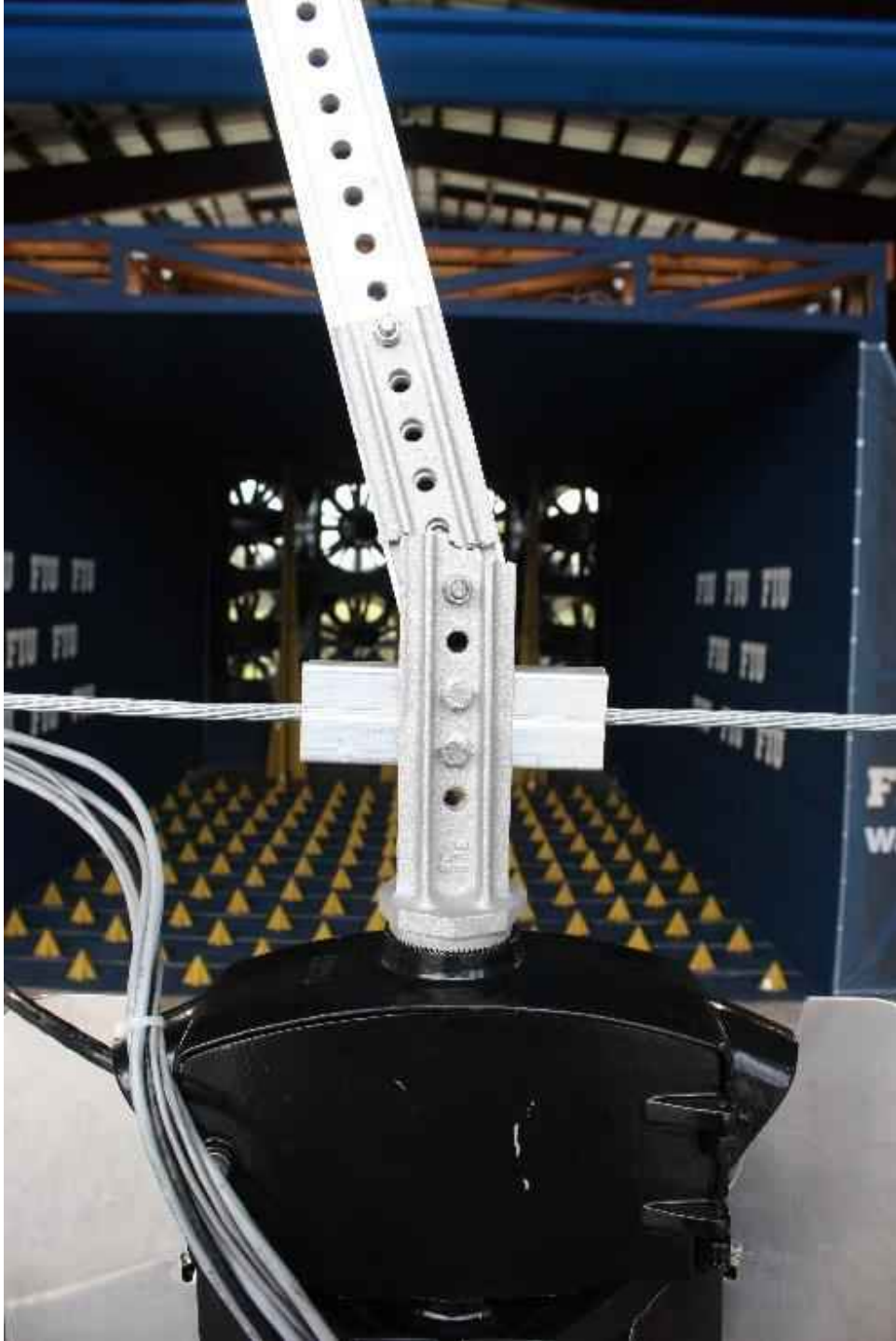
Figure 181: Sheared Hanger Connection
