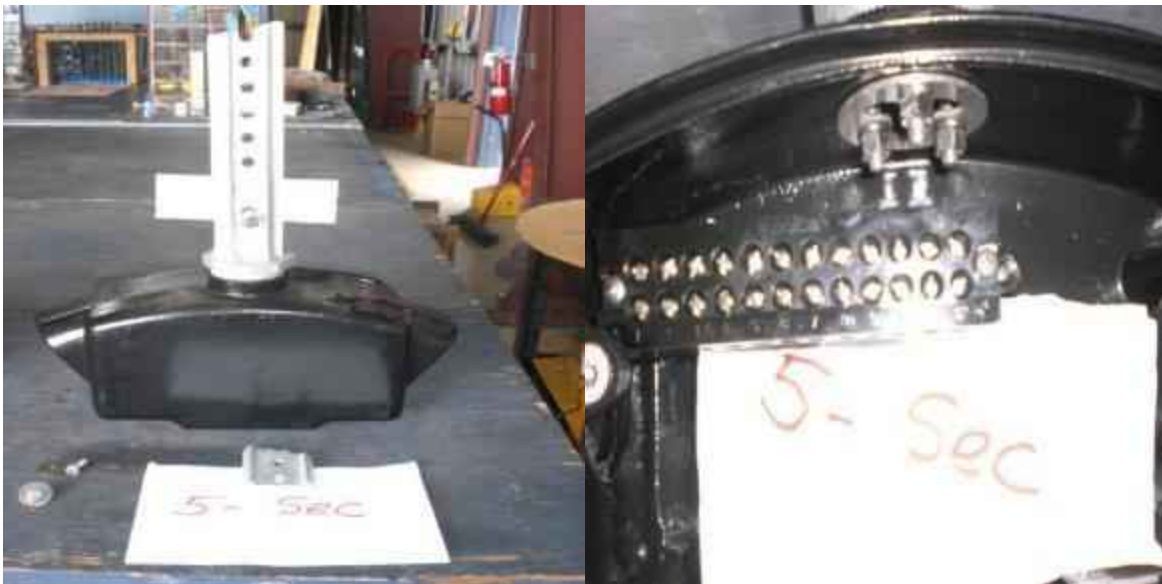
Figure 29: Disconnect box for 5-section signal after Test 1 showing no noticeable damage
