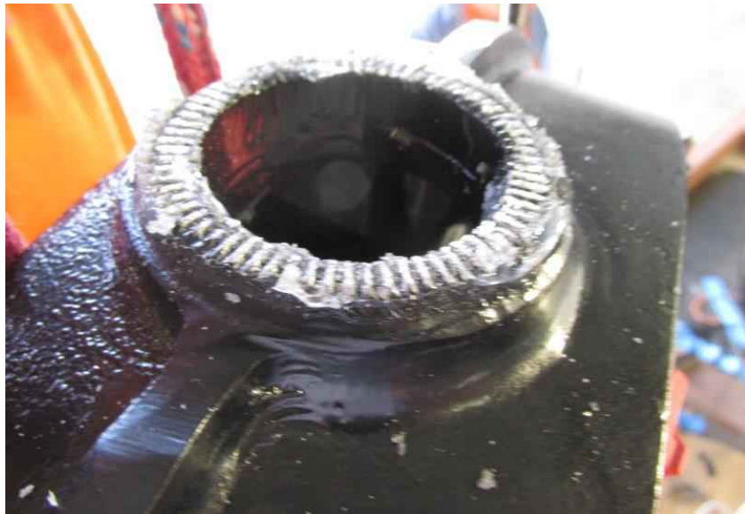
Figure 66: Disconnect box with worn way serrated box with worn away serrated teeth
