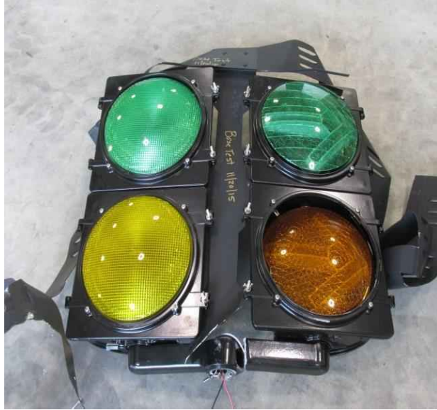
Figure 128: Lower portion of 5-section signal that severed
