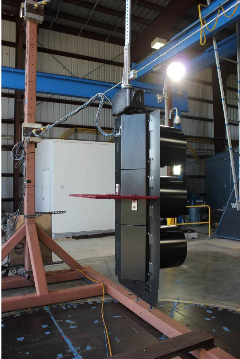
Figure 263: Close up of fin located at middle of signal housing
