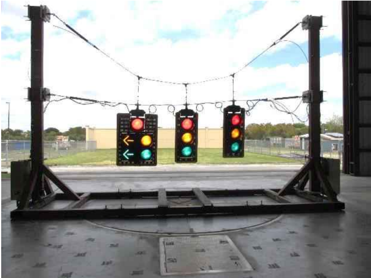
Figure 148: Picture of test rig frame with the signals and the steel cable hanger assembly
