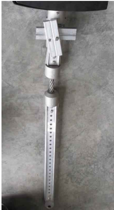
Figure 133: Traffic signal set up: a) portion of the messenger wire with the 3-section signal; b) enlarged picture of the adjustable hanger assembly connection
