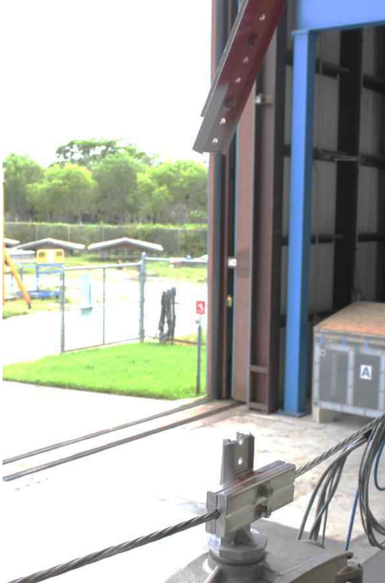
Figure 279: "No-mitigation case" failure of adjustable-hanger at 150 mph at 0 degrees
